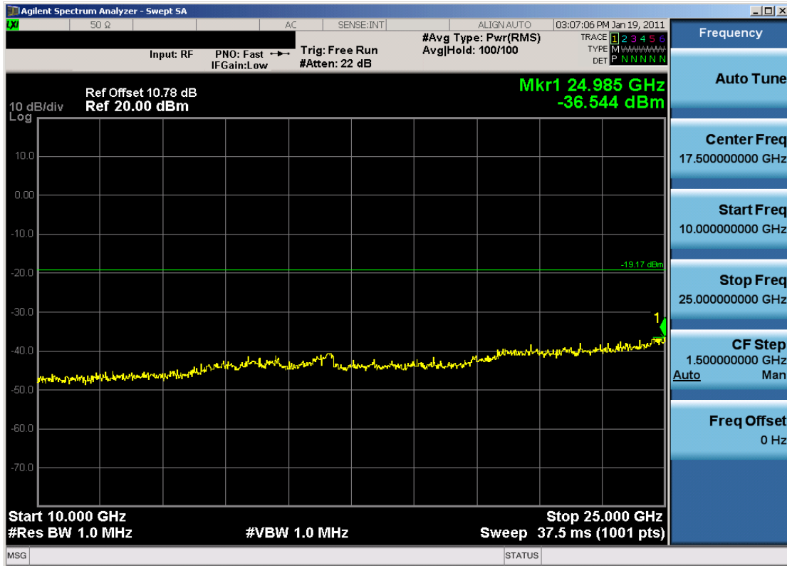
Plot 6-26. Conducted Spurious Plot (802.11b – Ch. 1)
