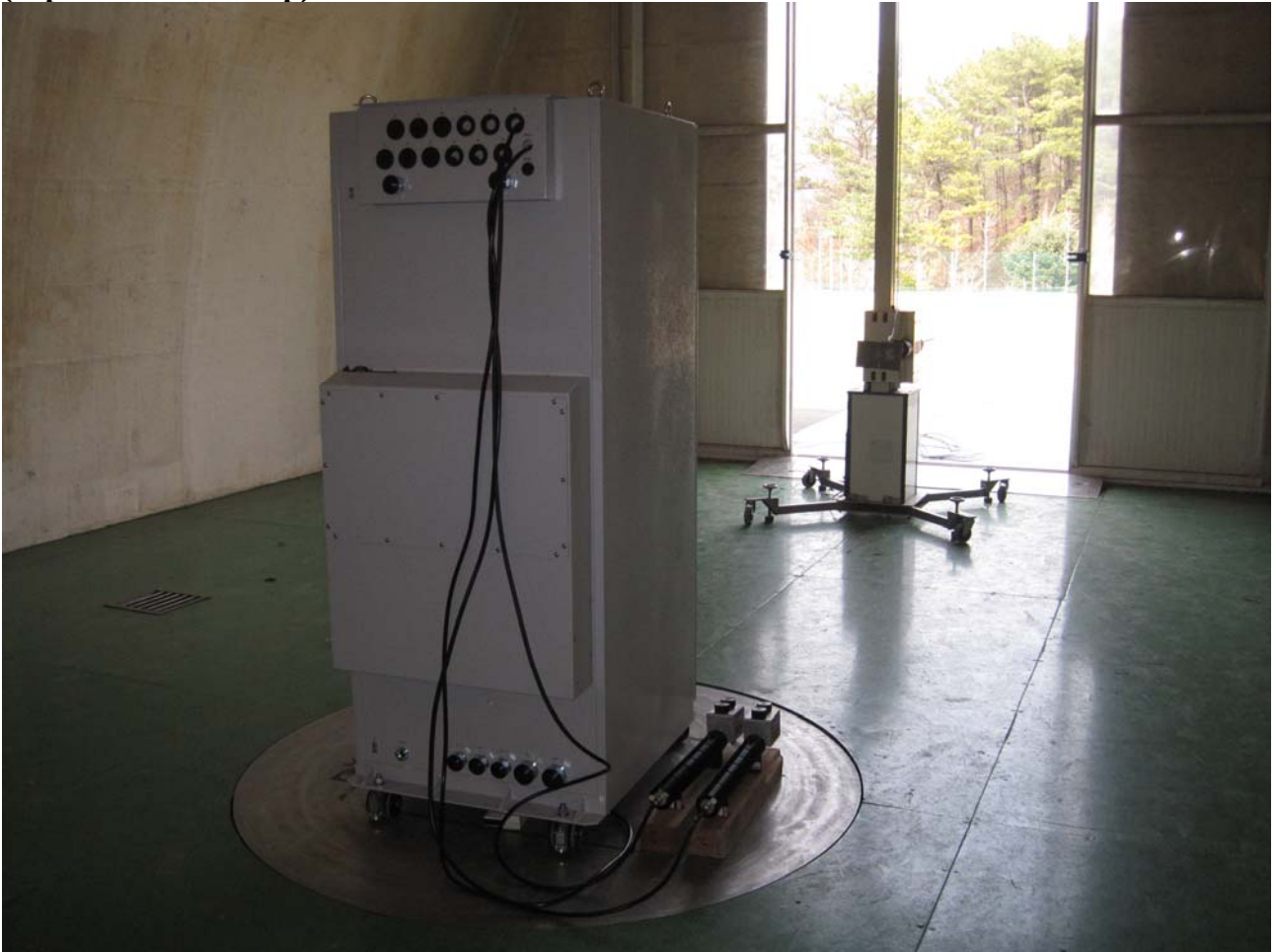
( Open Site Test Setup)
