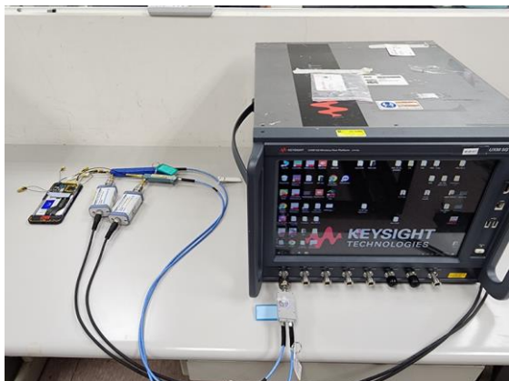
Photograph 5. Test Case 16, Band handover
