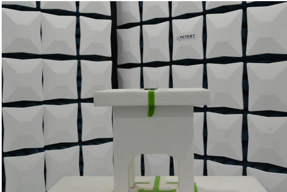
Figure 1. Test Setup – X Position – 1GHz-18GHz
