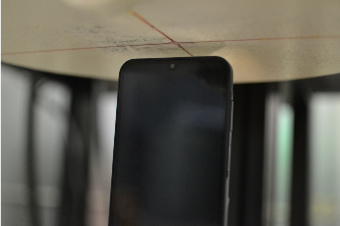
SAR Test Setup Photo 10 – Hotspot, Top Edge at 10mm
