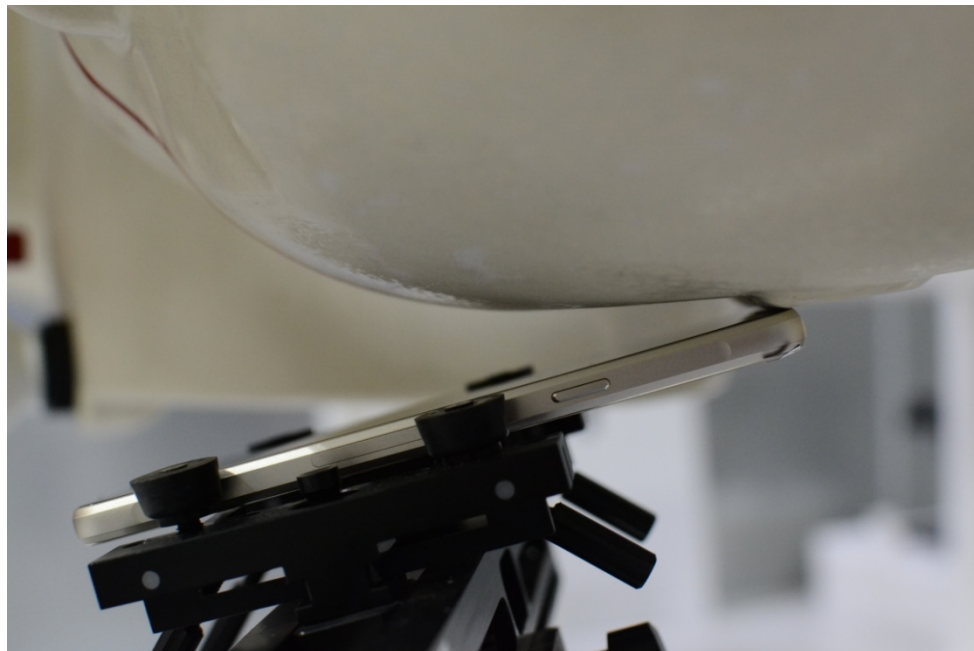
SAR Test Setup Photo 4- Left Tilt
