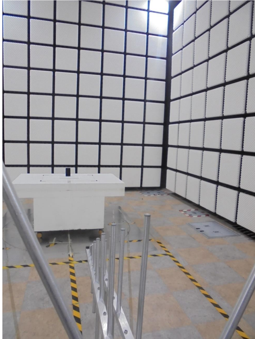
NFC Radiated Test Setup Photo for 30 MHz ~ 1 GHz
