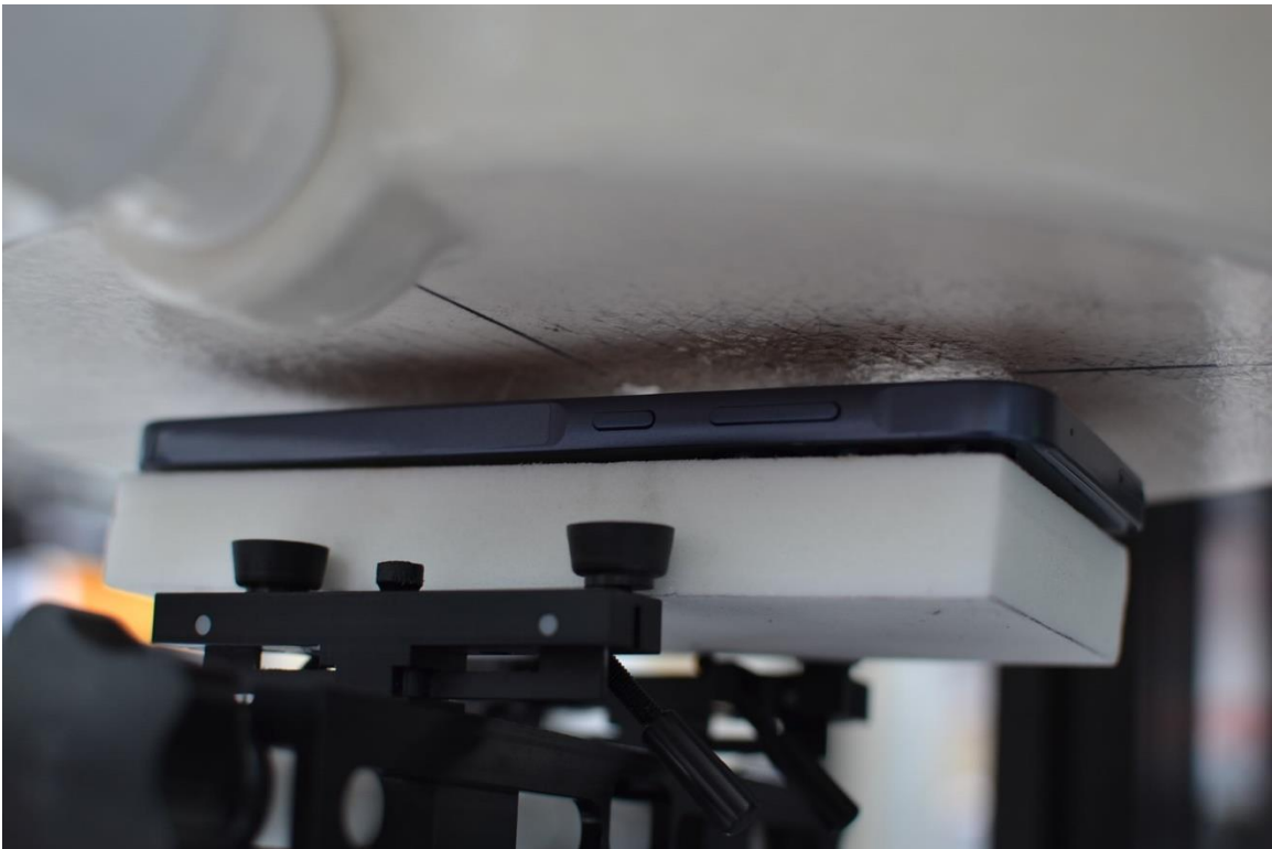
SAR Test Setup Photo 8 – Hotspot, Front Side at 10mm
