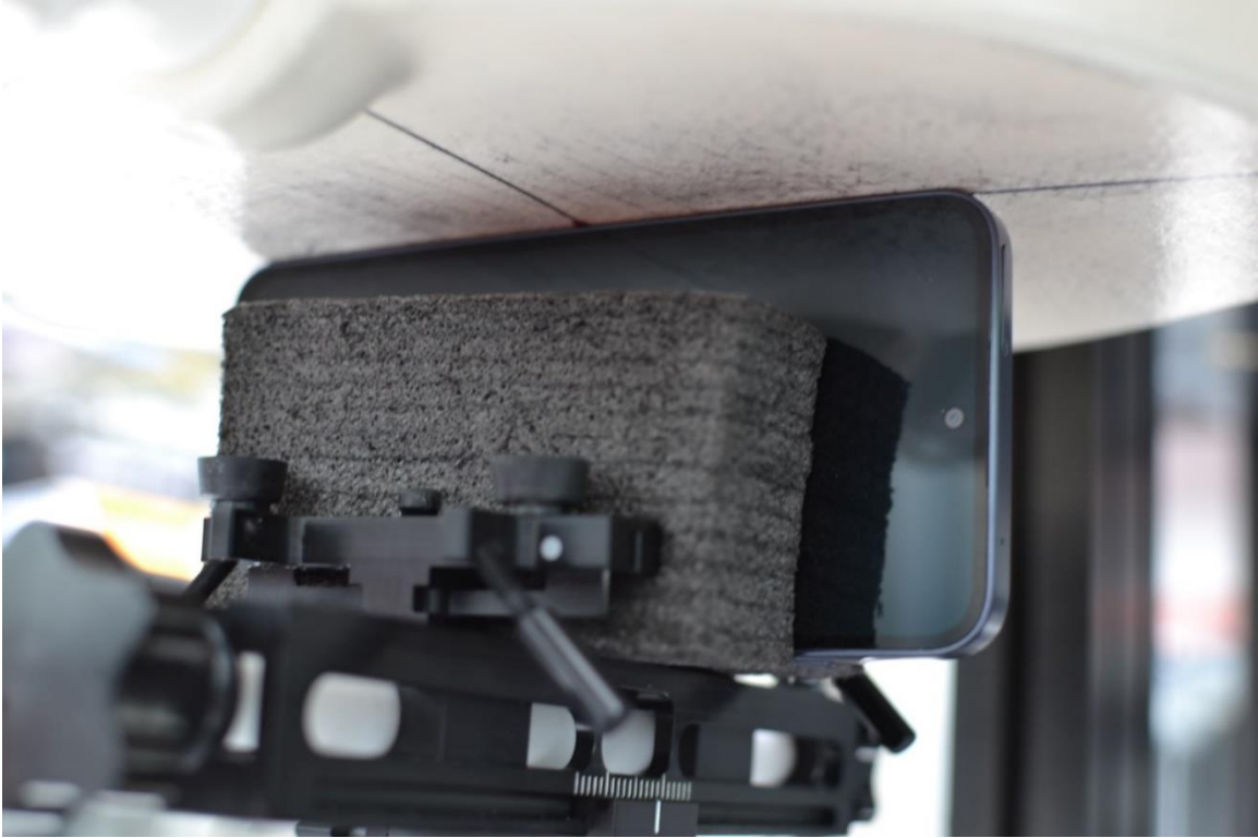
SAR Test Setup Photo 17 – Phablet, Left Edge at 0mm
