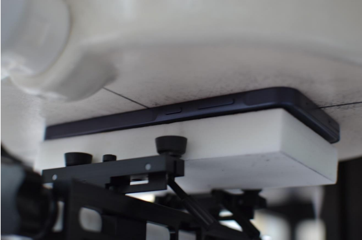
SAR Test Setup Photo 9 – Phablet, Front Side at 0mm
