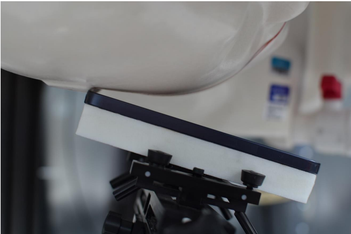
SAR Test Setup Photo 2 – Head, Right Tilt at 0mm
