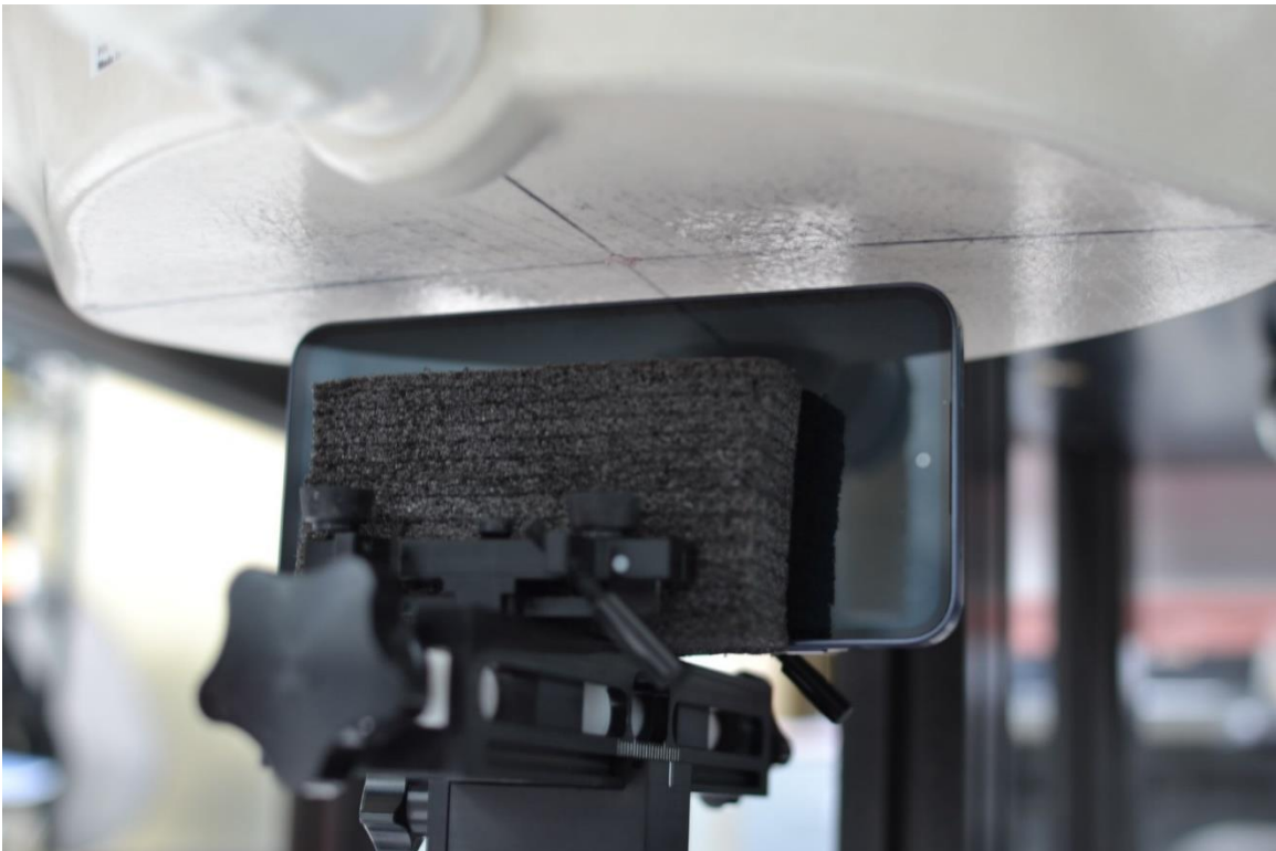
SAR Test Setup Photo 16 – Hotspot, Left Edge at 10mm
