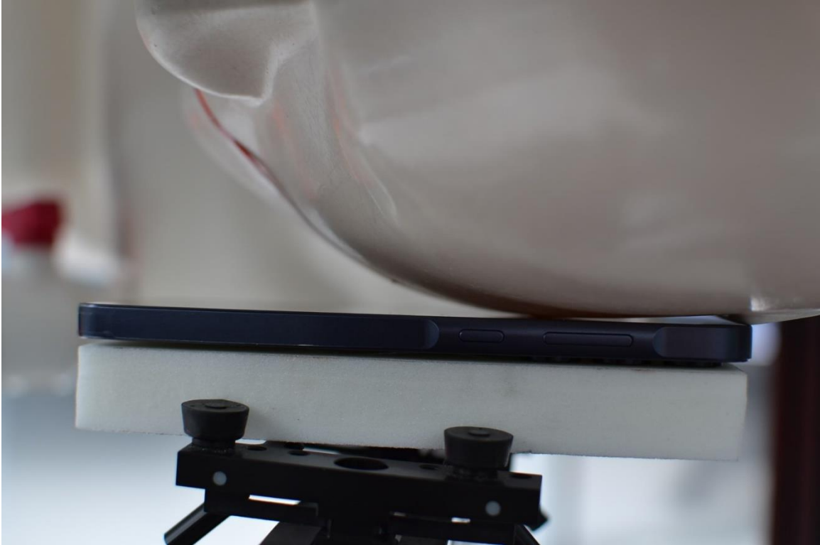
SAR Test Setup Photo 3 – Head, Left Cheek at 0mm
