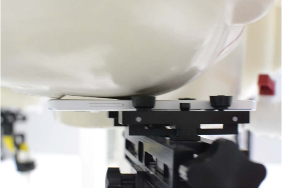
SAR Test Setup Photo 1 – Right Cheek
