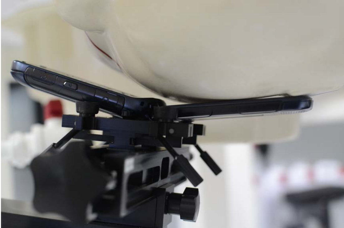
SAR Test Setup Photo 3 – Left Cheek
