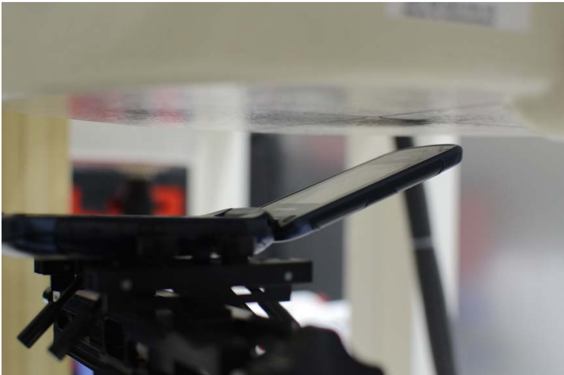
SAR Test Setup Photo 4 –Left Cheek (Mouth Jaw Configuration)
