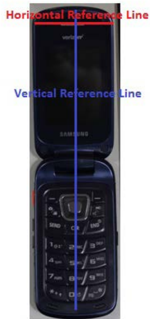
SAR Test Setup Photo 7 – DUT Reference Lines
