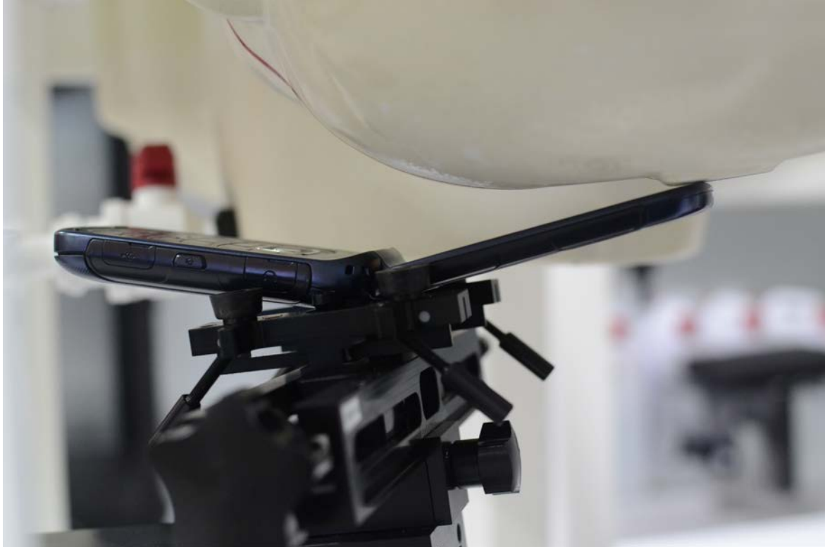
SAR Test Setup Photo 5 – Left Tilt
