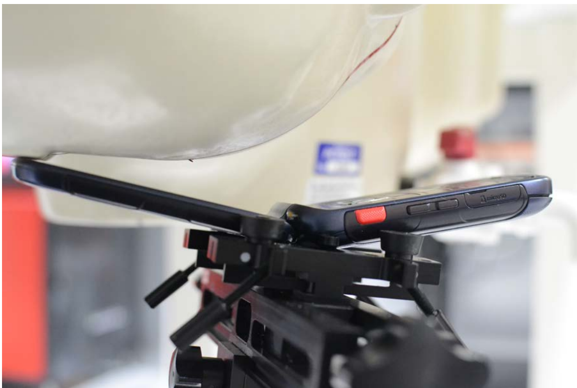
SAR Test Setup Photo 2 – Right Tilt
