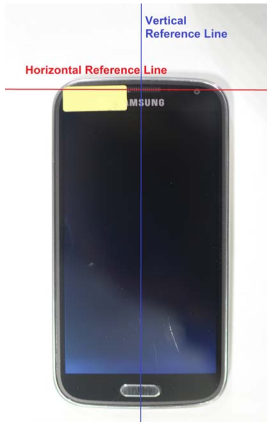
SAR Test Setup Photo 10: Vertical and Horizontal Reference Lines
