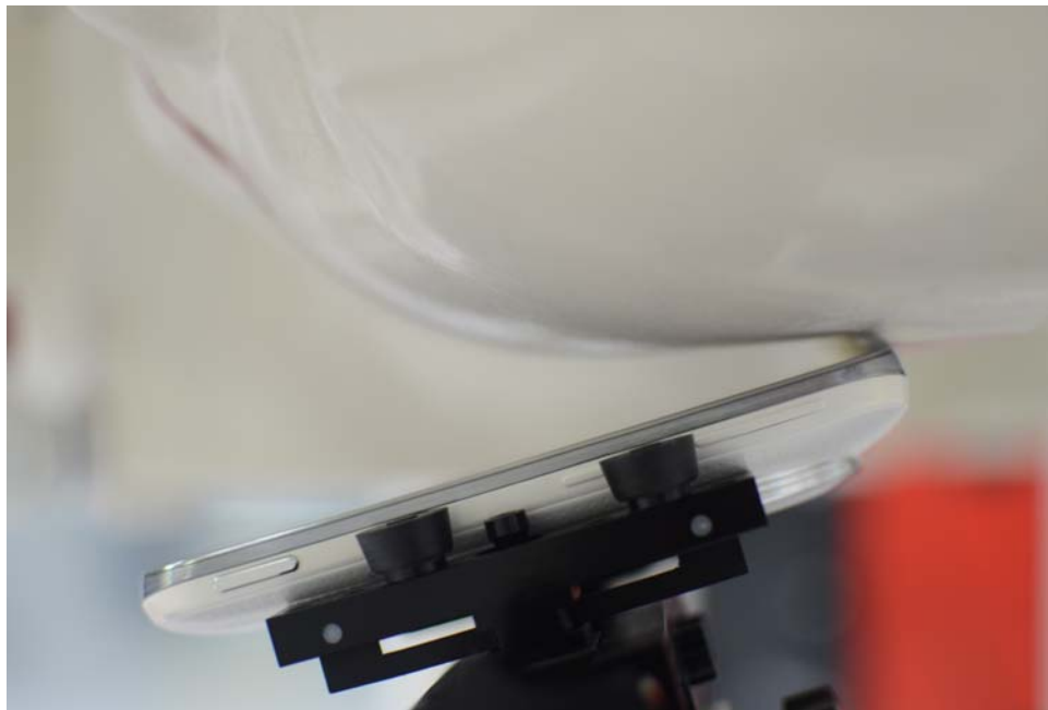
SAR Test Setup Photo 4: Left Tilt
