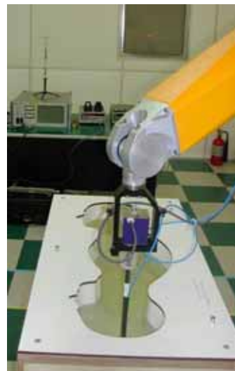
Figure 3. Photograph of the probe and the Phantom
