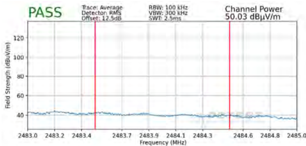
Plot 7-107. Radiated Restricted Upper Band Edge Measurement SISO ANT1 (Average)
