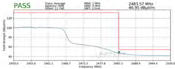
Plot 7-125. Radiated Restricted Lower Band Edge Measurement MIMO (Average)
