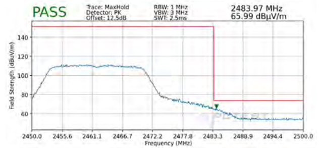
Plot 7-128. Radiated Restricted Upper Band Edge Measurement MIMO (Peak)
