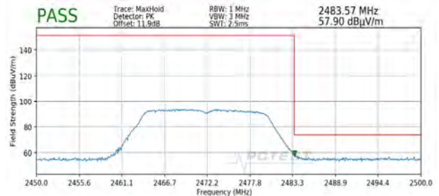
Plot 7-120. Radiated Restricted Upper Band Edge Measurement SISO ANT2 (Peak)
