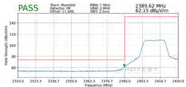
Plot 7-114. Radiated Restricted Lower Band Edge Measurement SISO ANT2 (Peak)
