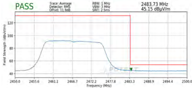
Plot 7-109. Radiated Restricted Upper Band Edge Measurement SISO ANT1 (Average)
