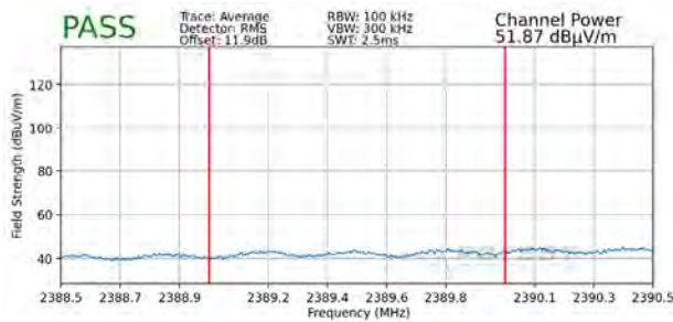
Plot 7-105. Radiated Restricted Lower Band Edge Measurement SISO ANT1 (Average)
