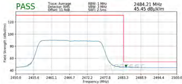
Plot 7-133. Radiated Restricted Upper Band Edge Measurement MIMO (Average - 242 Tones)
