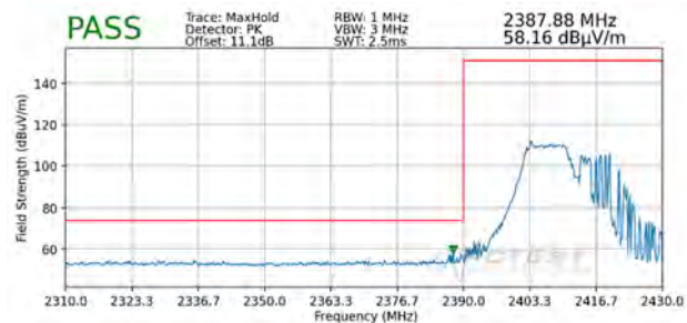
Plot 7-106. Radiated Restricted Lower Band Edge Measurement SISO ANT2 (Peak – 106 Tones)
