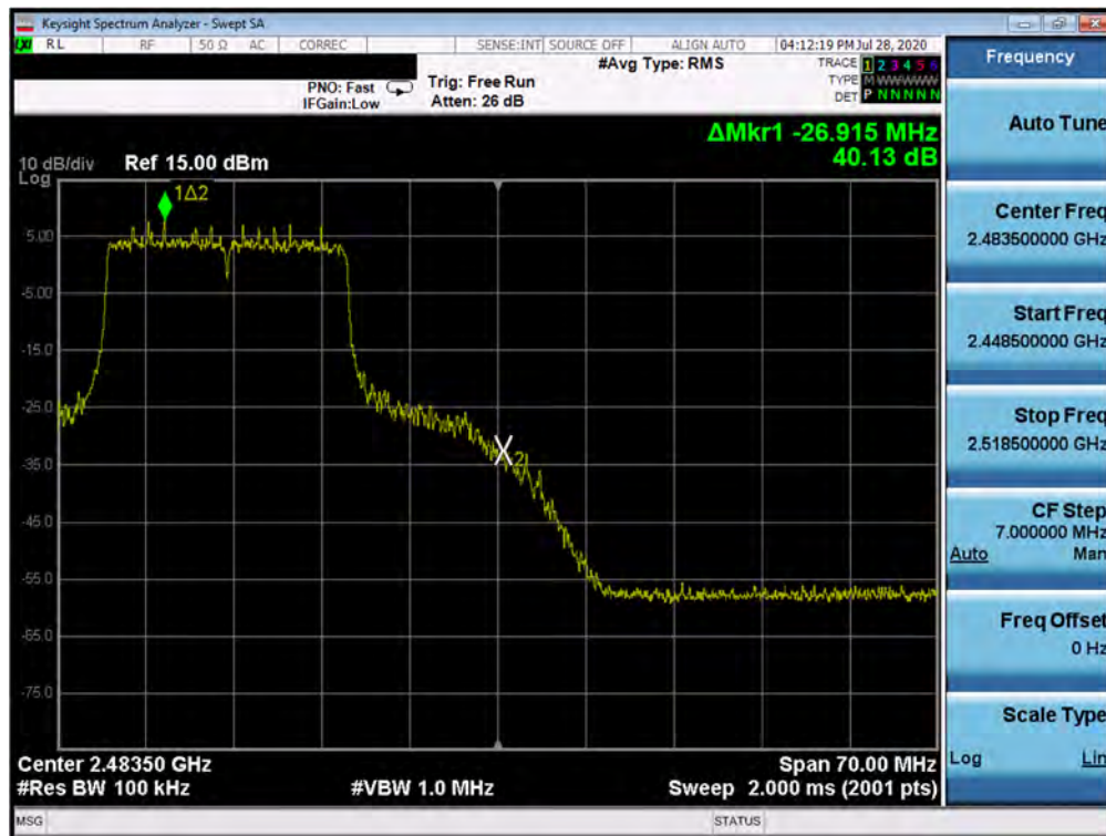
Plot 7-30. Band Edge Plot SISO ANT1 (802.11ax OFDMA - 242 Tones - Ch. 11)
