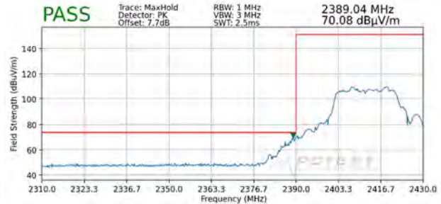
Plot 7-130. Radiated Restricted Lower Band Edge Measurement MIMO (Peak - 242 Tones)
