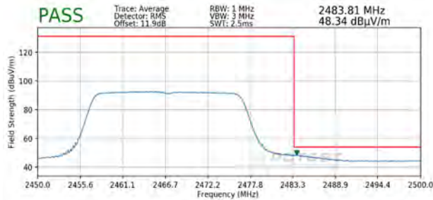
Plot 7-117. Radiated Restricted Upper Band Edge Measurement SISO ANT2 (Average – 242 Tones)
