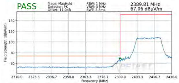
Plot 7-114. Radiated Restricted Lower Band Edge Measurement SISO ANT2 (Peak - 242 Tones)
