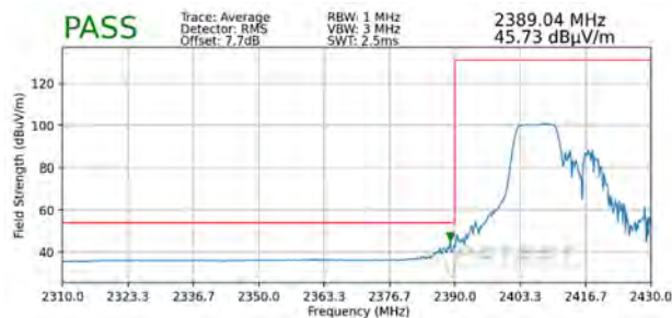
Plot 7-121. Radiated Restricted Lower Band Edge Measurement MIMO (Average – 106 Tones)
