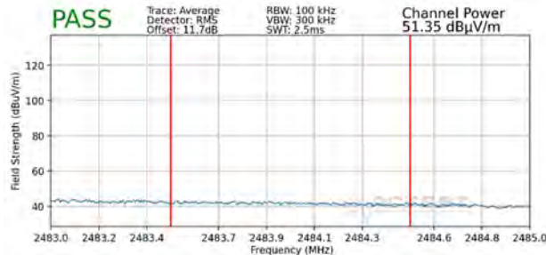
Plot 7-99. Radiated Restricted Upper Band Edge Measurement SISO ANT1 (Average - 242 Tones)
