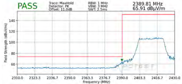
Plot 7-98. Radiated Restricted Lower Band Edge Measurement SISO ANT1 (Peak - 242 Tones)
