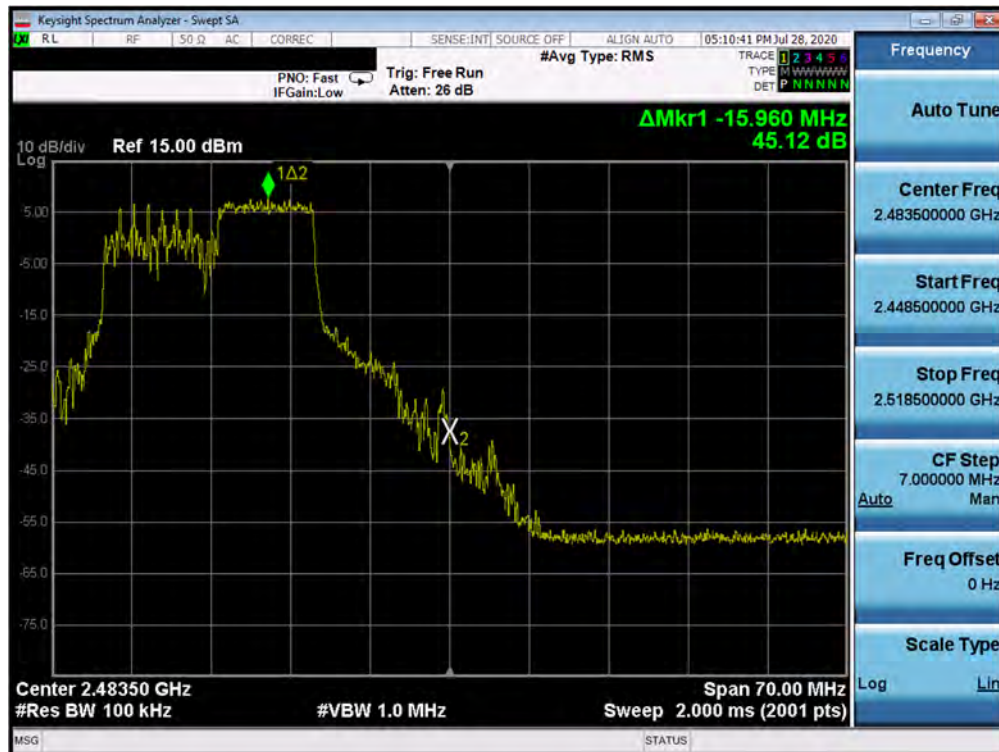
Plot 7-34. Band Edge Plot SISO ANT2 (802.11ax OFDMA – 106 Tones – Ch. 11)
