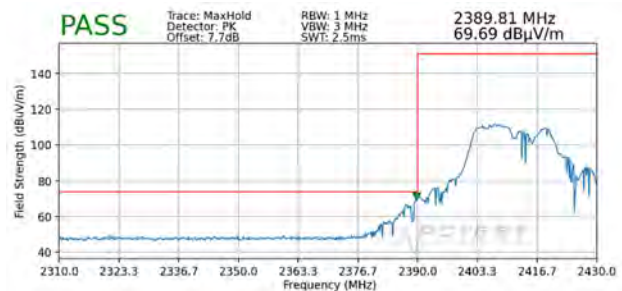
Plot 7-122. Radiated Restricted Lower Band Edge Measurement MIMO (Peak – 106 Tones)
