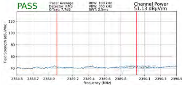
Plot 7-129. Radiated Restricted Lower Band Edge Measurement MIMO (Average - 242 Tones)
