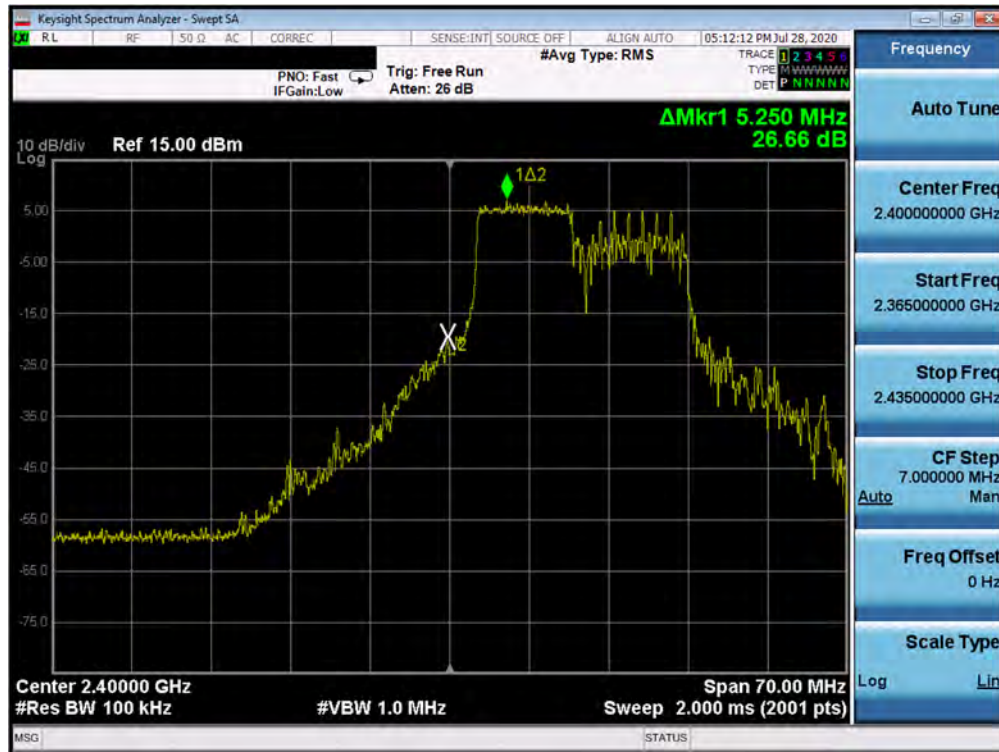
Plot 7-33. Band Edge Plot SISO ANT2 (802.11ax OFDMA – 106 Tones – Ch. 1)
