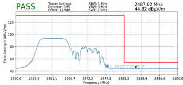
Plot 7-125. Radiated Restricted Lower Band Edge Measurement MIMO (Average - 106 Tones)
