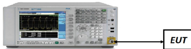
Figure 7-5. Test Instrument & Measurement Setup
