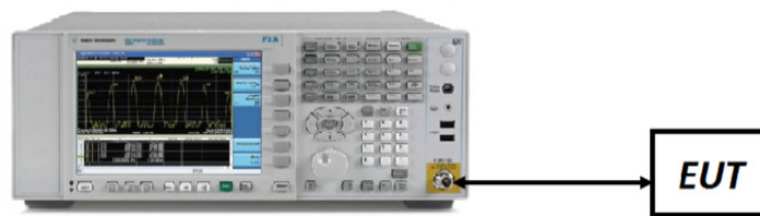
Figure 7-3. Test Instrument & Measurement Setup
