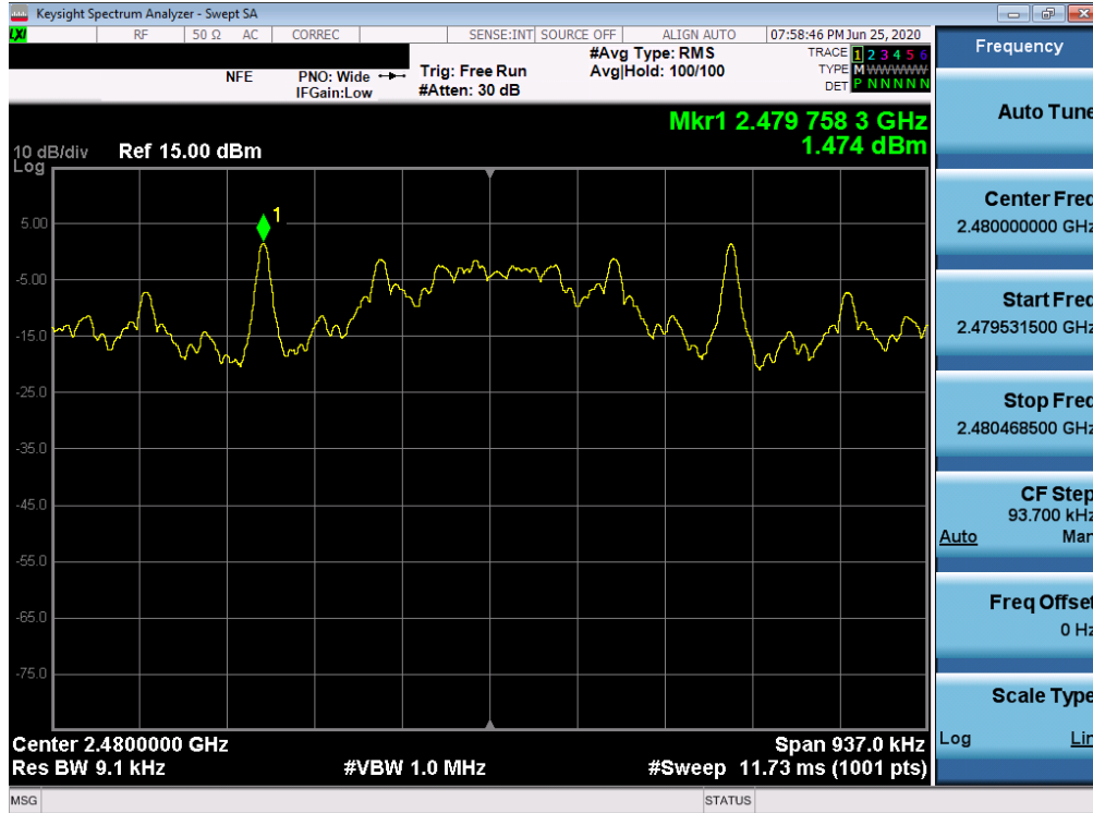
Plot 7-27. Power Spectral Density Plot (Bluetooth (LE), 125kbps – Ch. 39)
