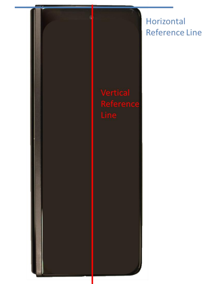
SAR Test Setup Photo 32– Closed Configuration (Handset) Horizontal and Vertical Reference Lines
