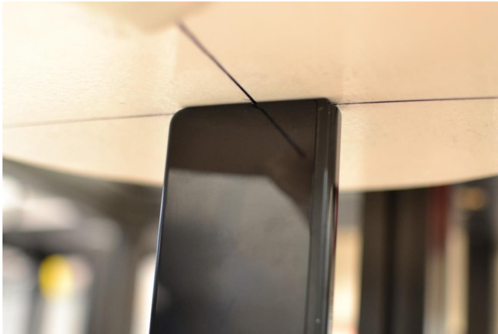
SAR Test Setup Photo 14– Closed Configuration (Handset), Phablet, Bottom Edge, 0 mm
