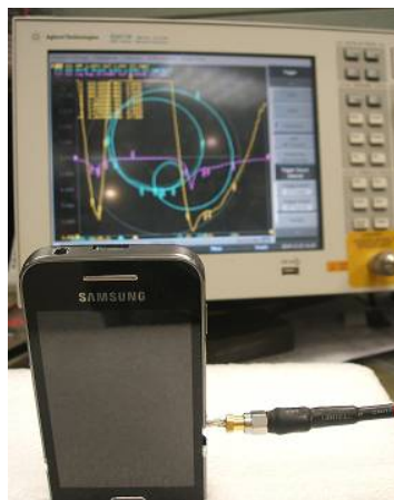
Figure 1: Testing with network analyzer
