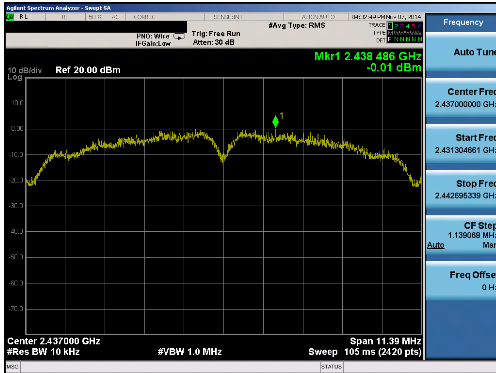
Plot 6-11. Power Spectral Density Plot (802.11b – Ch. 6)
