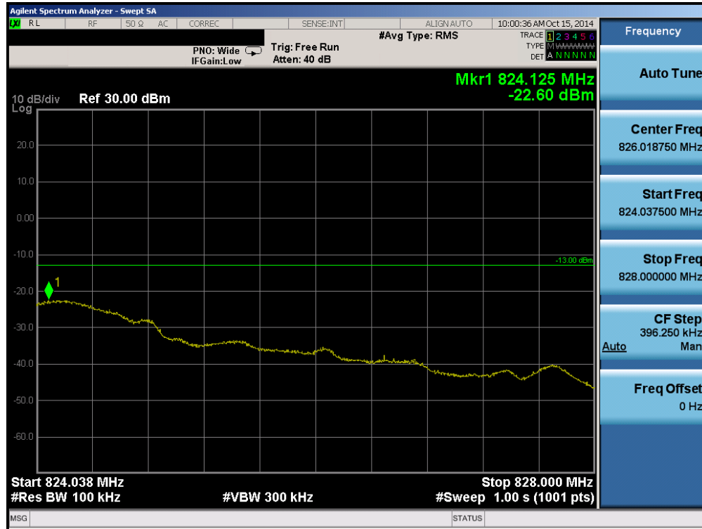
Plot 7-10. Outer Extended Band Edge Plot (Ch. 684)
