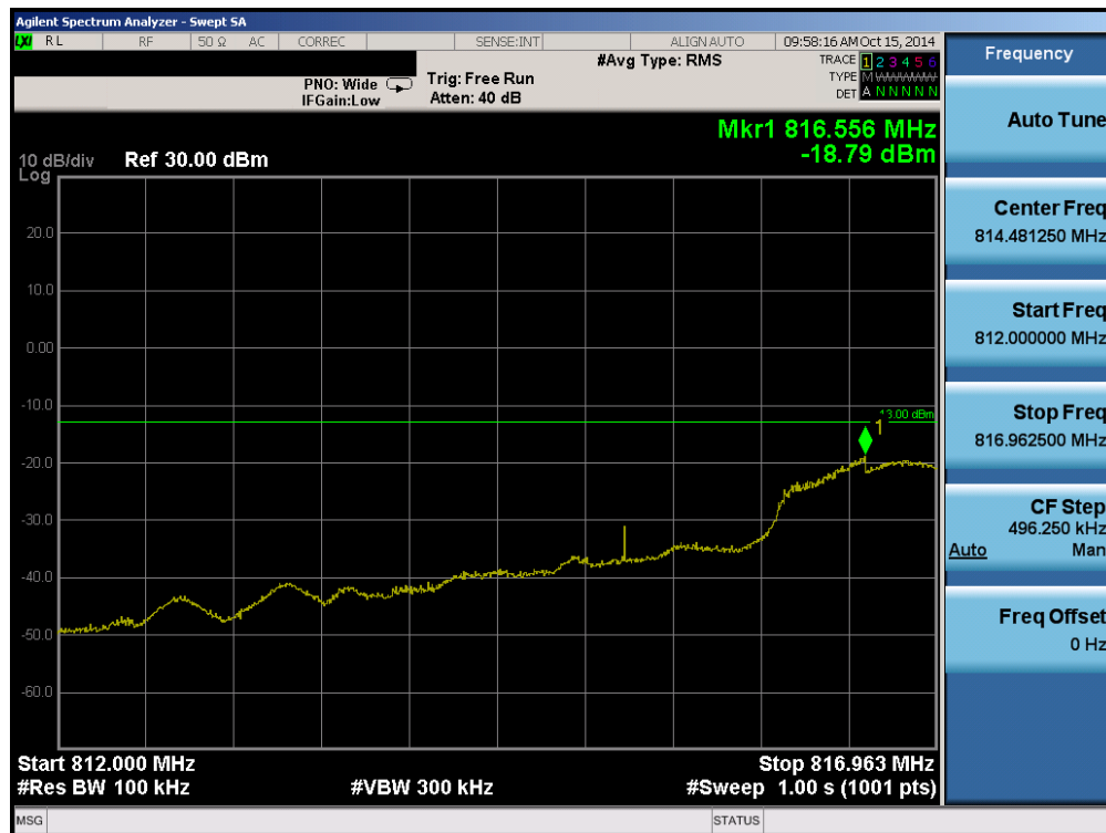
Plot 7-5. Outer Extended Band Edge Plot (Ch. 476)
