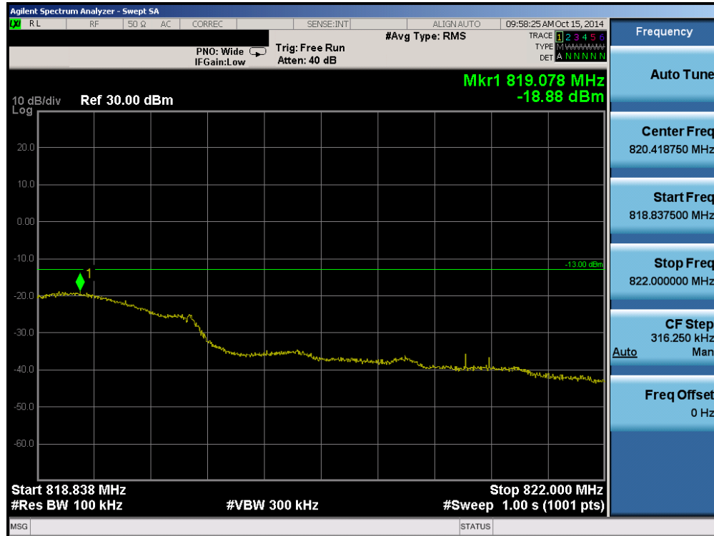
Plot 7-4. Inner Extended Band Edge Plot (Ch. 476)
