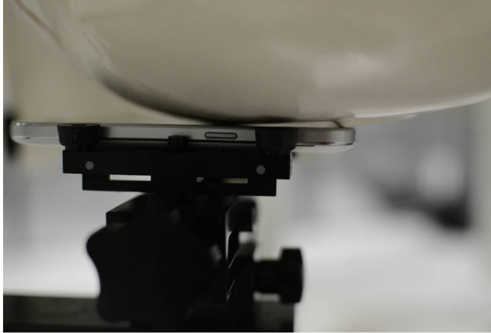
SAR Test Setup Photo 3: Left Cheek
