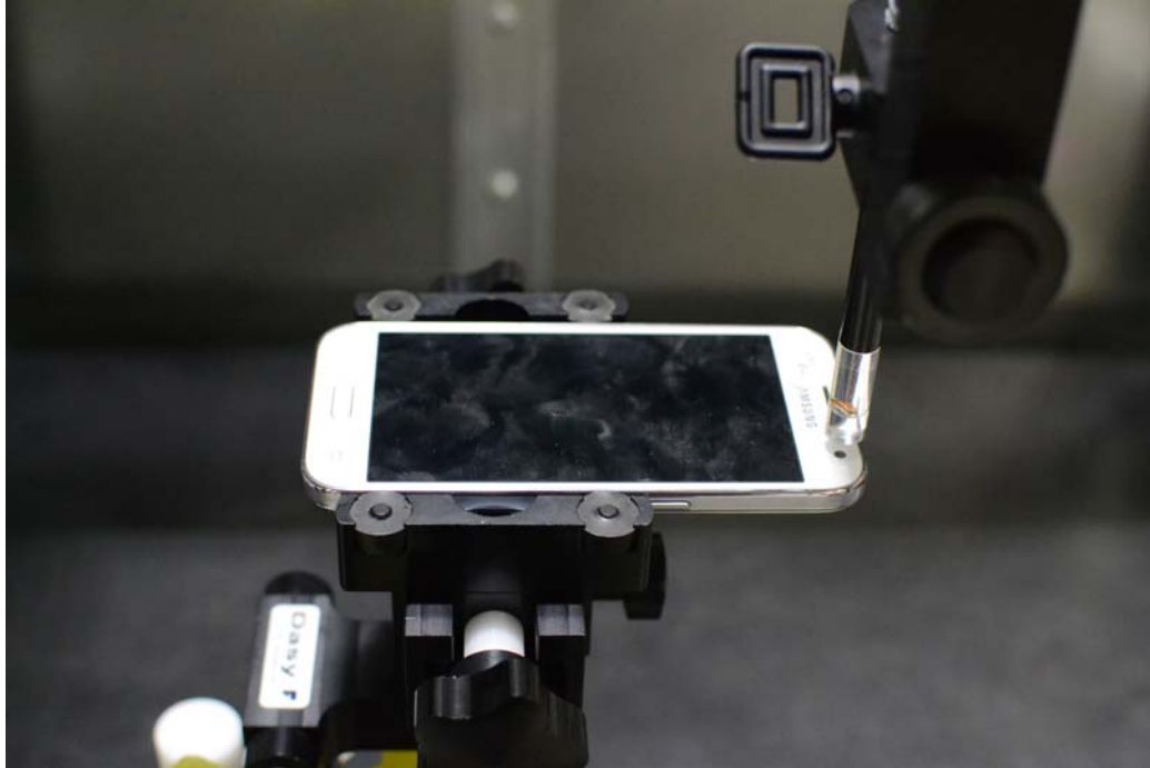
Figure 13-1 Test Setup for Wireless Device
