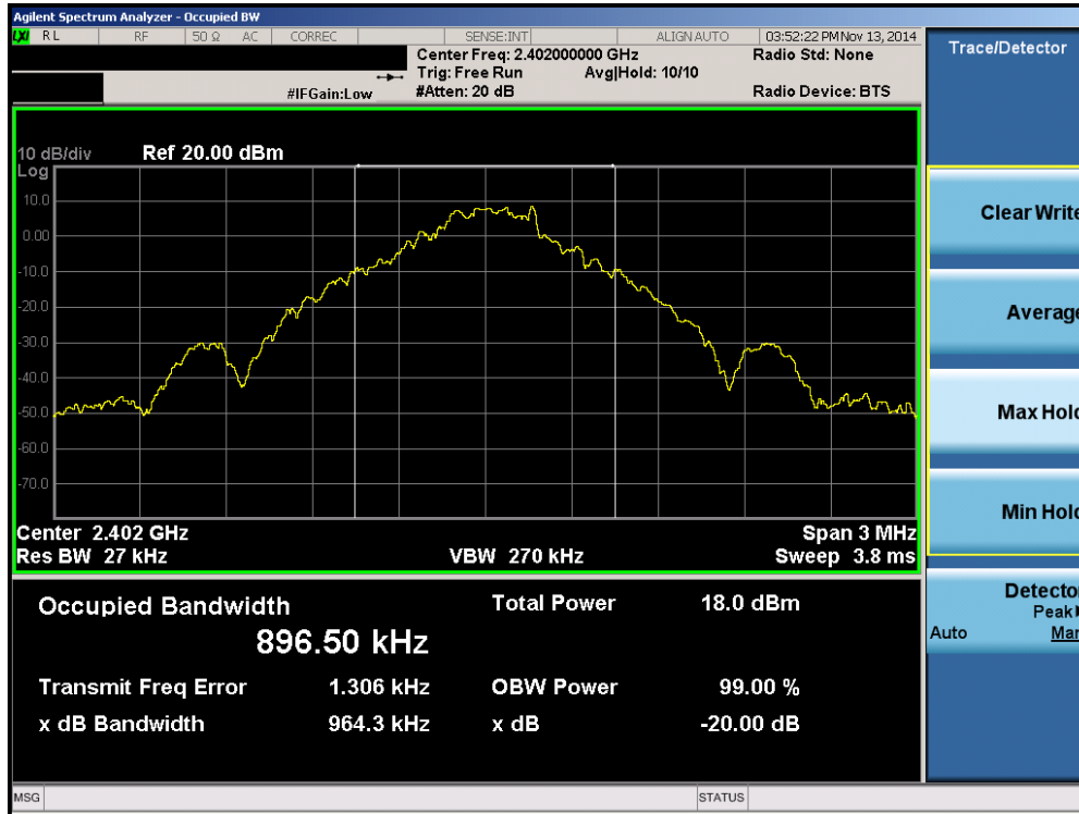
Plot 6-1. 20dB Bandwidth Plot (Bluetooth, 1Mbps – Ch. 0)
