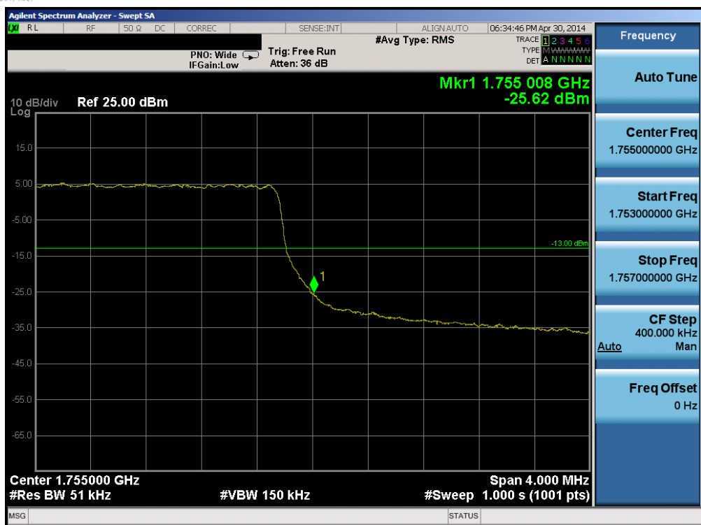
Plot 6-107. Upper Band Edge Plot (Band 4 – 5.0MHz QPSK – RB Size 25)
