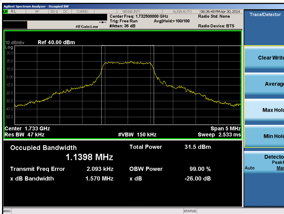
Plot 6-17. Occupied Bandwidth Plot (Band 4 – 1.4MHz QPSK – RB Size 6)
