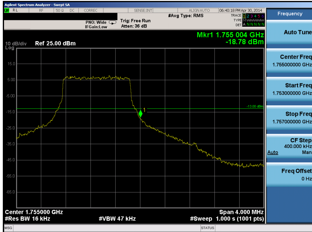
Plot 6-99. Upper Band Edge Plot (Band 4 – 1.4MHz QPSK – RB Size 6)
