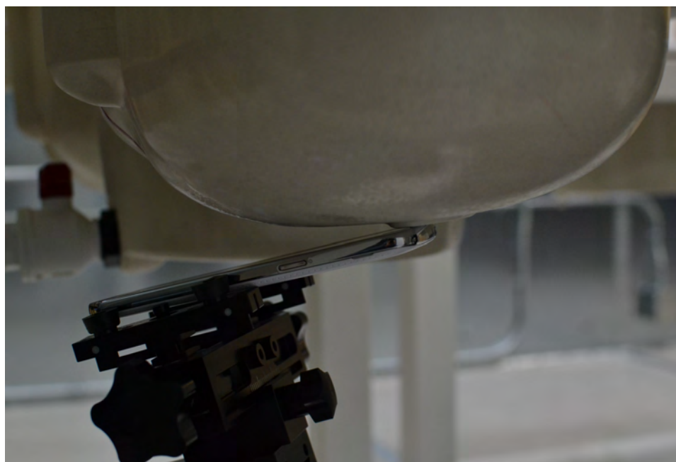
SAR Test Setup Photo 4 – Left Tilt
