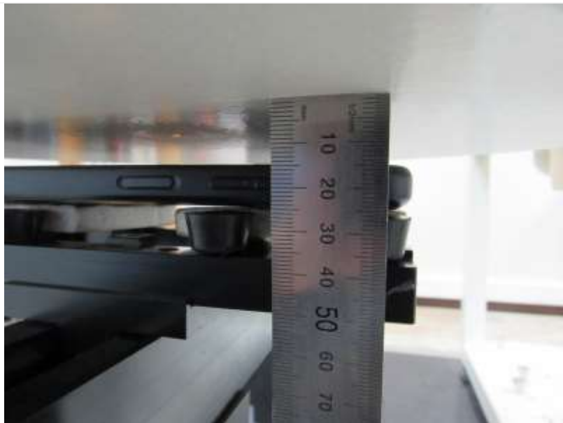
Distance of 15 mm from the EUT
