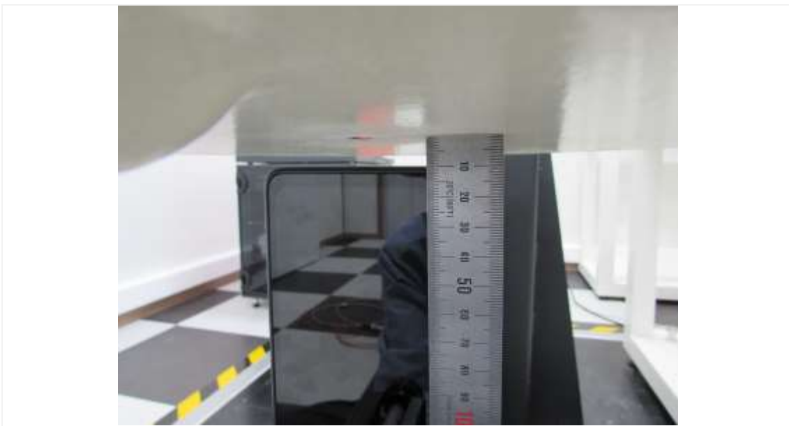
Distance of 10 mm from the EUT
