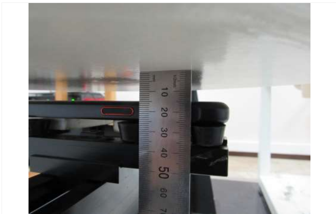
Distance of 15 mm from the EUT
