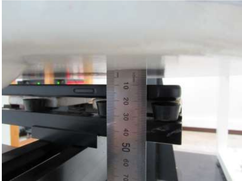
Distance of 10 mm from the EUT
