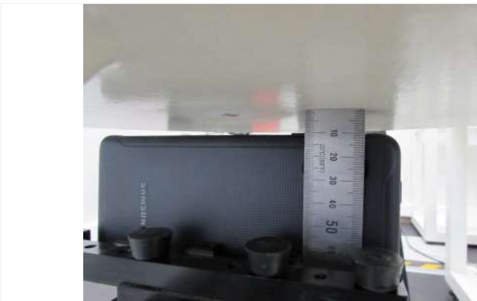
Distance of 10 mm from the EUT
