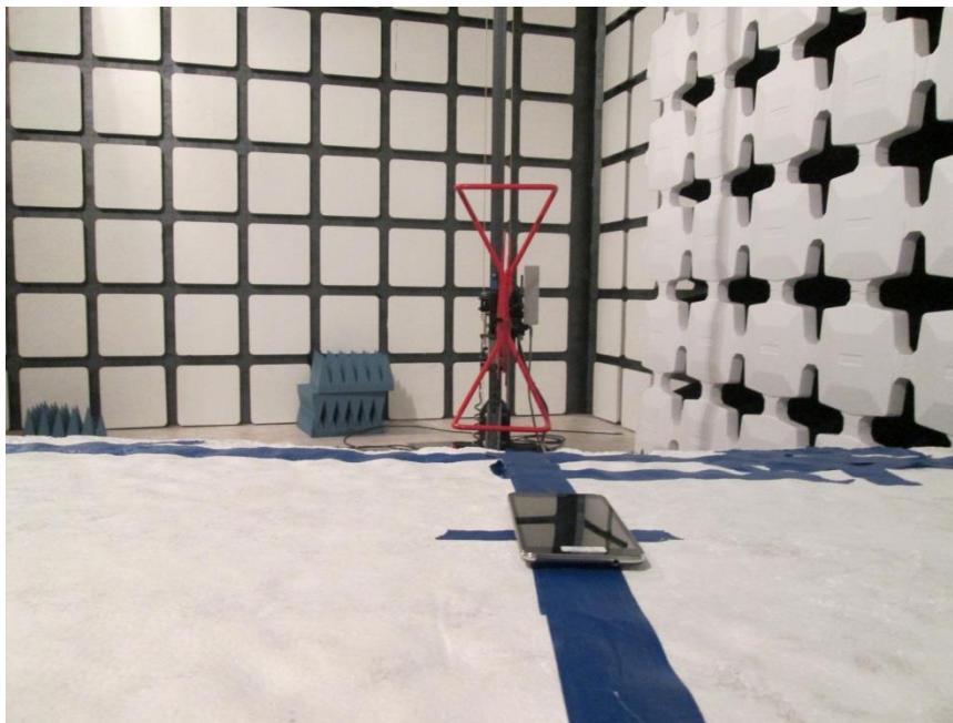
RADIATED FRONT PHOTO (BELOW 1 GHz)
