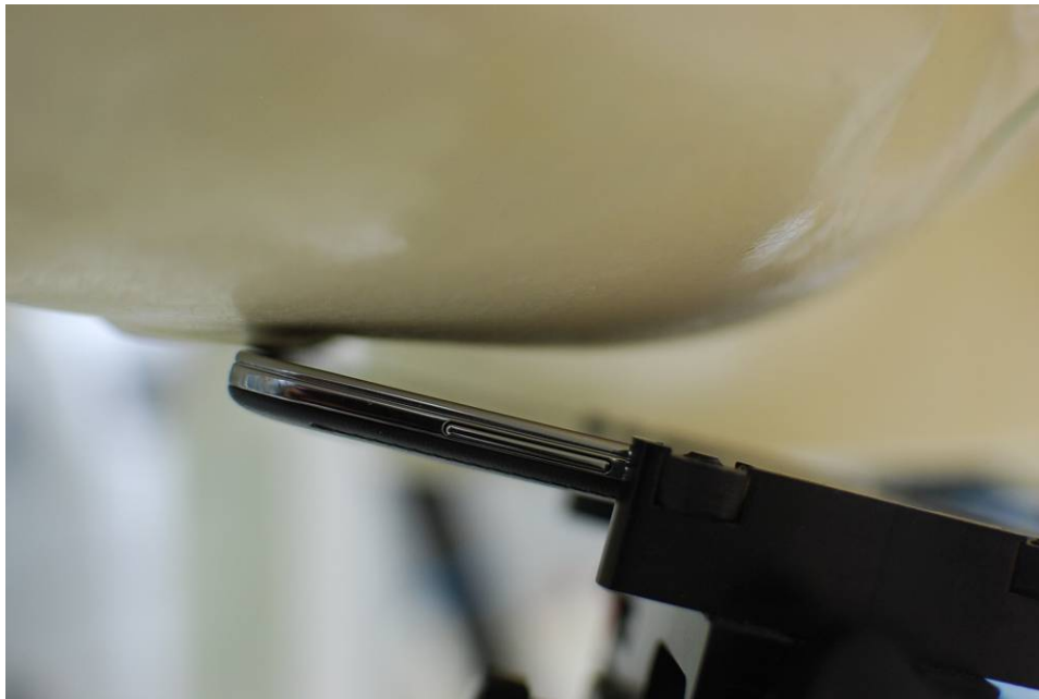
SAR Test Setup Photo 2 – Right Tilt
