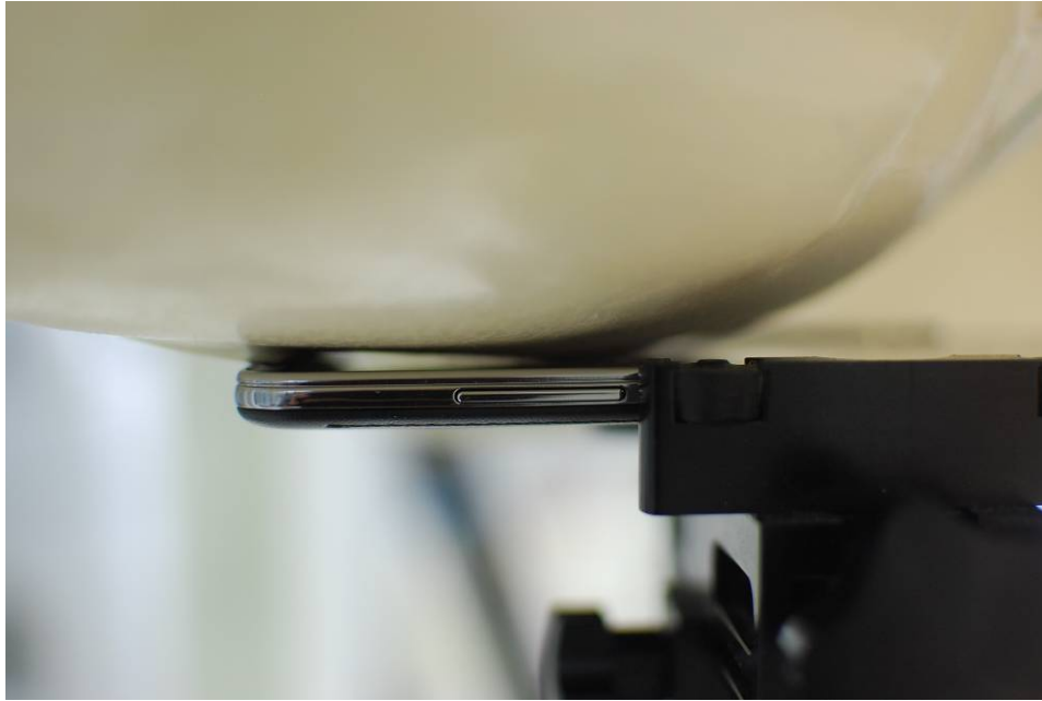
SAR Test Setup Photo 1 – Right Cheek
