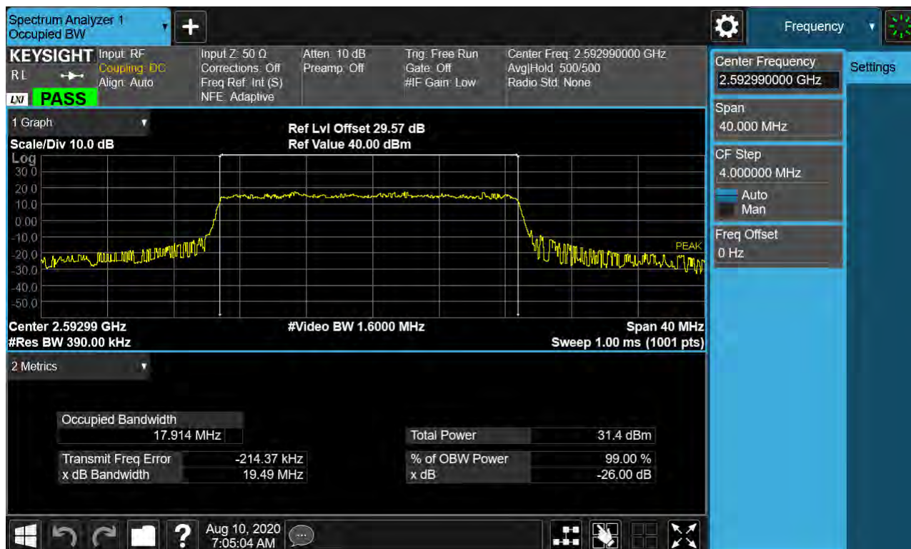
Sub6 n41. Occupied Bandwidth Plot (20 MHz Ch.518598 BPSK RB 25)_SCS 30 kHz
