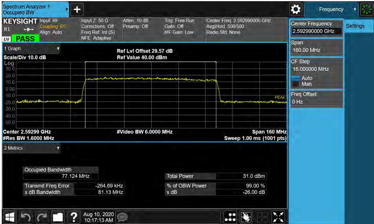
Sub6 n41. Occupied Bandwidth Plot (80 MHz Ch.518598 QPSK RB 25) _SCS 30 kHz
