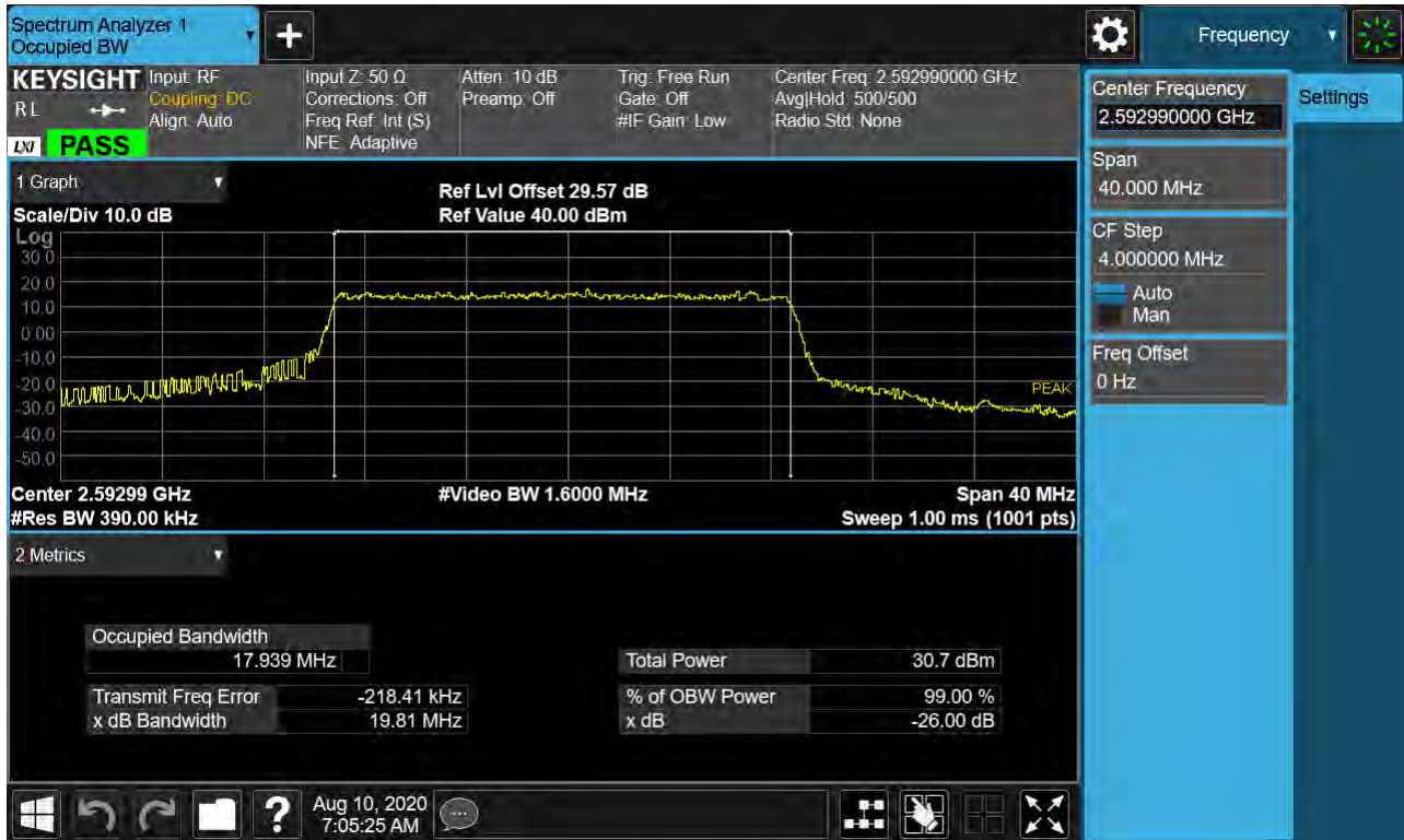
Sub6 n41. Occupied Bandwidth Plot (20 MHz Ch.518598 QPSK RB 25) _SCS 30 kHz
