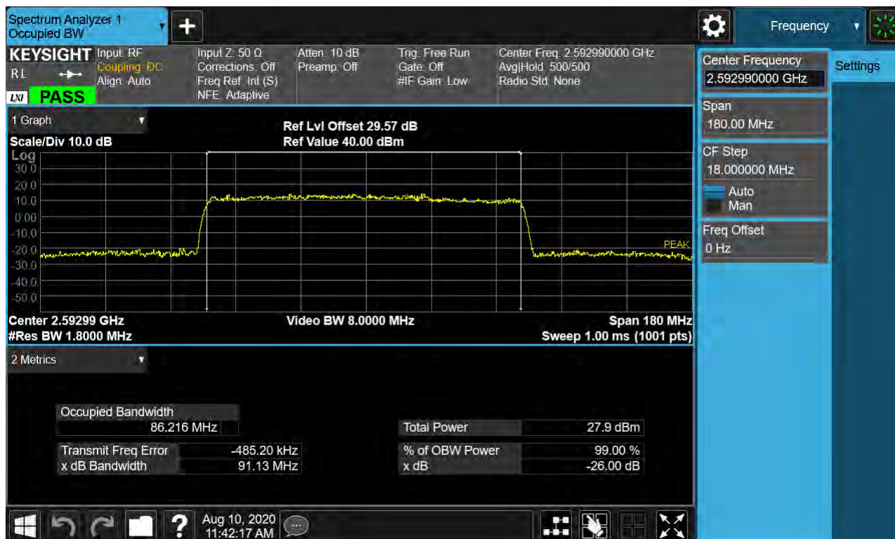
Sub6 n41. Occupied Bandwidth Plot (90 MHz Ch.518598 256-QAM RB 25) _SCS 30 kHz
