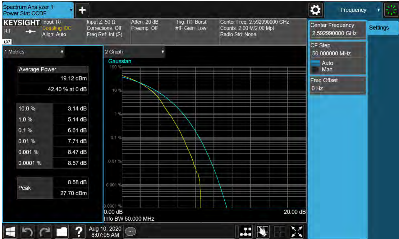
Sub6 n41. PAR Plot (50M BW_Ch.518598_256QAM_RB25_0)
