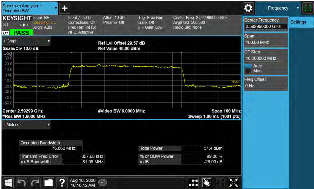
Sub6 n41. Occupied Bandwidth Plot (80 MHz Ch.518598 BPSK RB 25) _SCS 30 kHz
