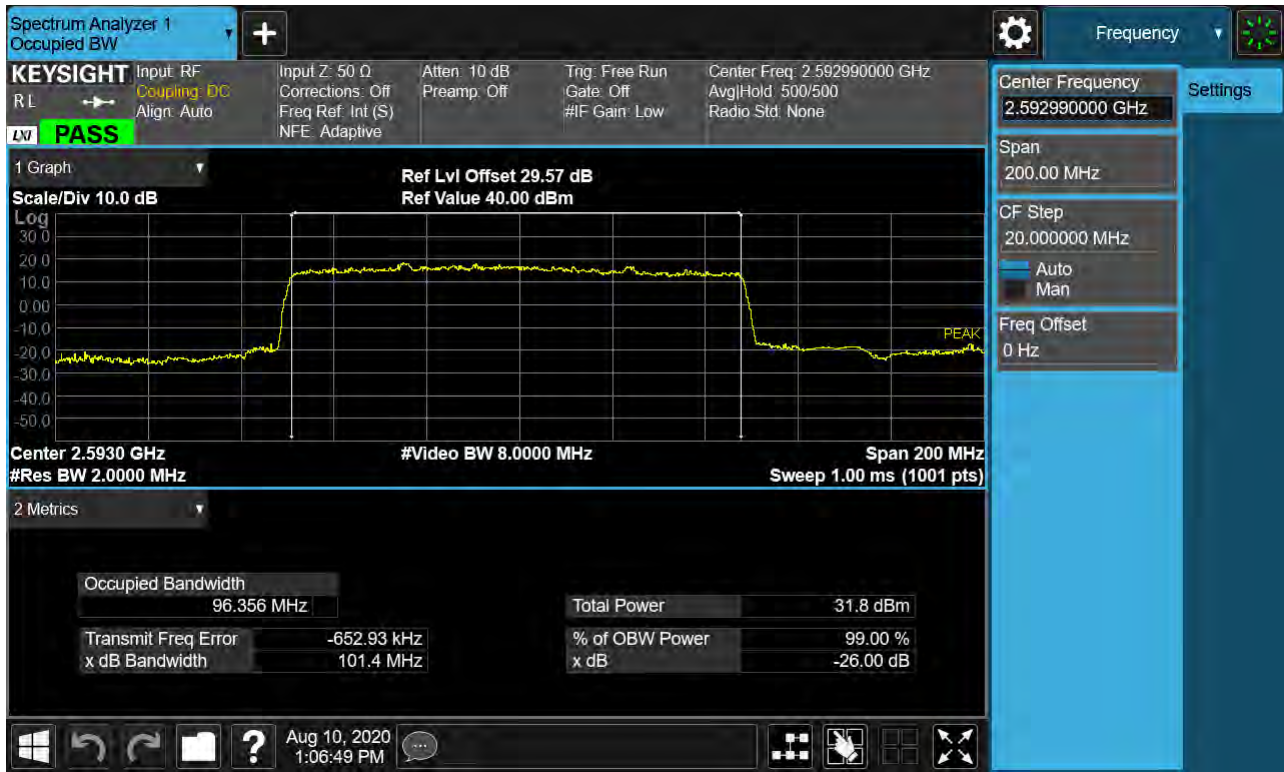
Sub6 n41. Occupied Bandwidth Plot (100 MHz Ch.518598 BPSK RB 25)_SCS 30 kHz
