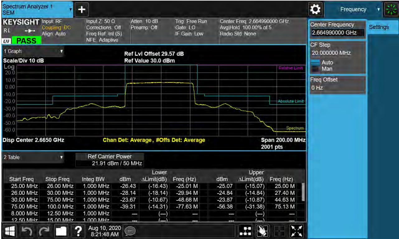
Sub6 n41. High Channel Edge Plot (50 MHz Ch.532998 BPSK_RB25_Offset 0)
