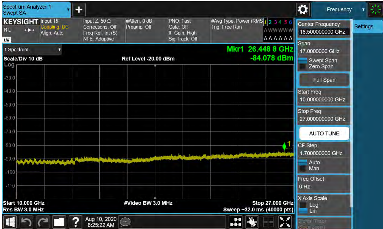
Sub6 n41. Conducted Spurious Plot 2 (50 MHz Ch.532998 BPSK RB 1, Offset 0)
