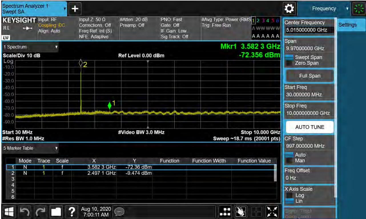
Sub6 n41. Conducted Spurious Plot 1 (20 MHz Ch.501204 BPSK RB 1, Offset 0)
