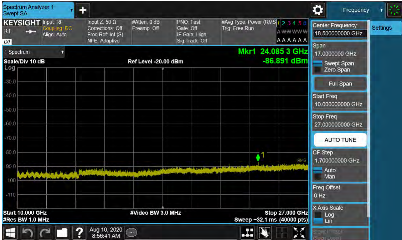
Sub6 n41. Conducted Spurious Plot 2 (60 MHz Ch.531996 BPSK RB 1, Offset 0)
