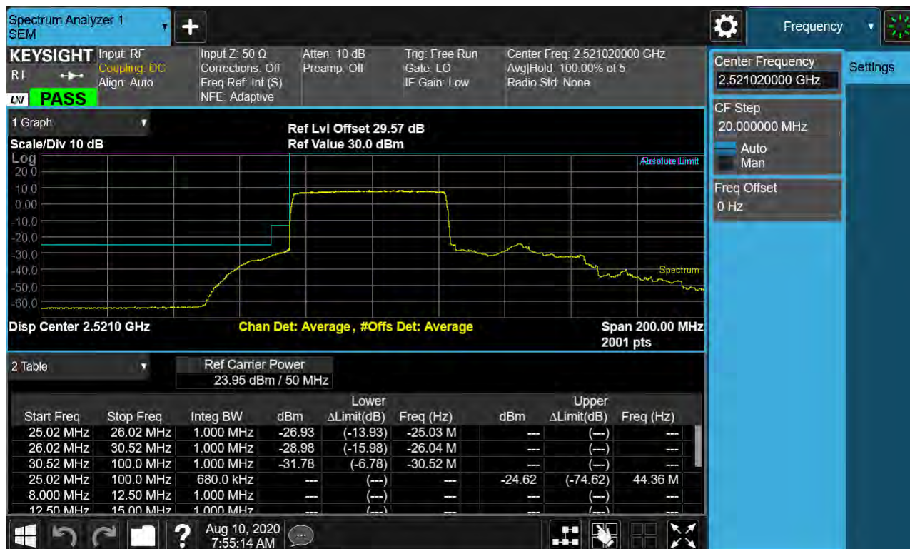
Sub6 n41. Low Channel Edge Plot (50 MHz Ch.504204 BPSK RB 25, Offset 0)-1
