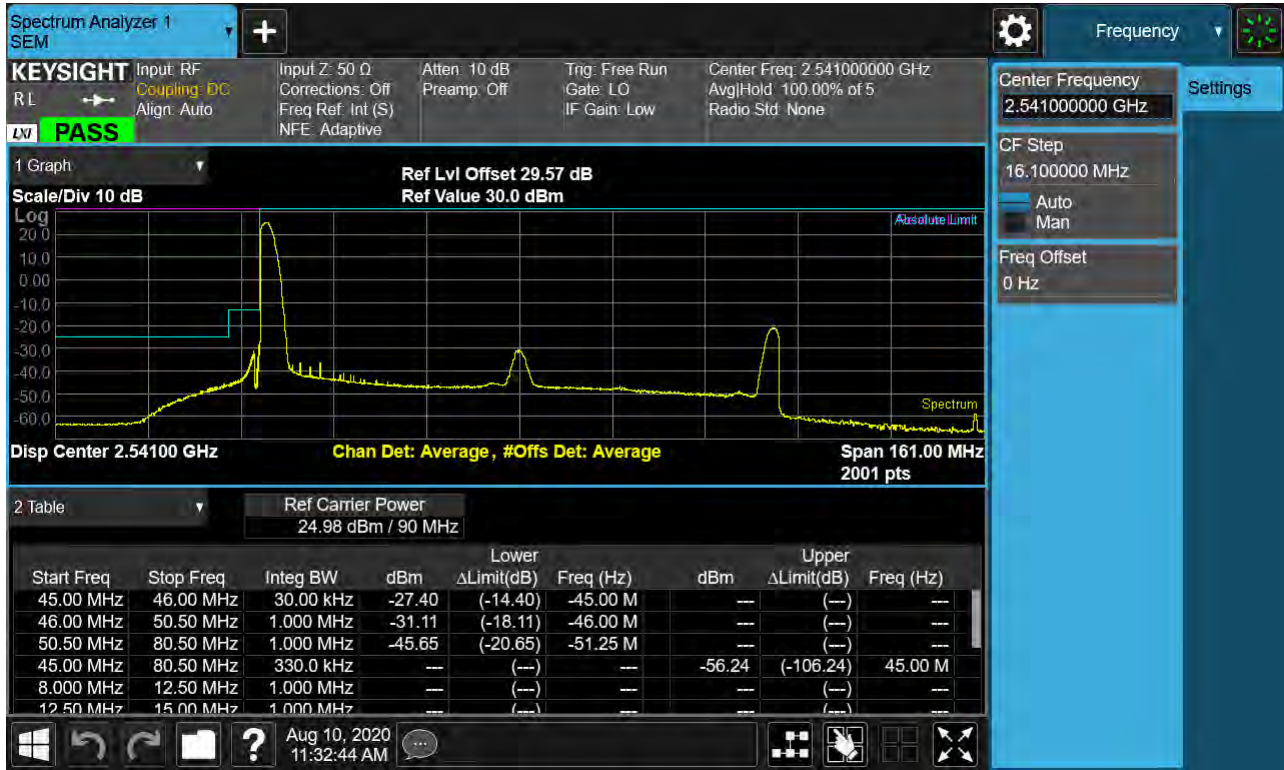
Sub6 n41. Low Channel Edge Plot (90 MHz Ch.508200 BPSK RB 1, Offset 0)-1
