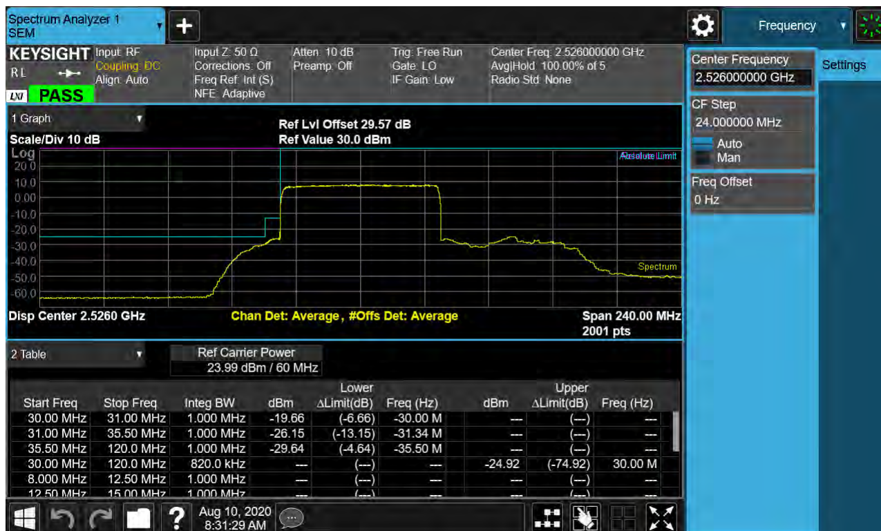
Sub6 n41. Low Channel Edge Plot (60 MHz Ch.505200 BPSK RB 25, Offset 0)-1
