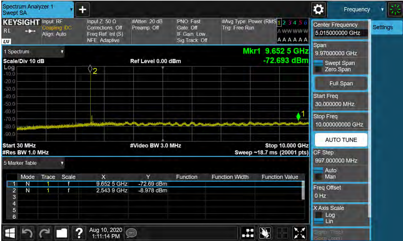
Sub6 n41. Conducted Spurious Plot 1 (100 MHz Ch.518598 BPSK RB 1, Offset 0)
