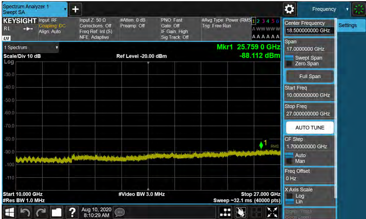
Sub6 n41. Conducted Spurious Plot 2 (50 MHz Ch. 518598 BPSK RB 1, Offset 0)
