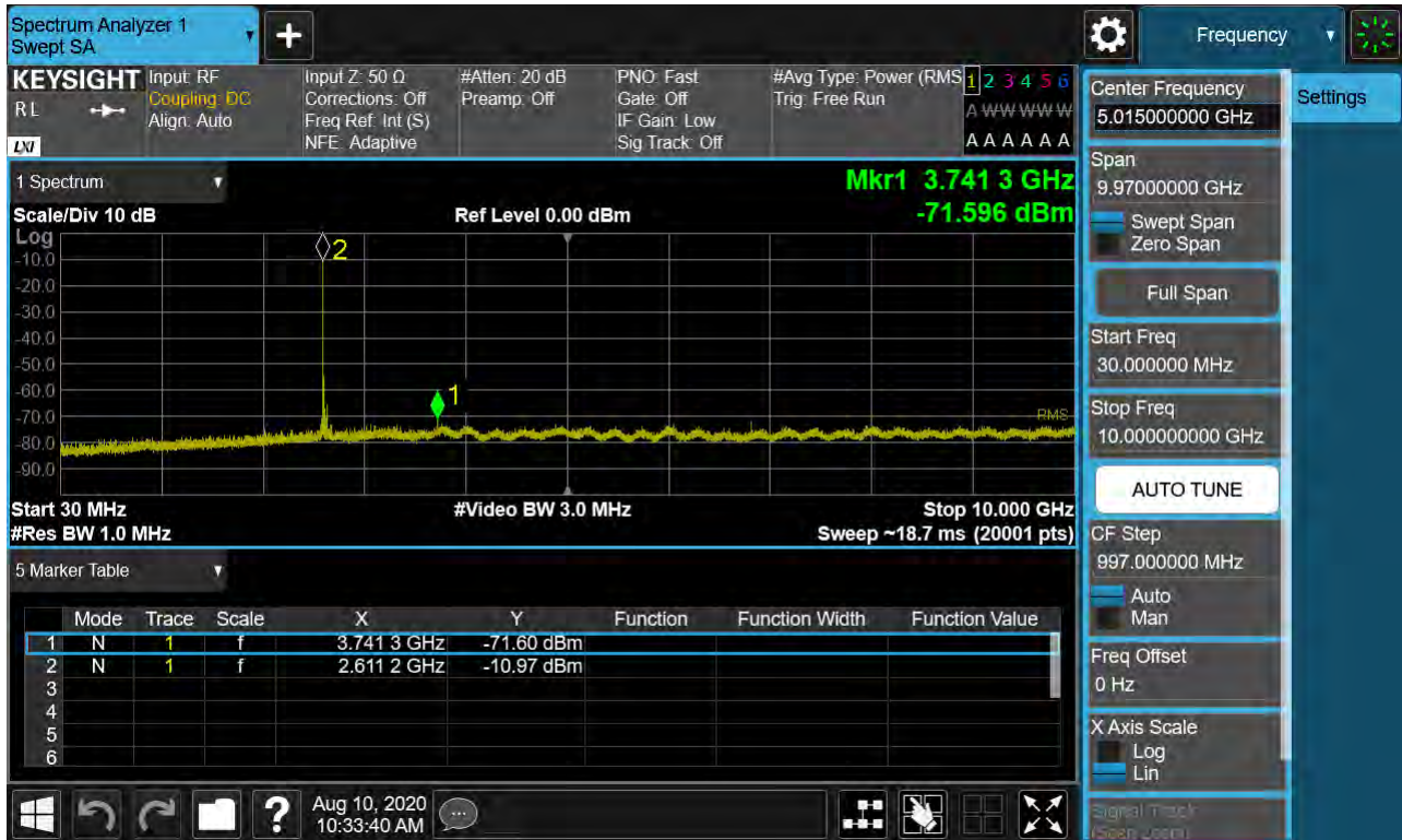
Sub6 n41. Conducted Spurious Plot 1 (80 MHz Ch.529998 BPSK RB 1, Offset 0)
