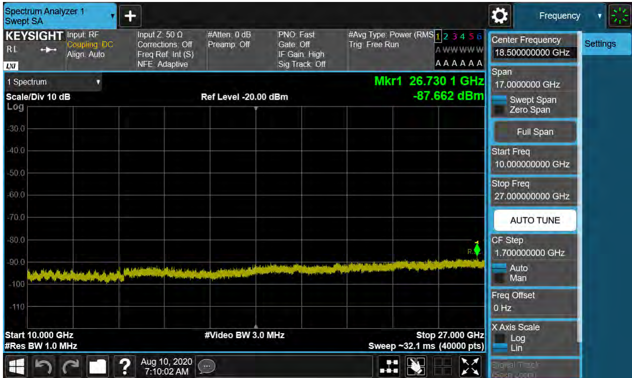
Sub6 n41. Conducted Spurious Plot 2 (20 MHz Ch. 518598 BPSK RB 1, Offset 0)
