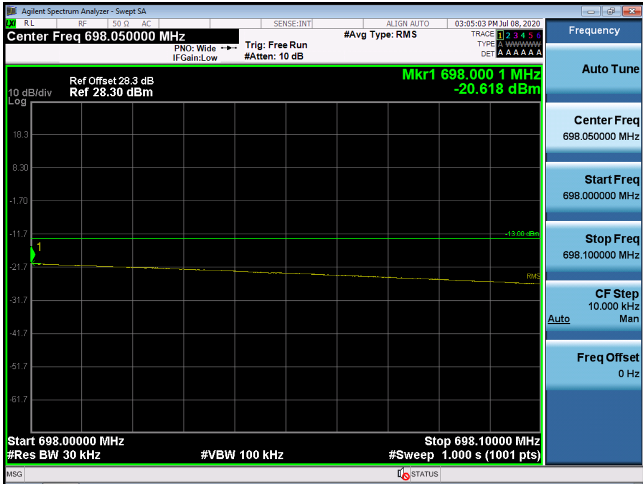
Sub6 n71. Upper Band Edge Plot (10M BW Ch.138600 BPSK_RB1_Offset 14)-1
