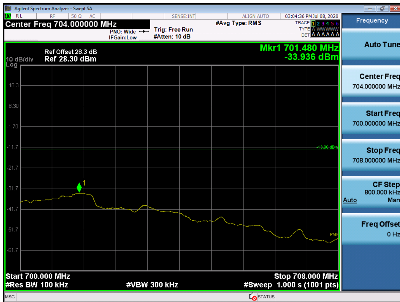
Sub6 n71. Upper Extended Band Edge Plot (10M BW Ch.138600 BPSK_RB15_0)
