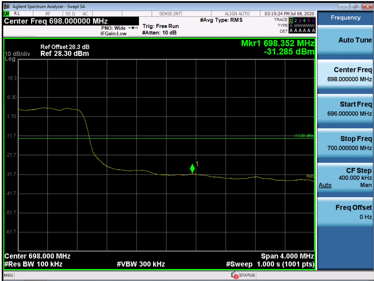
Sub6 n71. Upper Band Edge Plot (15M BW Ch.138100 BPSK_RB25_Offset 0)
