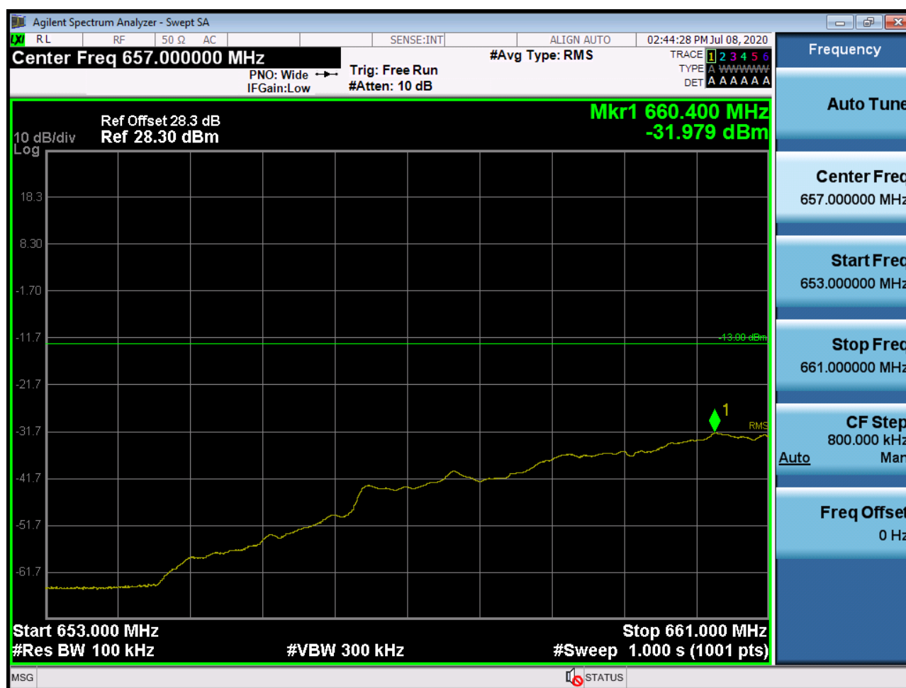
Sub6 n71. Lower Extended Band Edge Plot (10M BW Ch.133600 BPSK_RB15_0)
