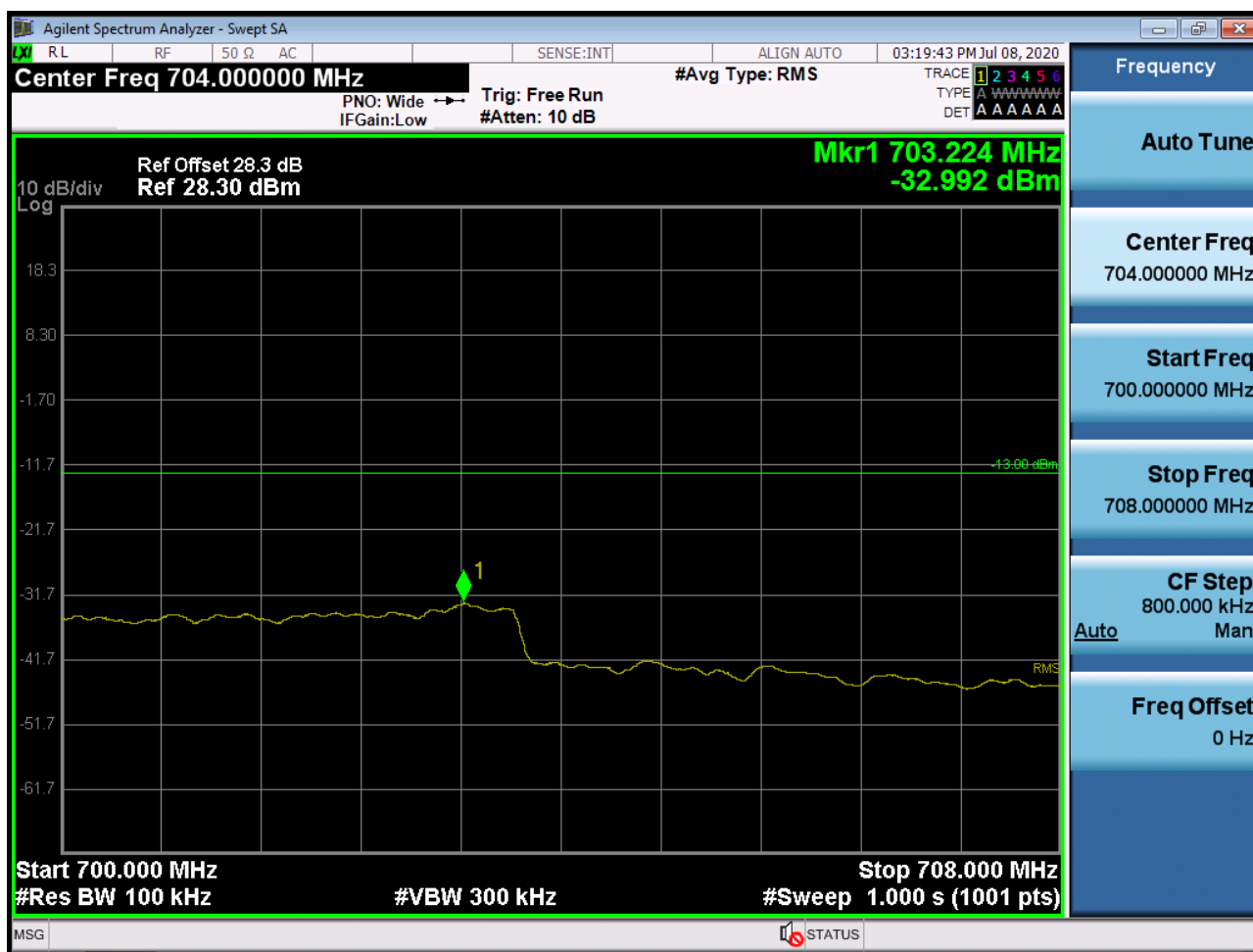
Sub6 n71. Upper Extended Band Edge Plot (15M BW Ch.138100 BPSK_RB25_0)
