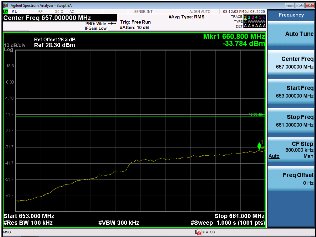
Sub6 n71. Lower Extended Band Edge Plot (15M BW Ch.134100 BPSK_RB25_0)
