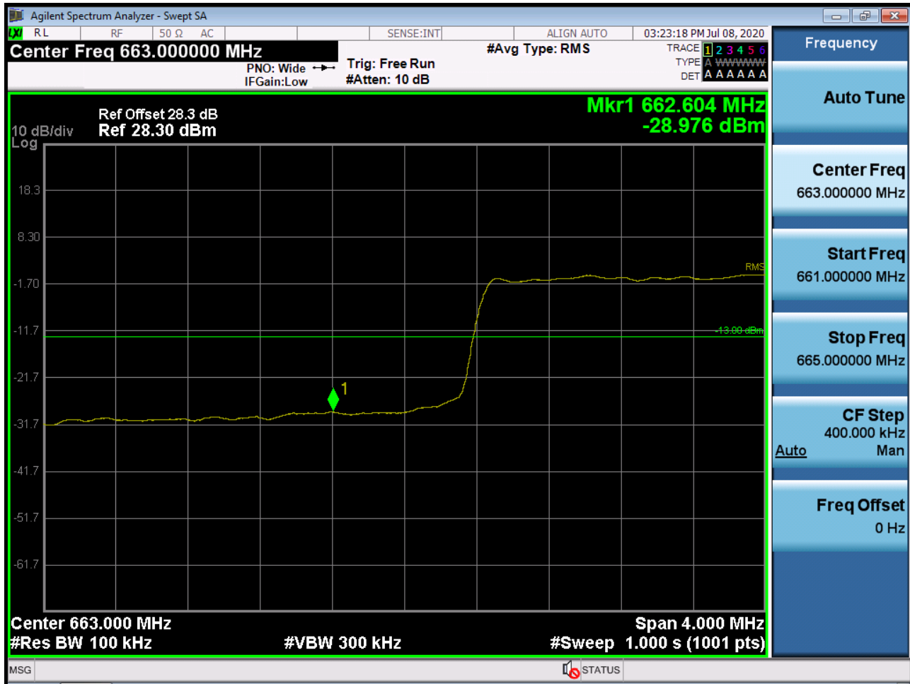
Sub6 n71. Lower Band Edge Plot (20M BW Ch.134600 BPSK_RB50_Offset 0)
