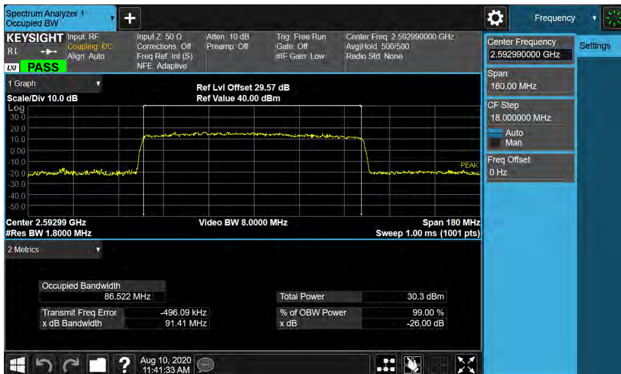
Sub6 n41. Occupied Bandwidth Plot (90 MHz Ch.518598 16-QAM RB 25)_SCS 30 kHz
