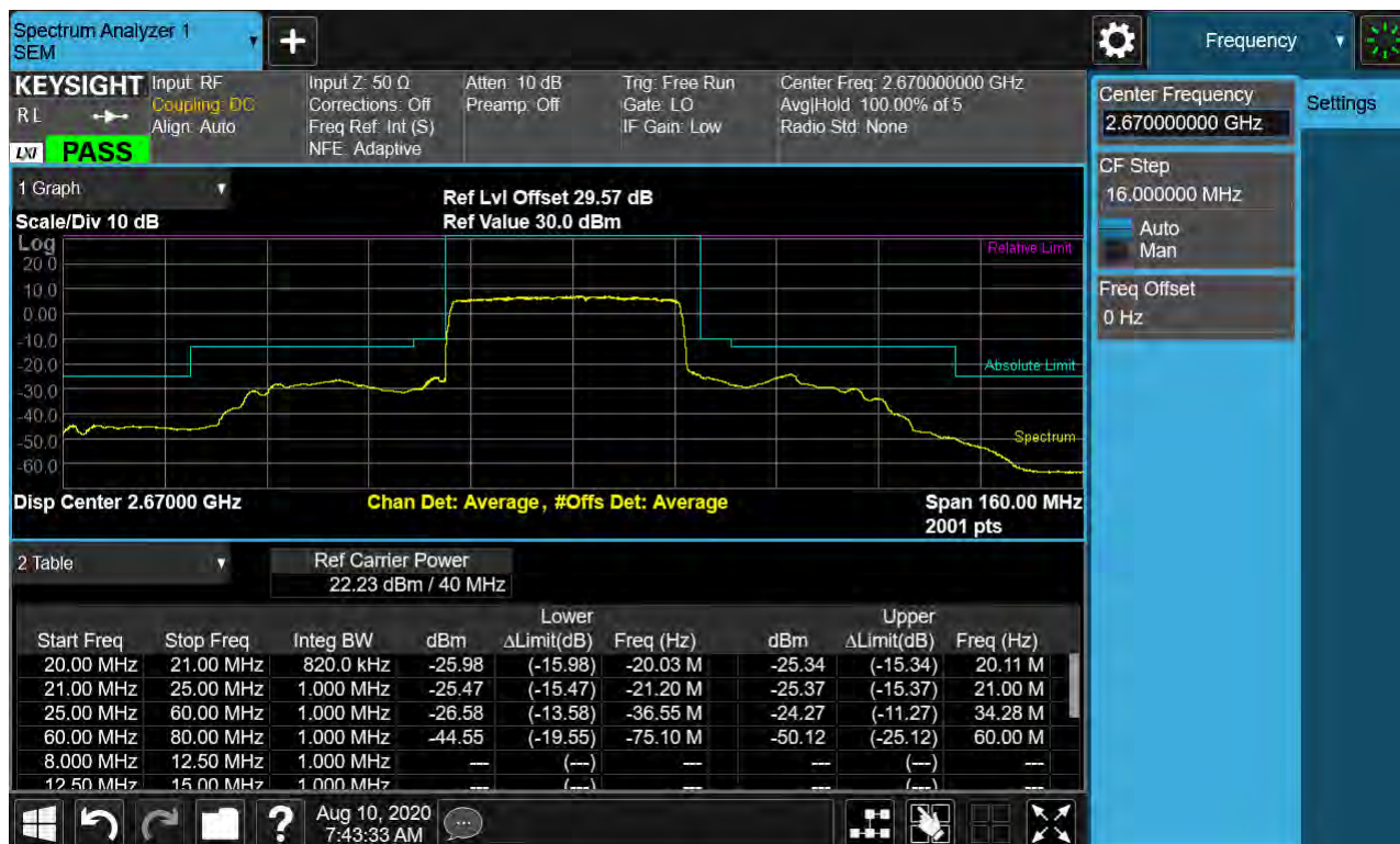
Sub6 n41. High Channel Edge Plot (40 MHz Ch.534000 BPSK_RB25_Offset 0)
