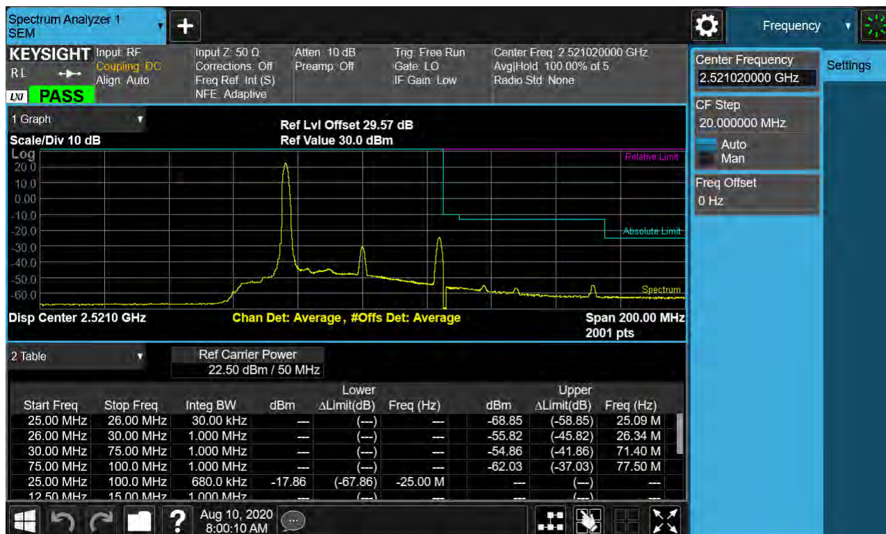
Sub6 n41. Low Channel Edge Plot (50 MHz Ch.504204 BPSK_RB1_Offset 0)-2
