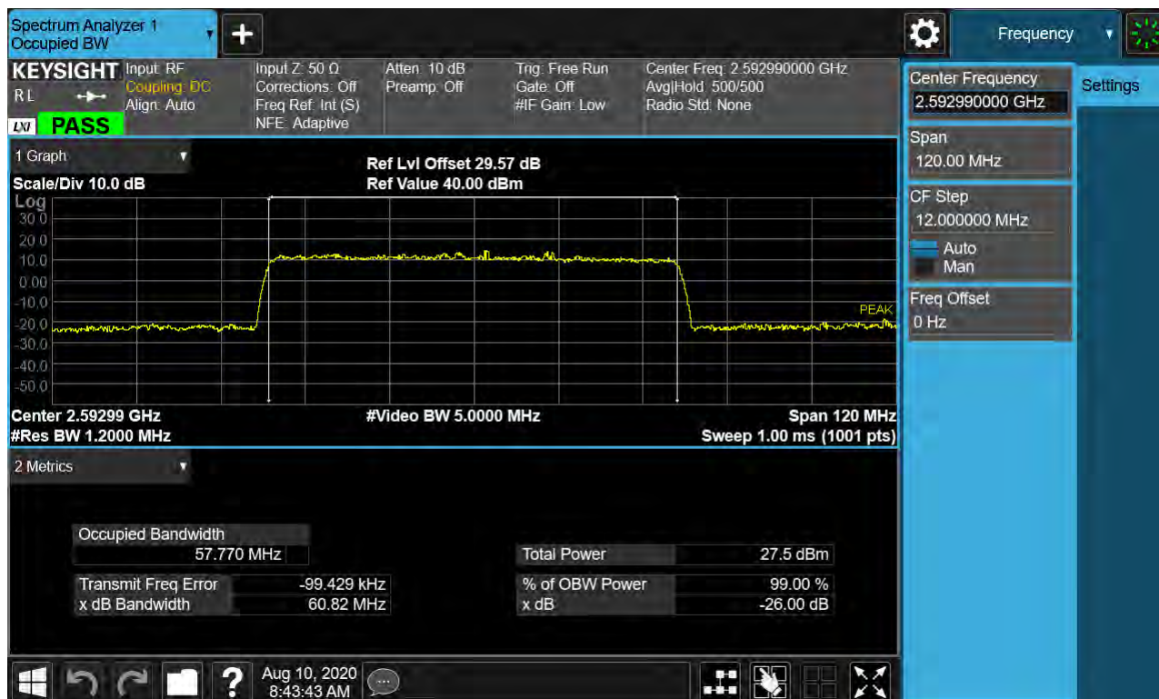
Sub6 n41. Occupied Bandwidth Plot (60 MHz Ch.518598 256-QAM RB 25) _SCS 30 kHz
