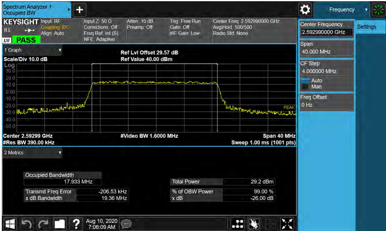
Sub6 n41. Occupied Bandwidth Plot (20 MHz Ch.518598 64-QAM RB 25)_SCS 30 kHz
