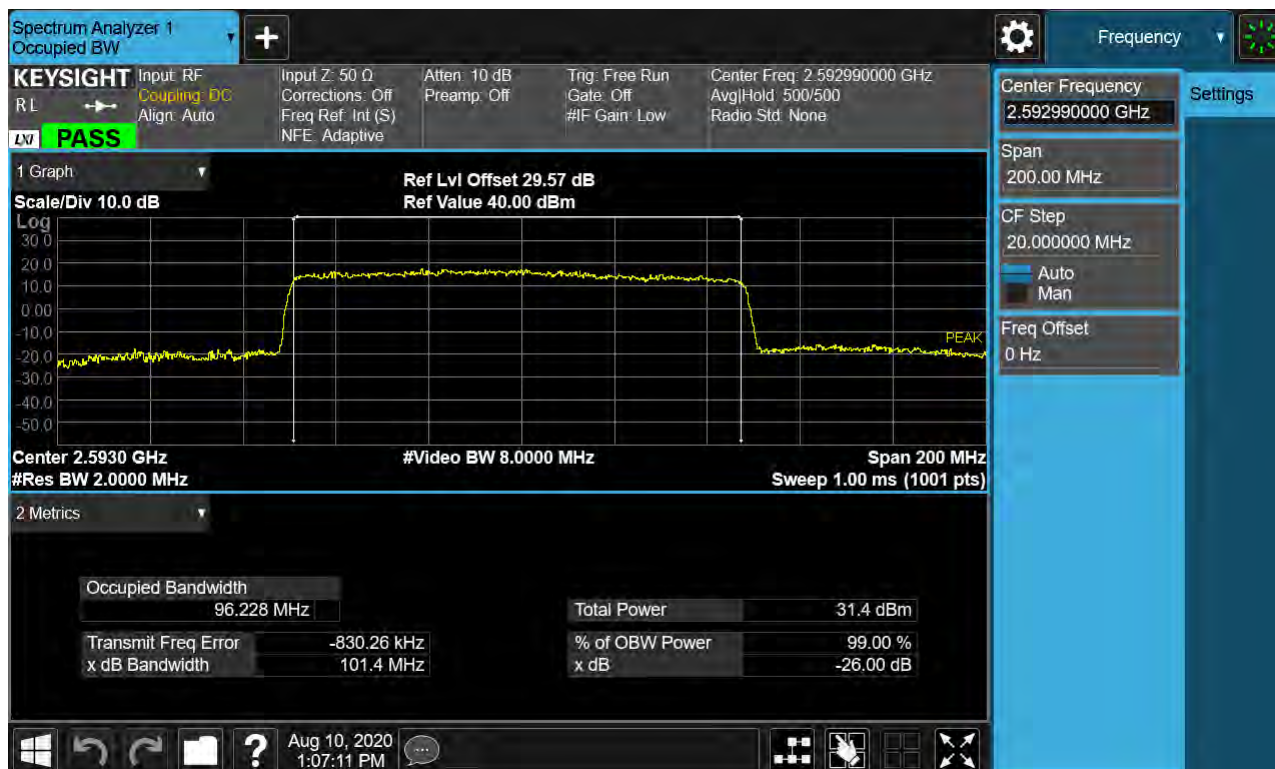
Sub6 n41. Occupied Bandwidth Plot (100 MHz Ch.518598 QPSK RB 25)_SCS 30 kHz
