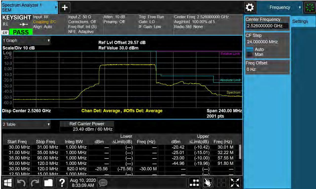
Sub6 n41. Low Channel Edge Plot (60 MHz Ch.505200 BPSK_RB25_Offset 0)-2
