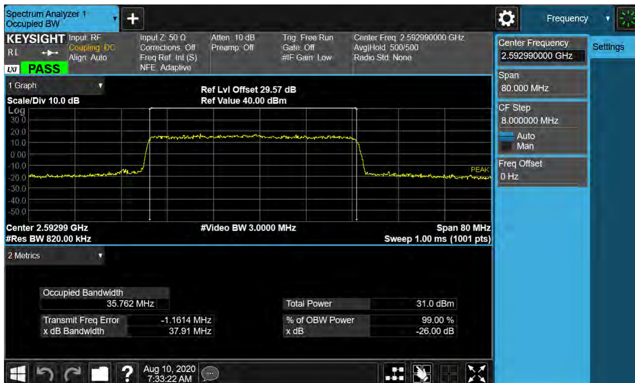
Sub6 n41. Occupied Bandwidth Plot (40 MHz Ch.518598 QPSK RB 25) _SCS 30 kHz
