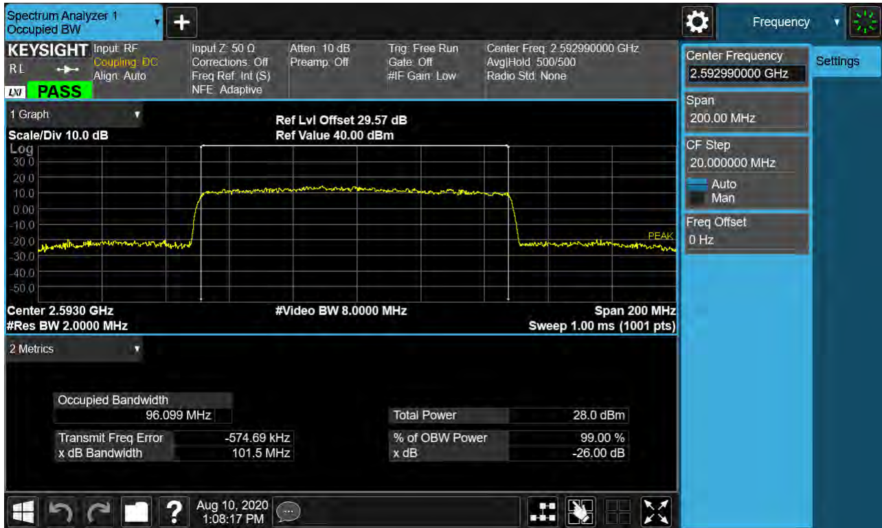
Sub6 n41. Occupied Bandwidth Plot (100 MHz Ch.518598 256-QAM RB 25)_SCS 30 kHz
