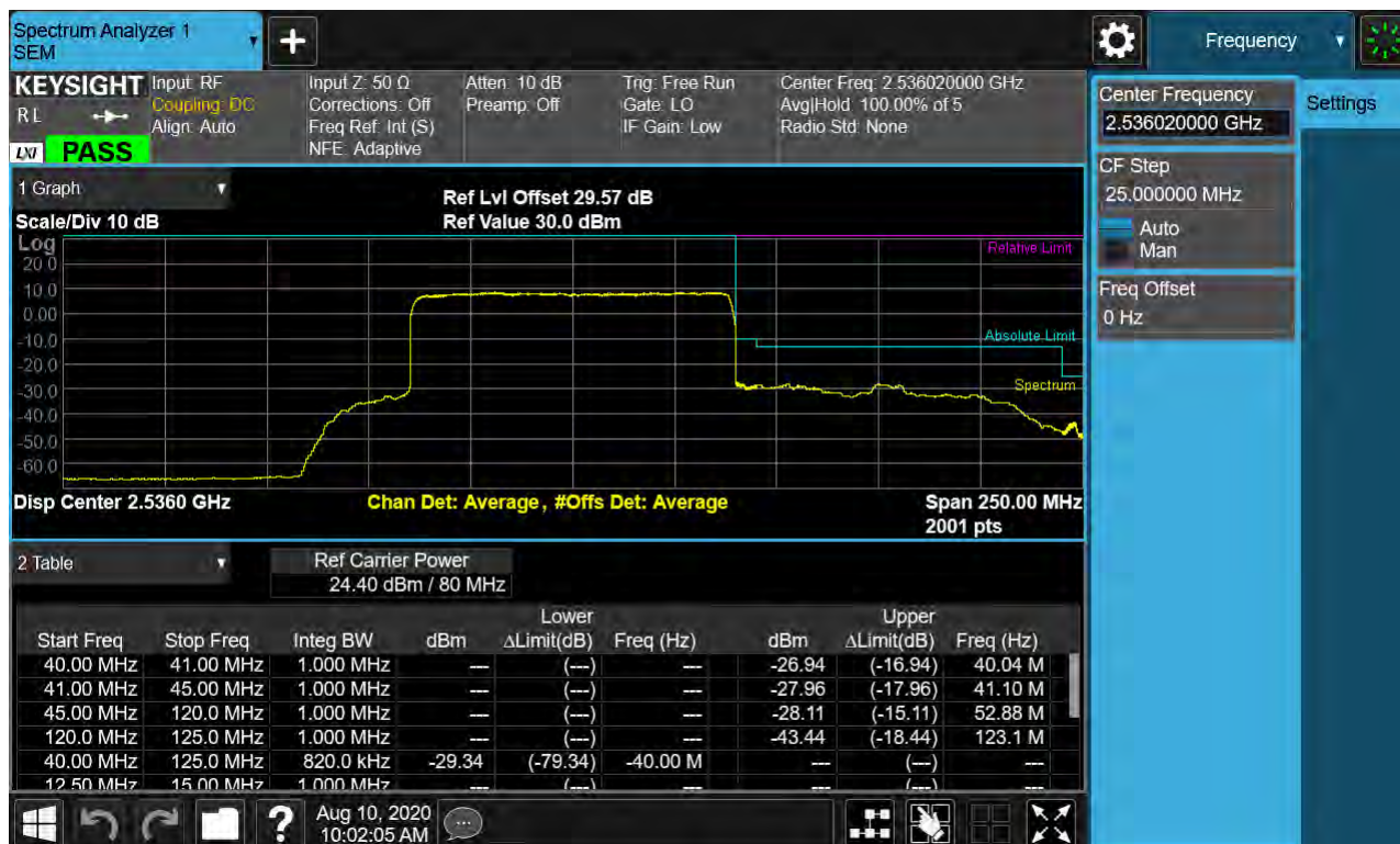
Sub6 n41. Low Channel Edge Plot (80 MHz Ch.507204 BPSK_RB25_Offset 0)-2
