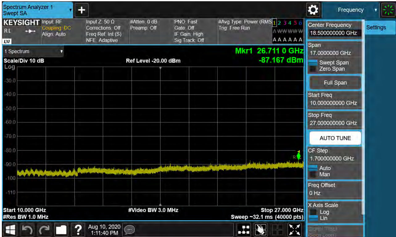
Sub6 n41. Conducted Spurious Plot 2 (100 MHz Ch. 518598 BPSK RB 1, Offset 0)
