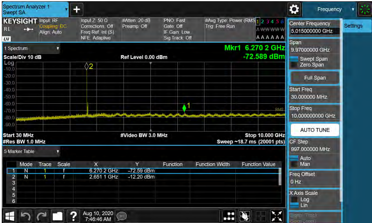
Sub6 n41. Conducted Spurious Plot 1 (40 MHz Ch.534000 BPSK RB 1, Offset 0)
