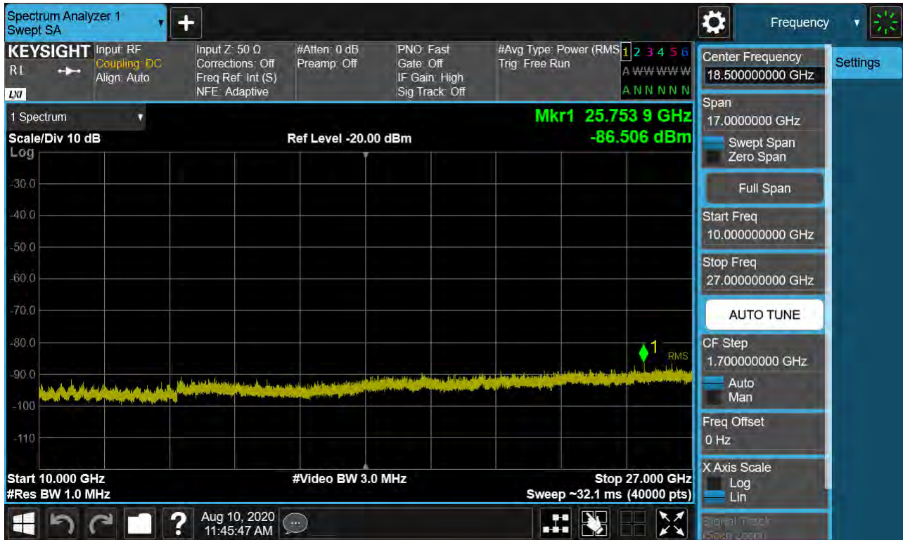
Sub6 n41. Conducted Spurious Plot 2 (90 MHz Ch. 518598 BPSK RB 1, Offset 0)
