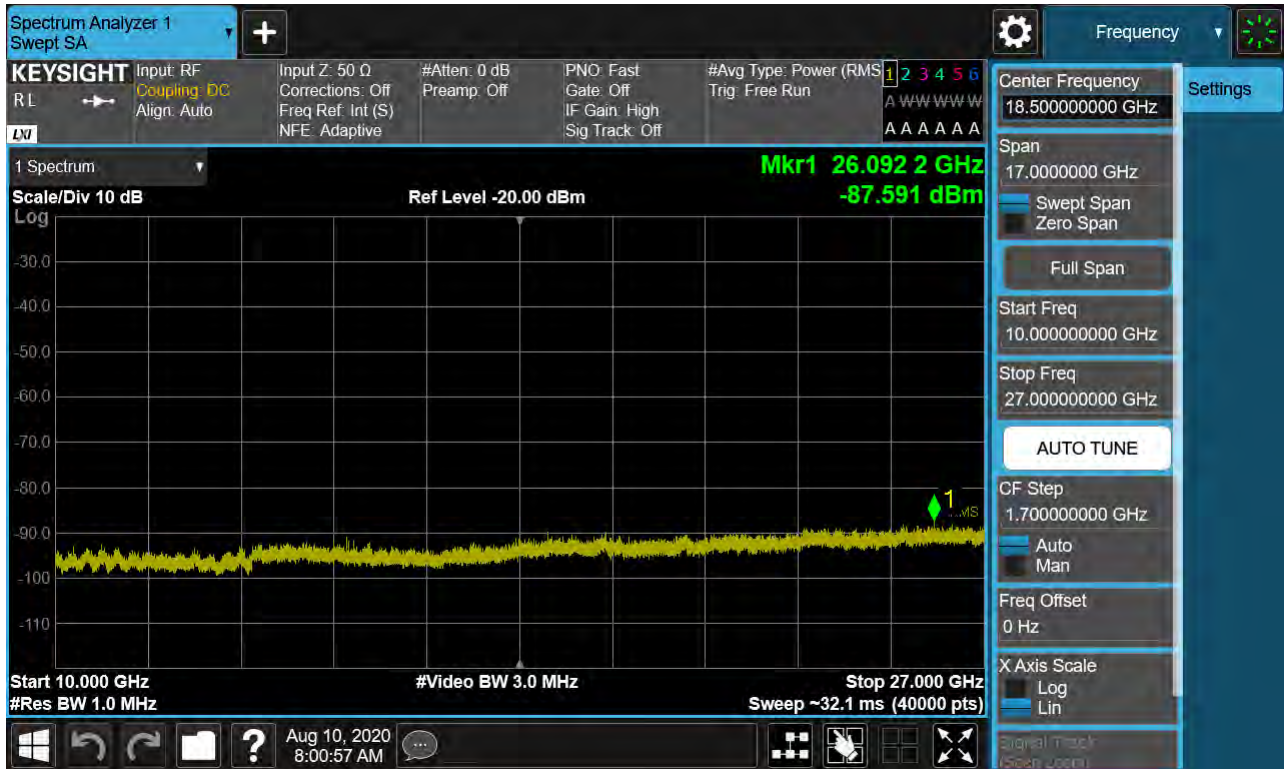
Sub6 n41. Conducted Spurious Plot 2 (50 MHz Ch.504204 BPSK RB 1, Offset 0)
