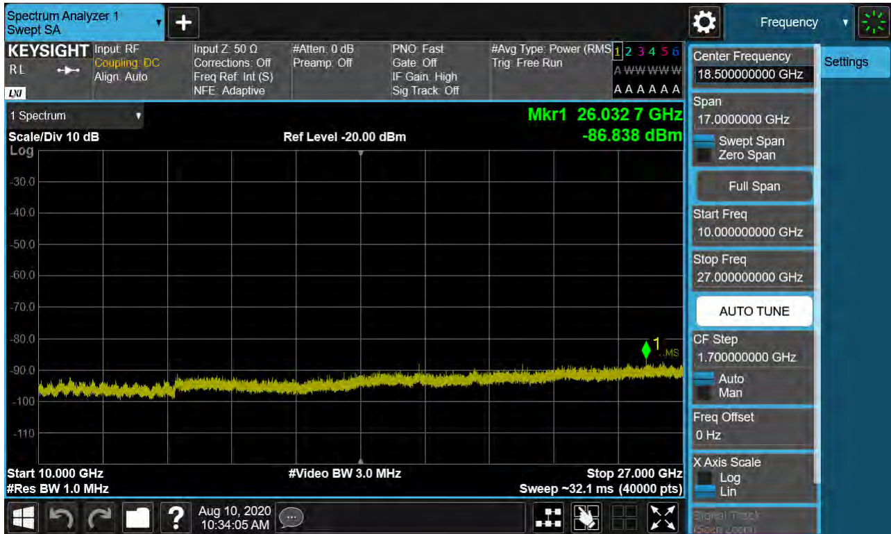
Sub6 n41. Conducted Spurious Plot 2 (80 MHz Ch.529998 BPSK RB 1, Offset 0)
