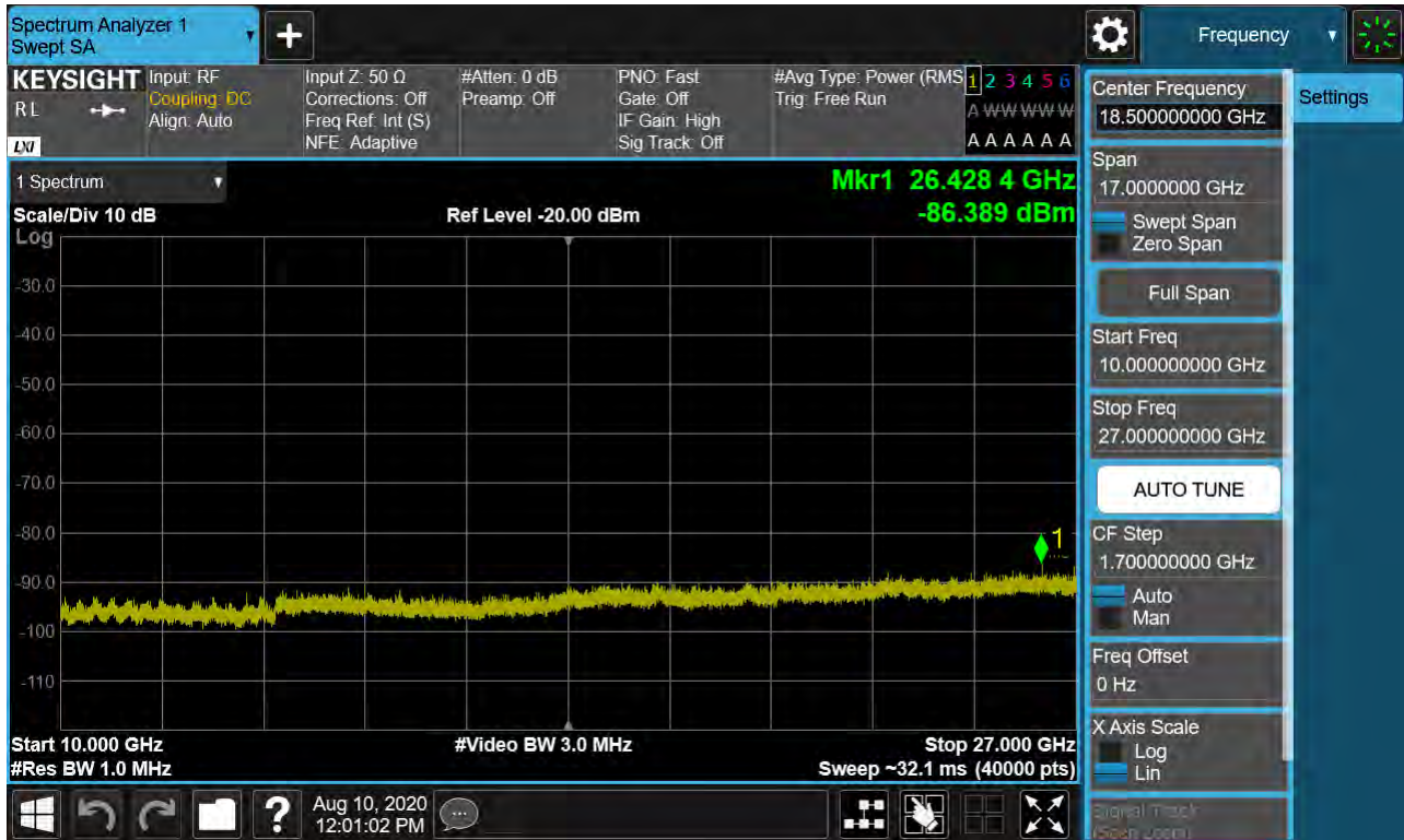
Sub6 n41. Conducted Spurious Plot 2 (90 MHz Ch.528996 BPSK RB 1, Offset 0)
