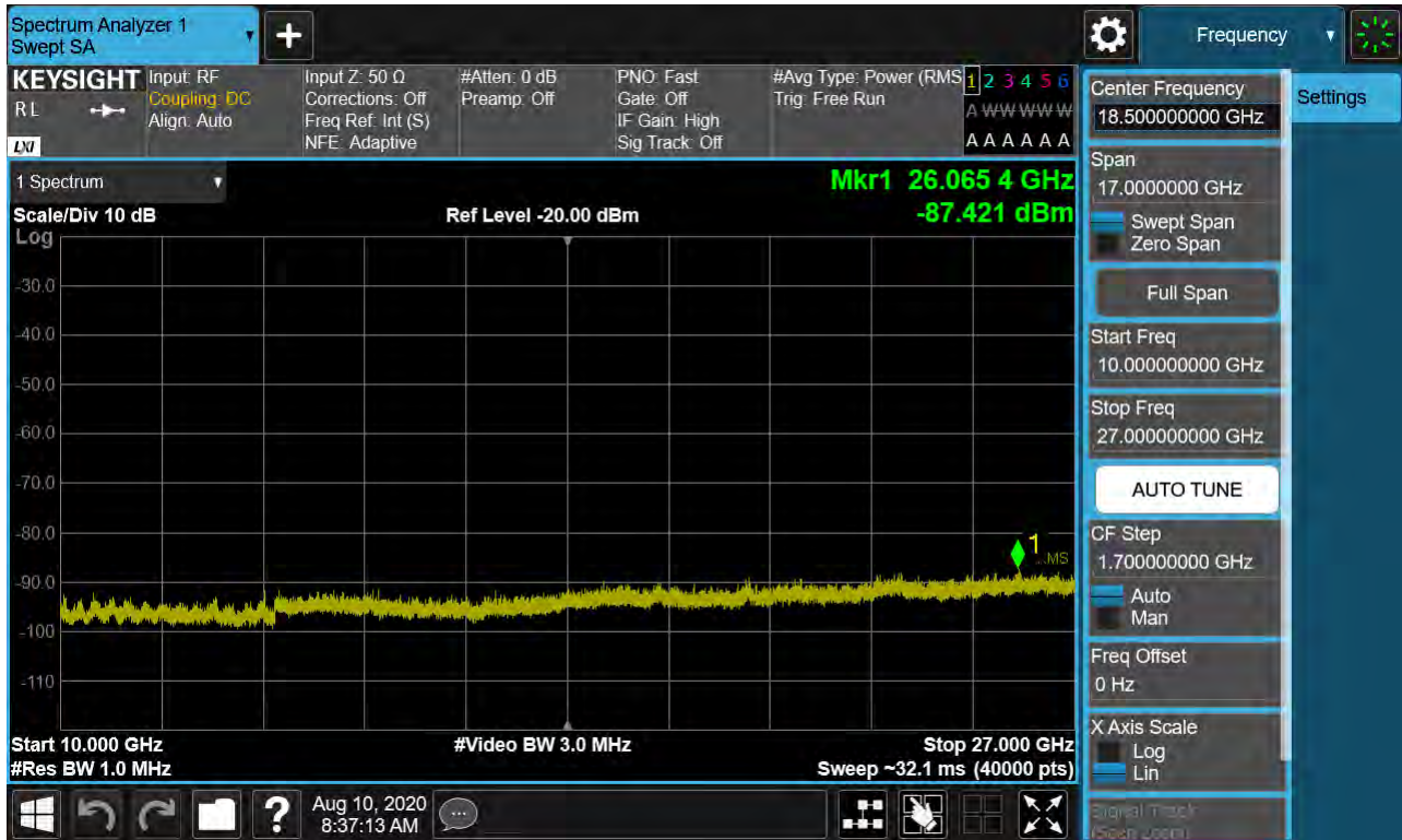
Sub6 n41. Conducted Spurious Plot 2 (60 MHz Ch.505200 BPSK RB 1, Offset 0)
