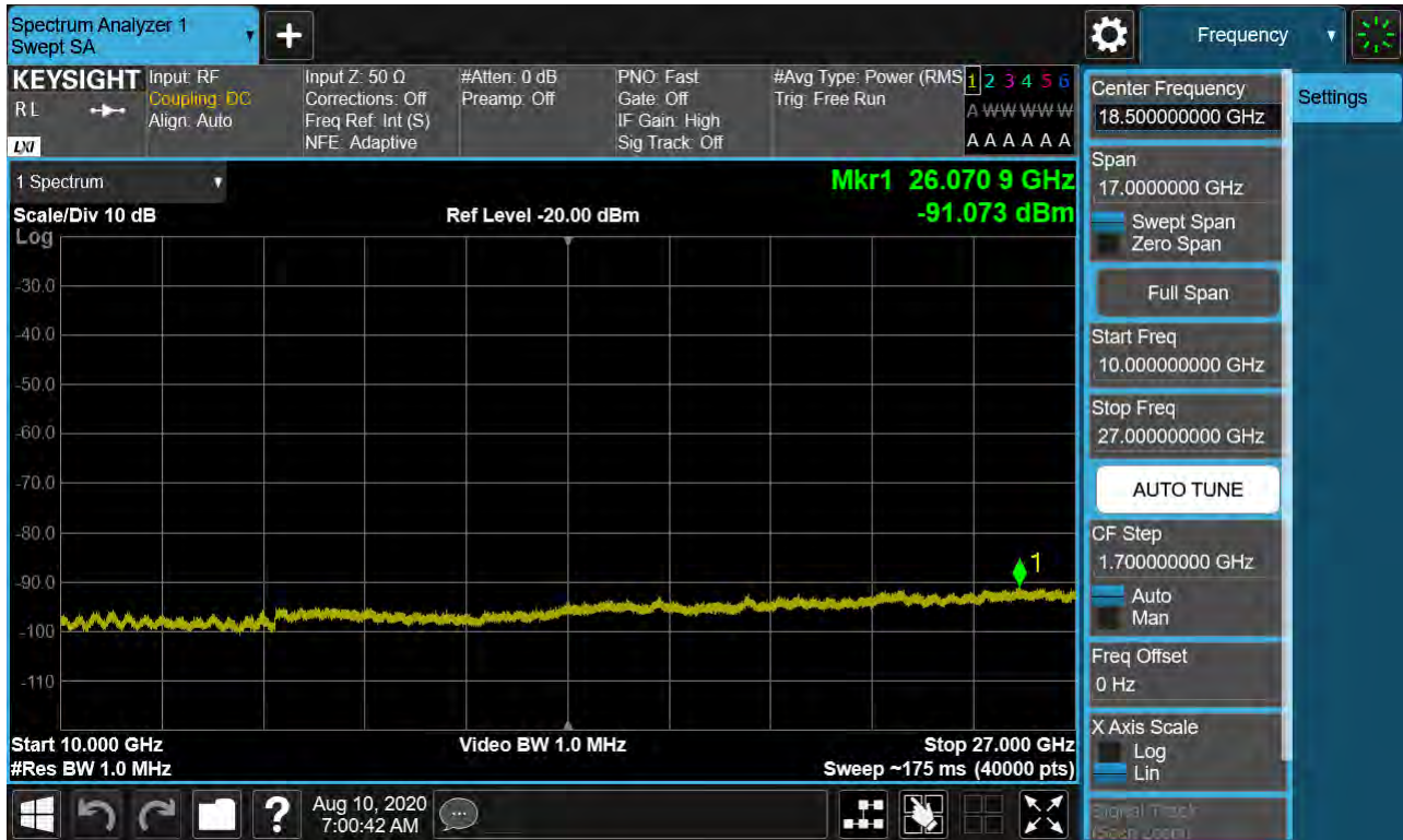
Sub6 n41. Conducted Spurious Plot 2 (20 MHz Ch.501204 BPSK RB 1, Offset 0)
