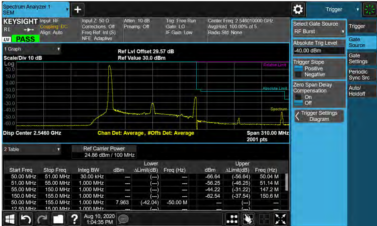
Sub6 n41. Low Channel Edge Plot (100 MHz Ch.509202 BPSK_RB1_Offset 0)-2
