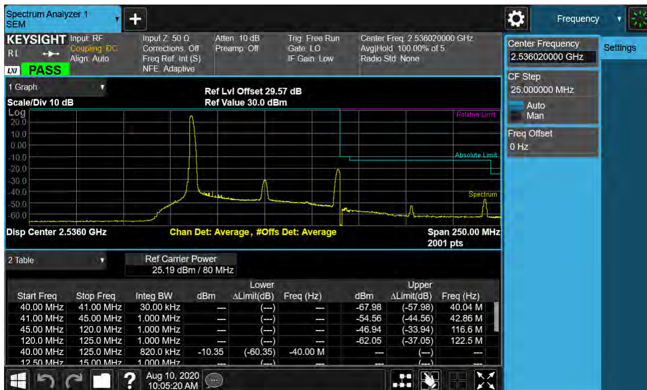
Sub6 n41. Low Channel Edge Plot (80 MHz Ch.507204 BPSK_RB1_Offset 0)-2
