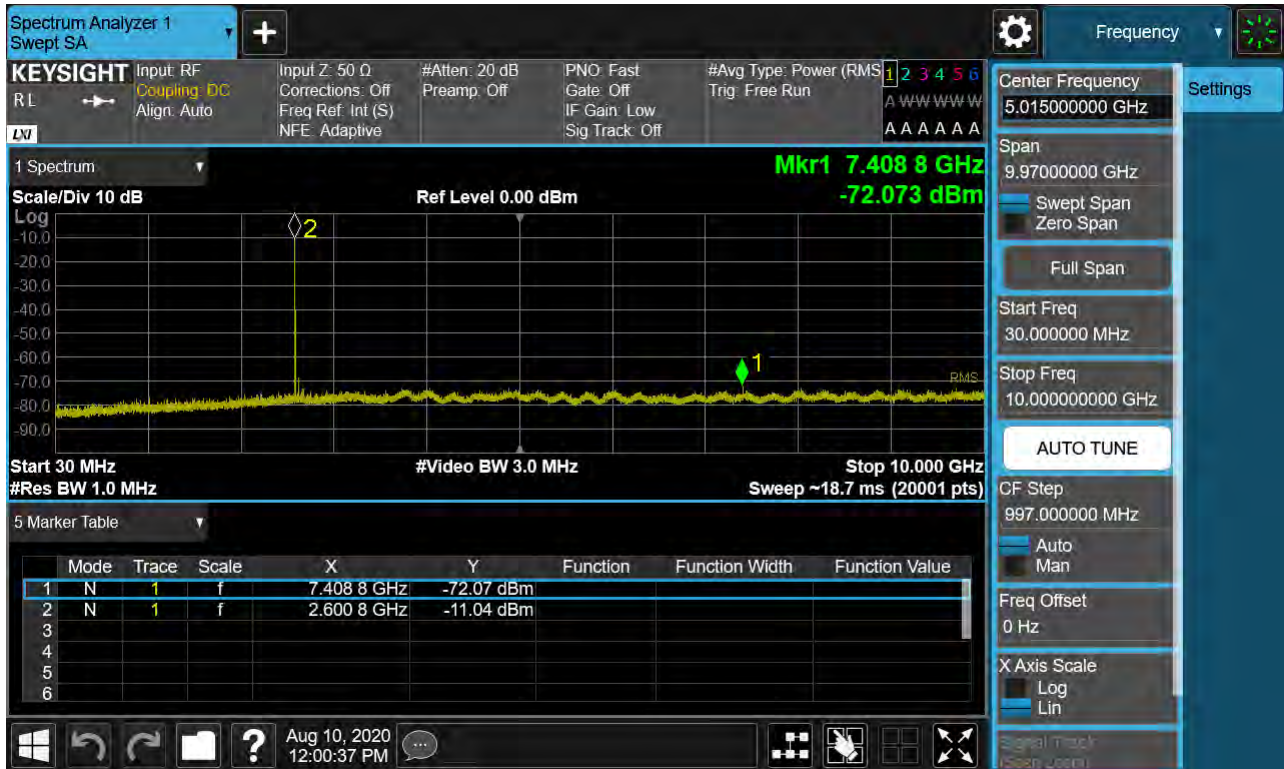
Sub6 n41. Conducted Spurious Plot 1 (90 MHz Ch.528996 BPSK RB 1, Offset 0)
