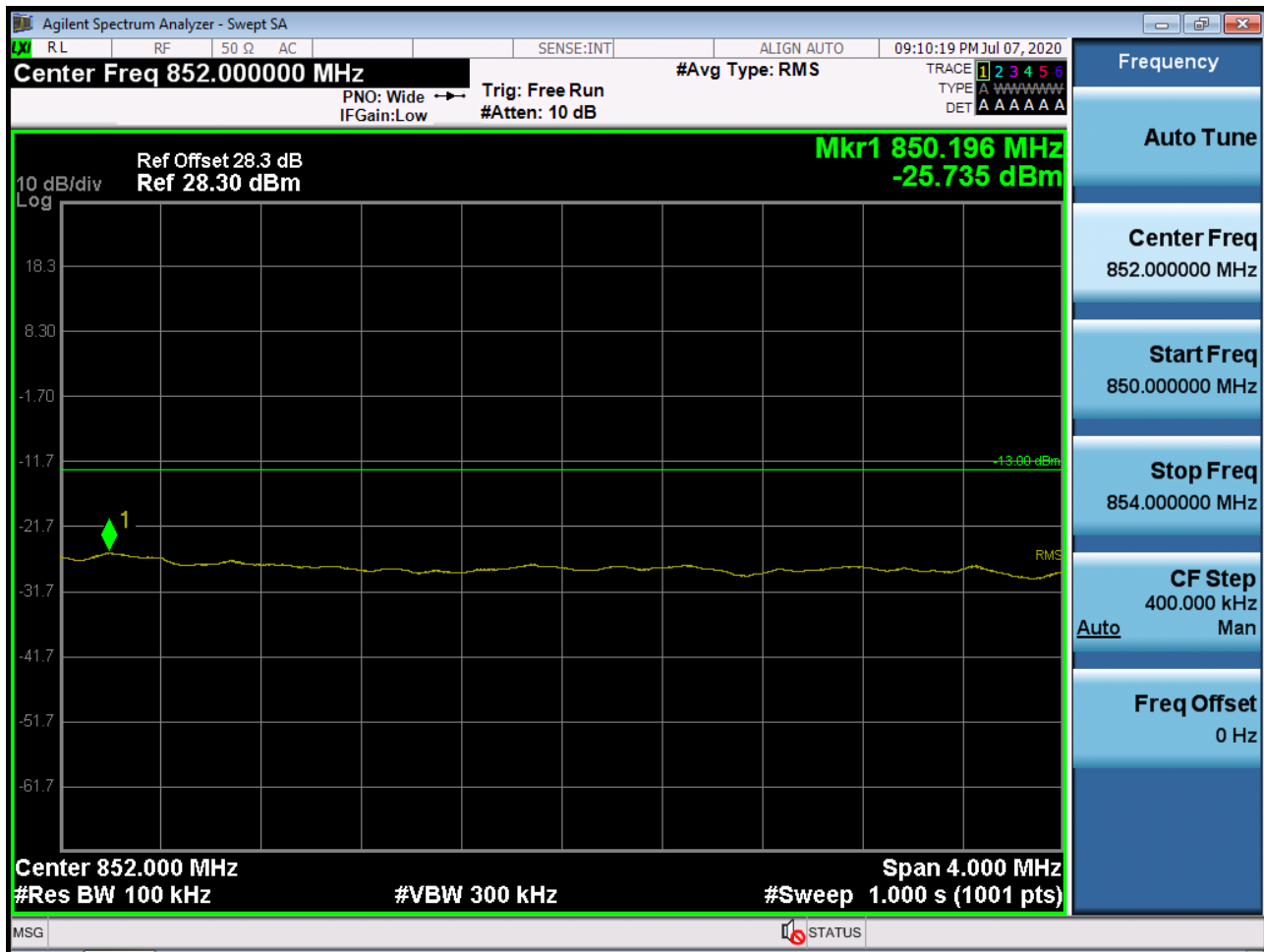
Sub6 n5. Upper Extended Band Edge Plot (15M BW Ch.168300 BPSK_RB75_0)
