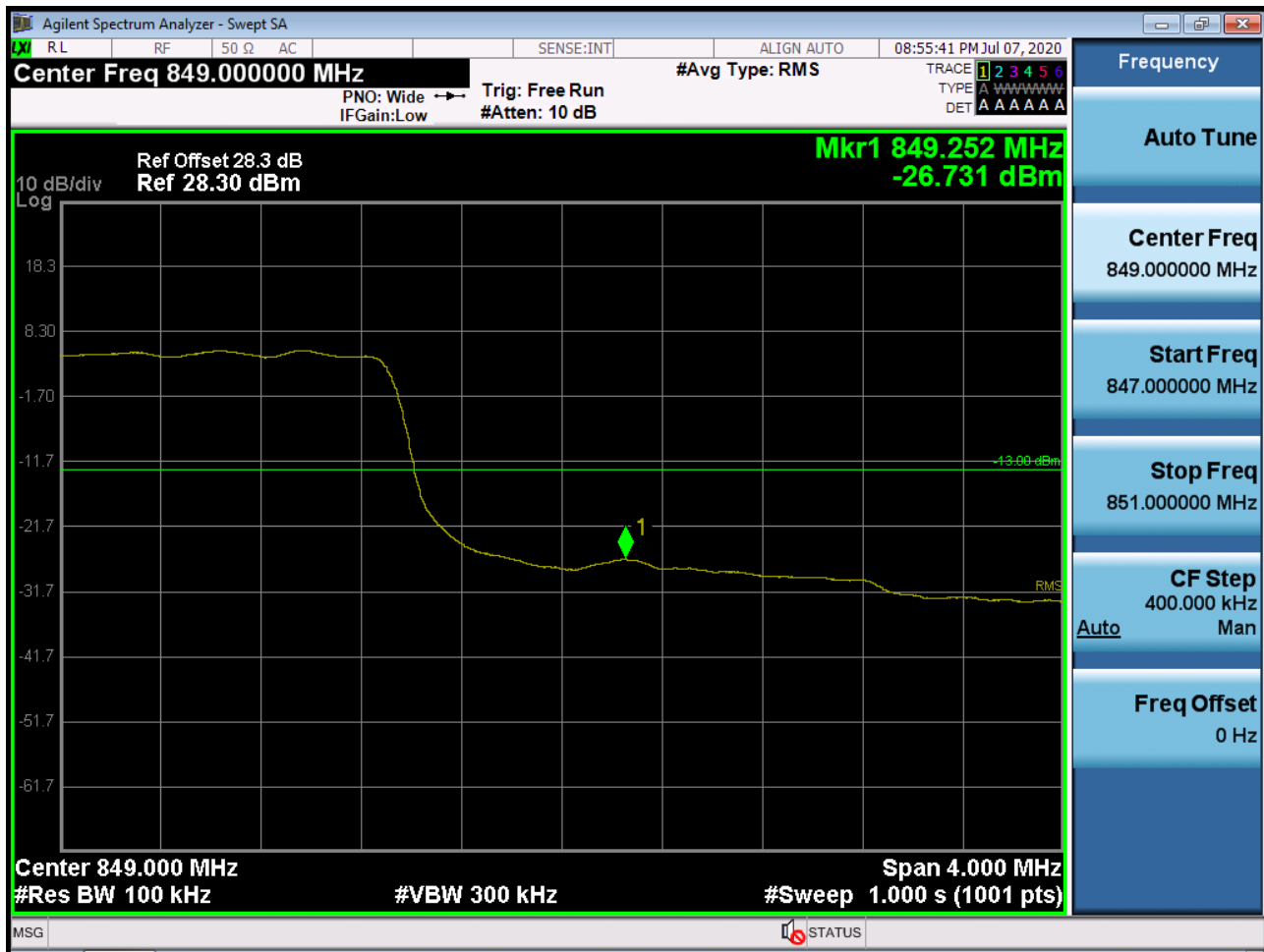
Sub6 n5. Upper Band Edge Plot (10M BW Ch.168800 BPSK_RB50_Offset 0)
