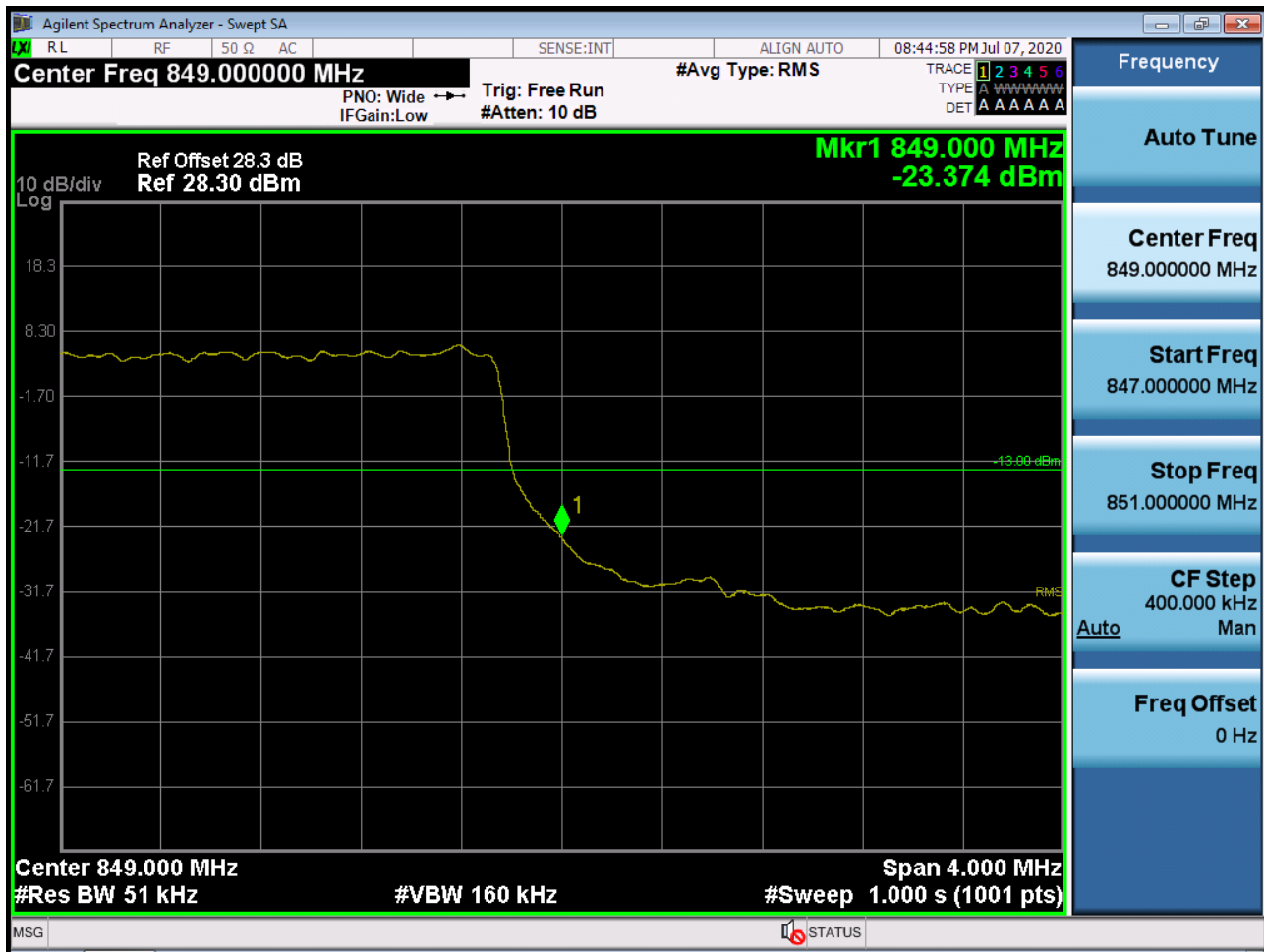
Sub6 n5. Upper Band Edge Plot (5M BW Ch.169300 BPSK_RB25_Offset 0)
