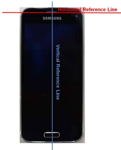
SAR Test Setup Photo 11 – Vertical and Horizontal Reference Lines
