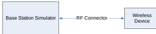
Figure 9-2 Power Measurement Setup
