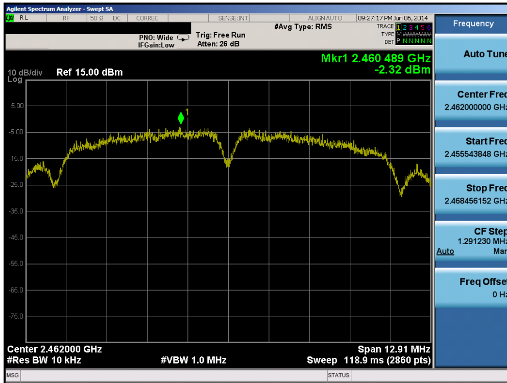
Plot 6-39. Power Spectral Density Plot (802.11b – Ch. 11)
