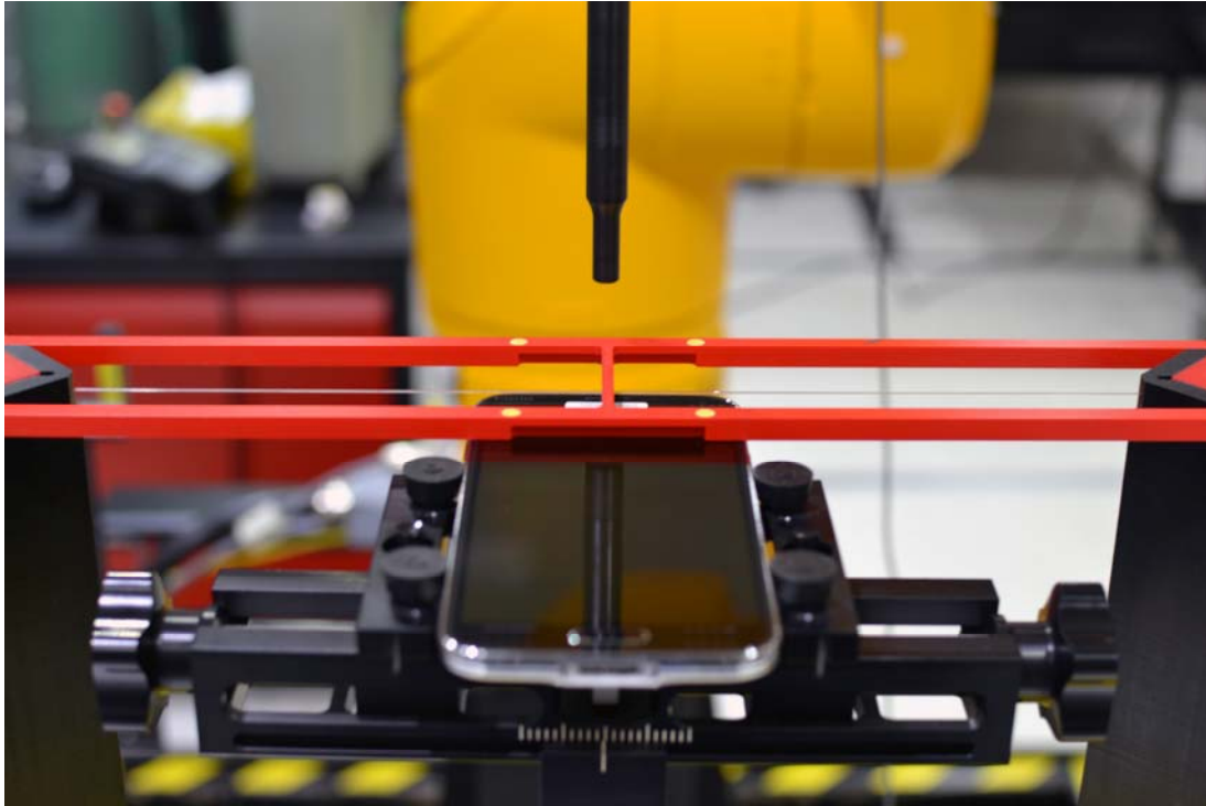
Figure 18-1 Ear Reference Point HAC Phantom Alignment
