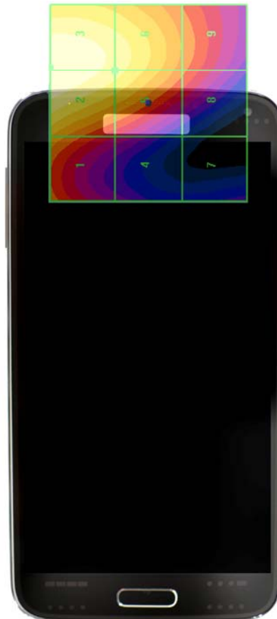
Figure 18-4 E-Field WD Scan overlay
