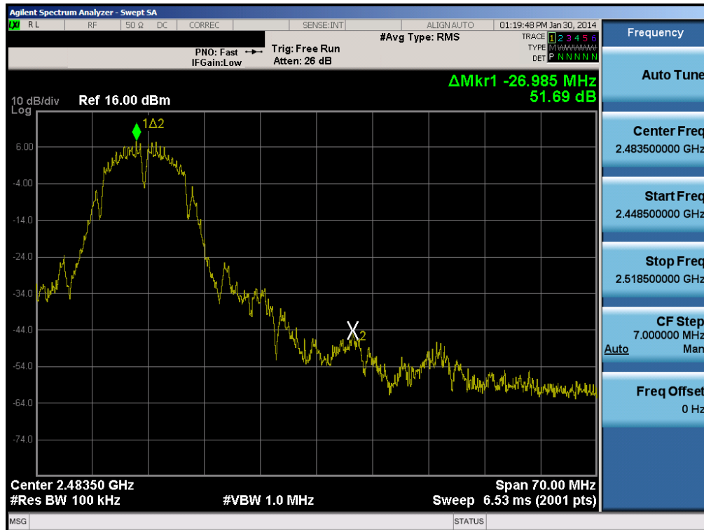
Plot 6-88. Band Edge Plot (802.11b – Ch. 11)
