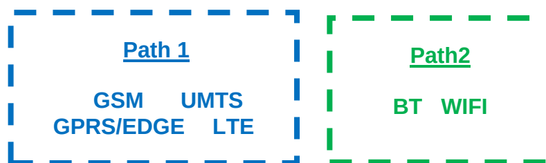
Figure 1-1 Simultaneous Transmission Paths
