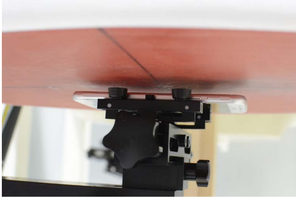
SAR Test Setup Photo 5: Back at 1.0 cm
