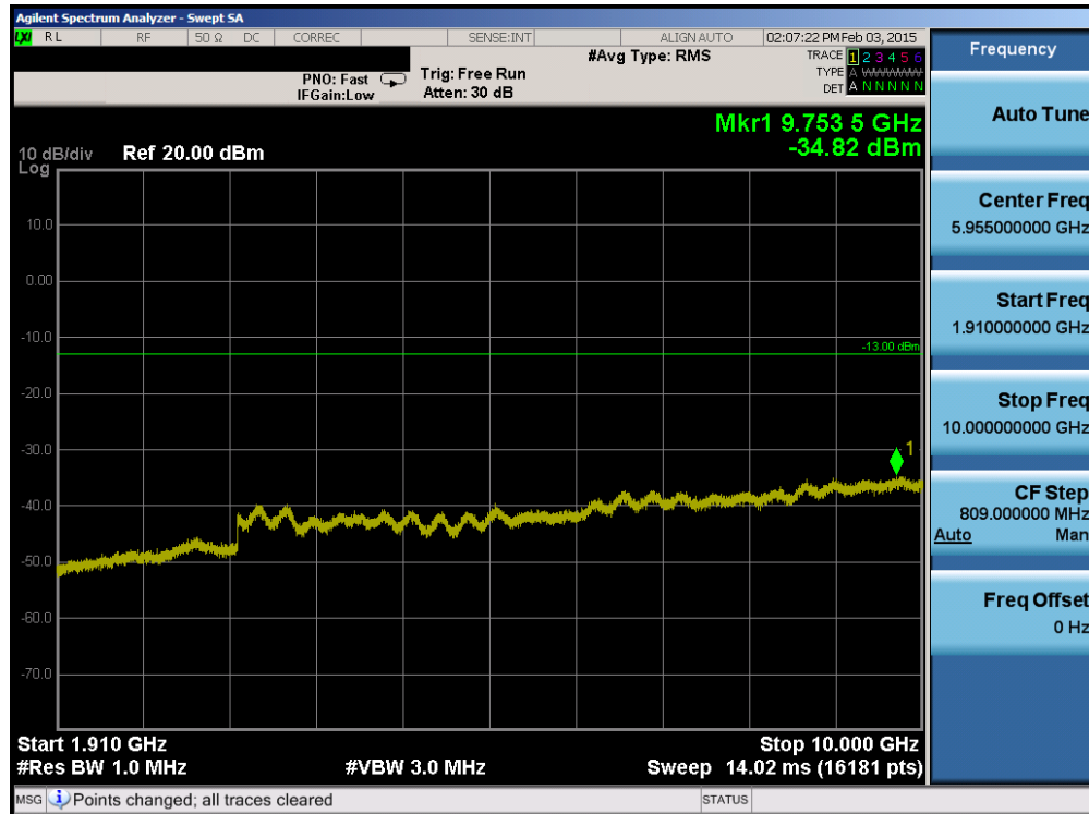
Plot 6-45. Conducted Spurious Plot (PCS WCDMA Mode – Ch. 9262)
