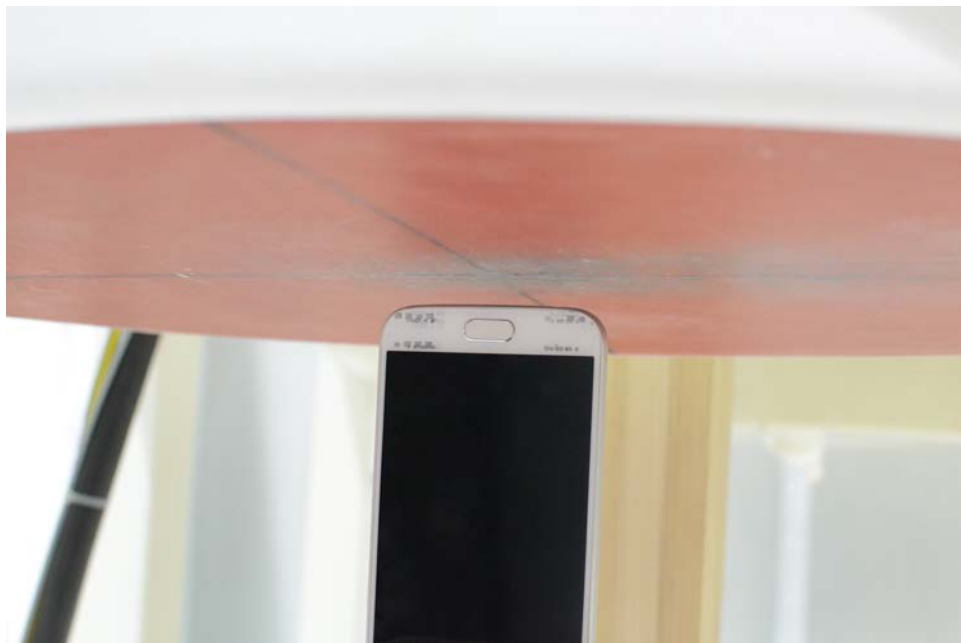
SAR Test Setup Photo 8: Bottom at 1.0 cm
