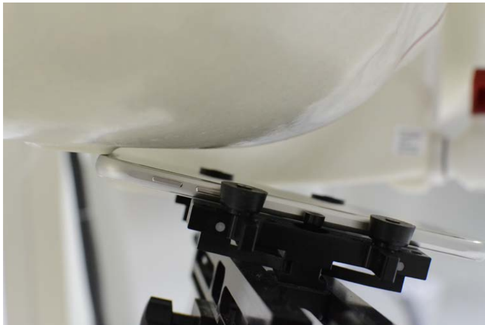
SAR Test Setup Photo 2: Right Tilt
