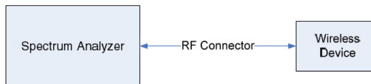
Figure 6-1. Test Instrument & Measurement Setup
