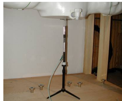
Figure 10-2 System Verification Setup Photo
