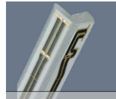
Figure 4-1 E-field Free-space Probe
