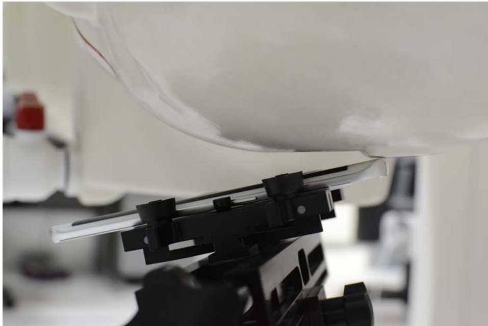
SAR Test Setup Photo 4: Left Tilt
