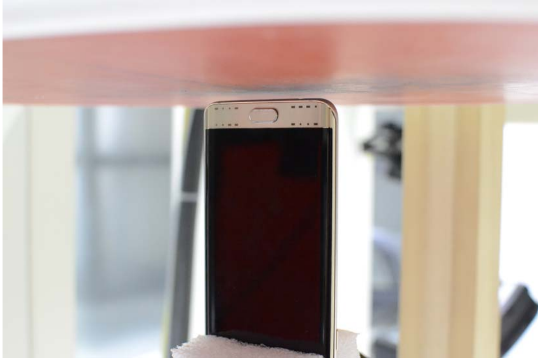
SAR Test Setup Photo 15 – Bottom Edge at 0.4 cm (Extremity)
