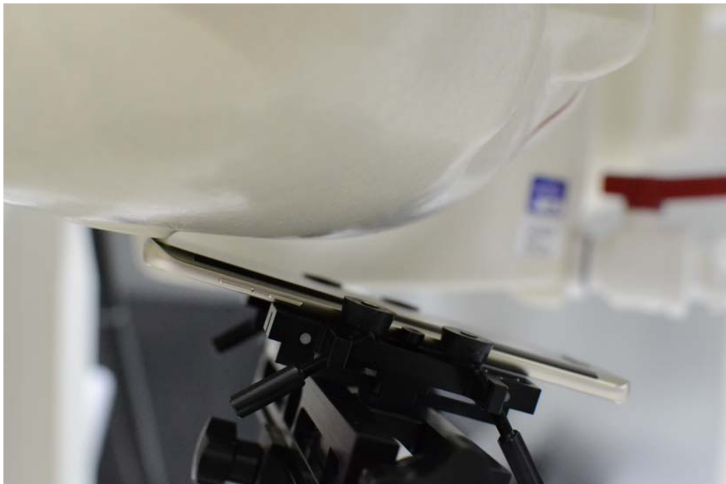
SAR Test Setup Photo 2- Right Tilt
