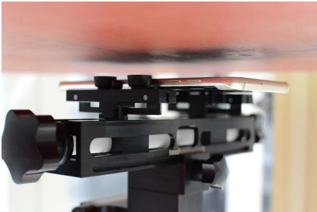
SAR Test Setup Photo 8– Back Side at 1.5 cm (Body-Worn)
