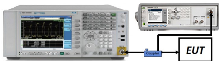
Figure 7-1. Test Instrument & Measurement Setup
