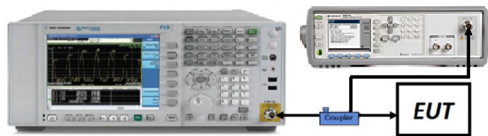
Figure 7-5. Test Instrument & Measurement Setup
