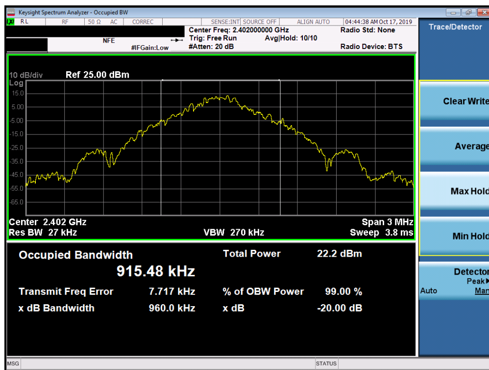
Plot 7-1. 20dB Bandwidth Plot (Bluetooth, 1Mbps – Ch. 0)
