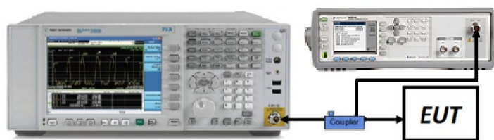
Figure 7-3. Test Instrument & Measurement Setup
