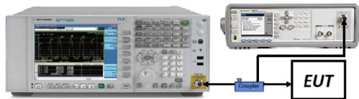
Figure 7-4. Test Instrument & Measurement Setup
