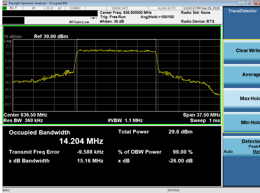
Plot 7-33. Occupied Bandwidth Plot (NR Band n5 - 15MHz 64-QAM - Full RB Configuration)
