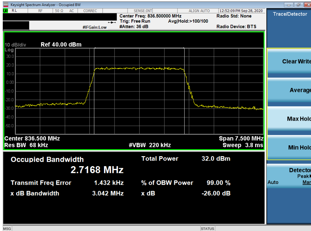
Plot 7-18. Occupied Bandwidth Plot (LTE Band 26/5 - 3MHz 16-QAM - Full RB Configuration)
