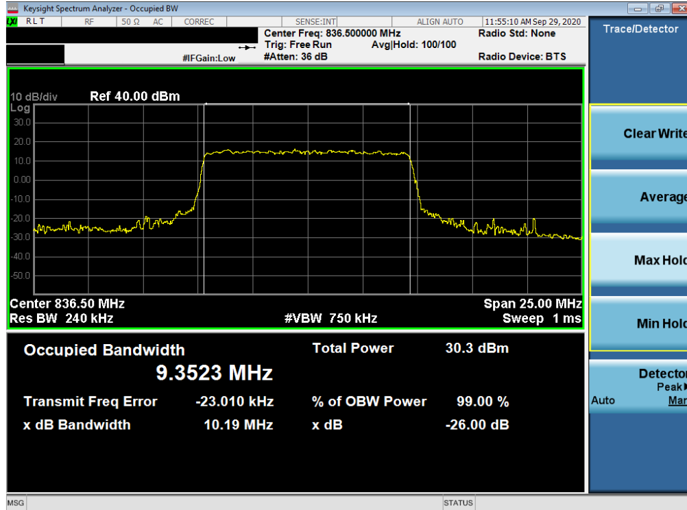
Plot 7-37. Occupied Bandwidth Plot (NR Band n5 - 10MHz 16-QAM - Full RB Configuration)
