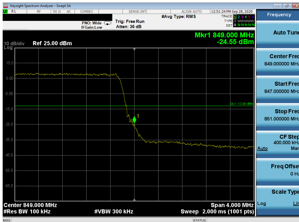
Plot 7-103. Upper Band Edge Plot (LTE Band 26/5 - 5MHz QPSK - Full RB Configuration)
