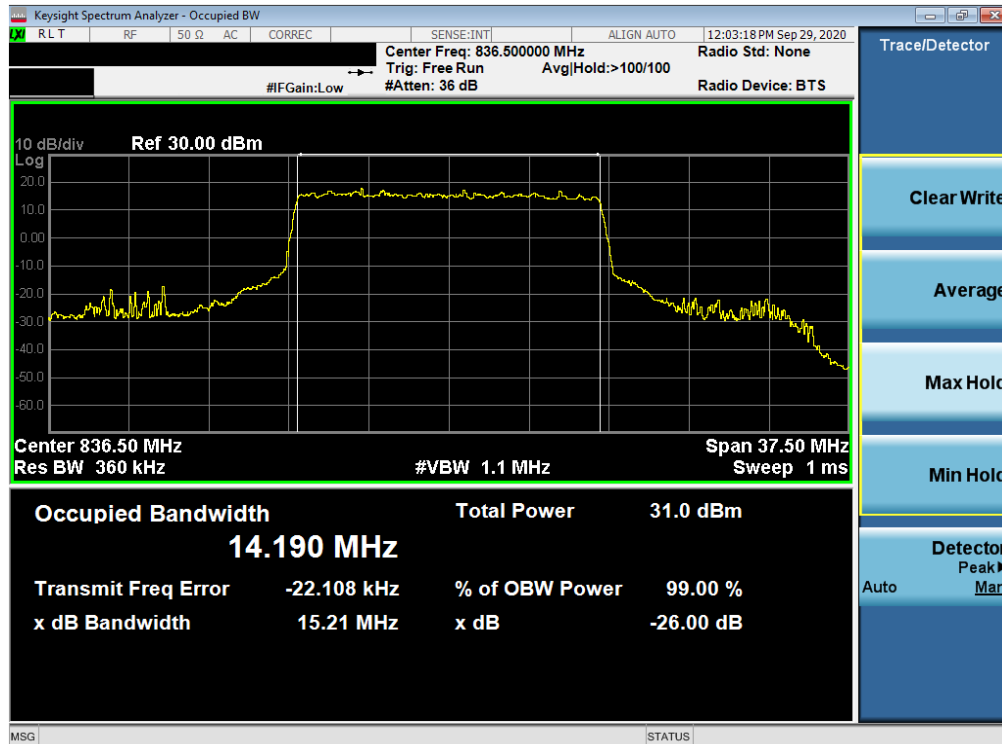
Plot 7-32. Occupied Bandwidth Plot (NR Band n5 - 15MHz 16-QAM - Full RB Configuration)
