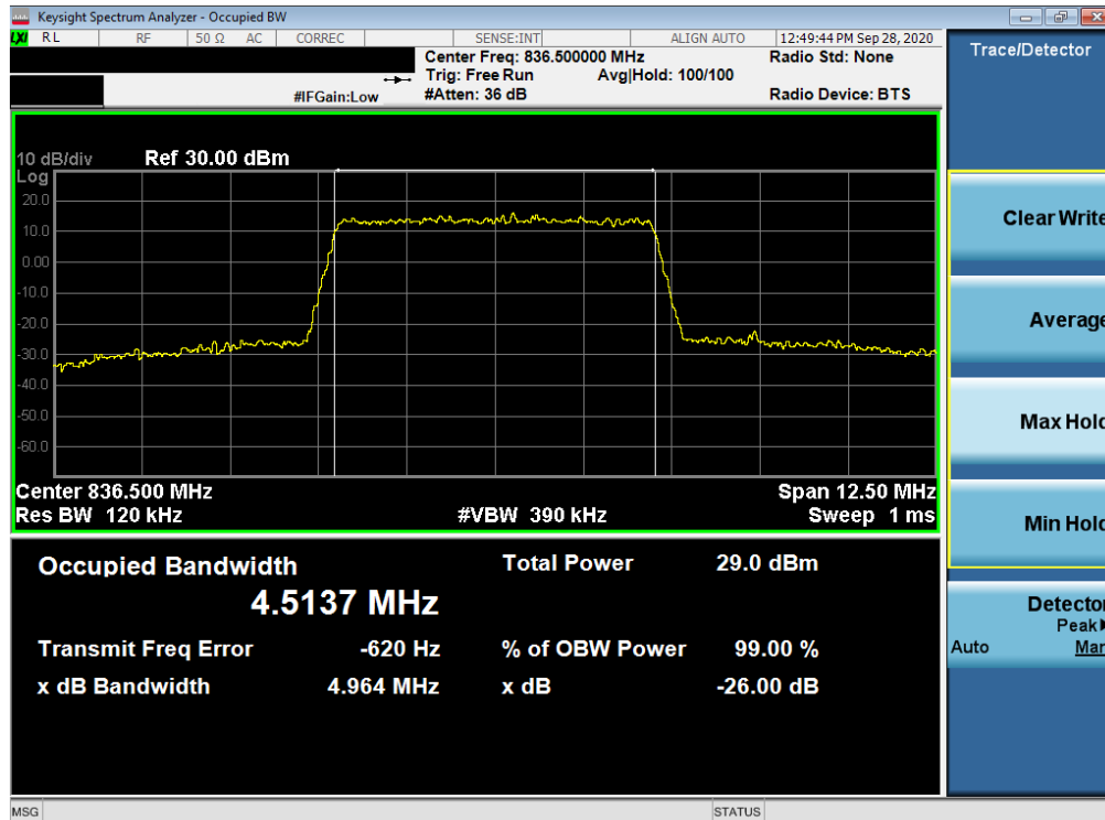
Plot 7-16. Occupied Bandwidth Plot (LTE Band 26/5 - 5MHz 256-QAM - Full RB Configuration)
