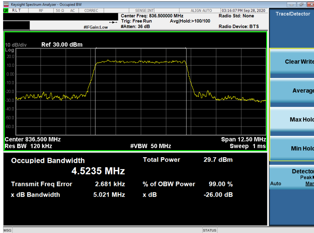
Plot 7-43. Occupied Bandwidth Plot (NR Band n5 - 5MHz 64-QAM - Full RB Configuration)
