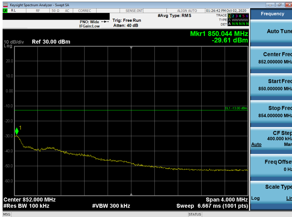
Plot 7-97. Upper Extended Band Edge Plot (CDMA Cell – Ch. 777)
