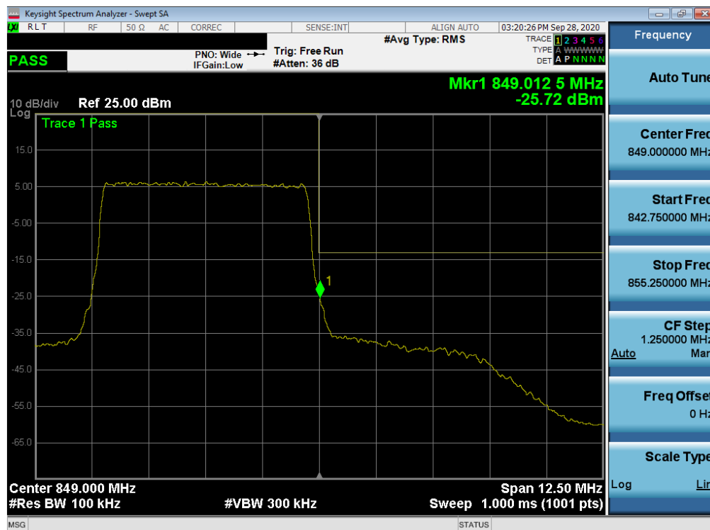
Plot 7-115. Upper Band Edge Plot (NR Band n5 – 5.0MHz - Full RB)
