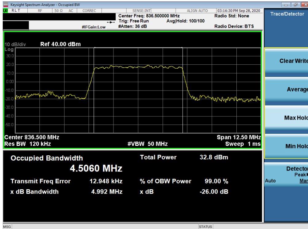
Plot 7-40. Occupied Bandwidth Plot (NR Band n5 - 5MHz \pi/2 BPSK - Full RB Configuration)
