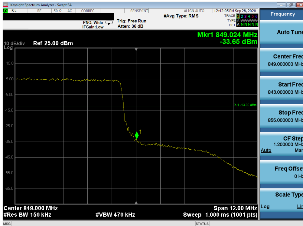
Plot 7-99. Upper Band Edge Plot (LTE Band 26 - 15MHz QPSK – Full RB Configuration)
