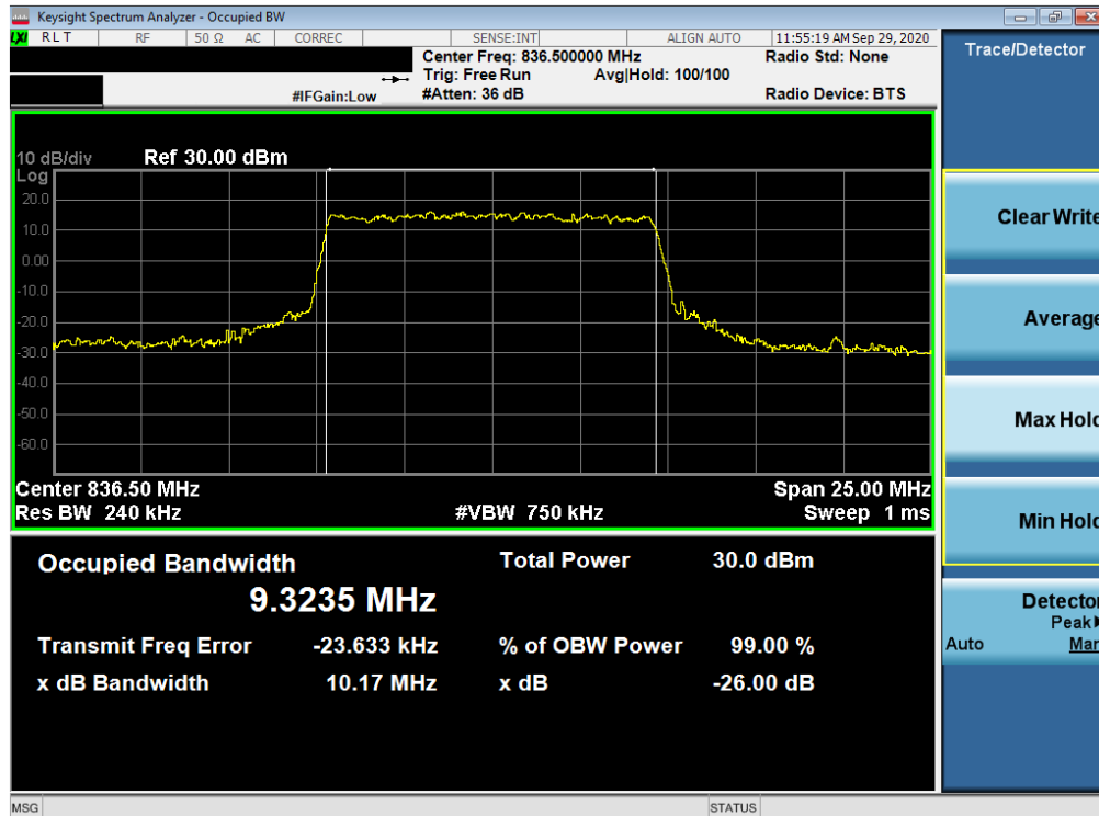
Plot 7-38. Occupied Bandwidth Plot (NR Band n5 - 10MHz 64-QAM - Full RB Configuration)
