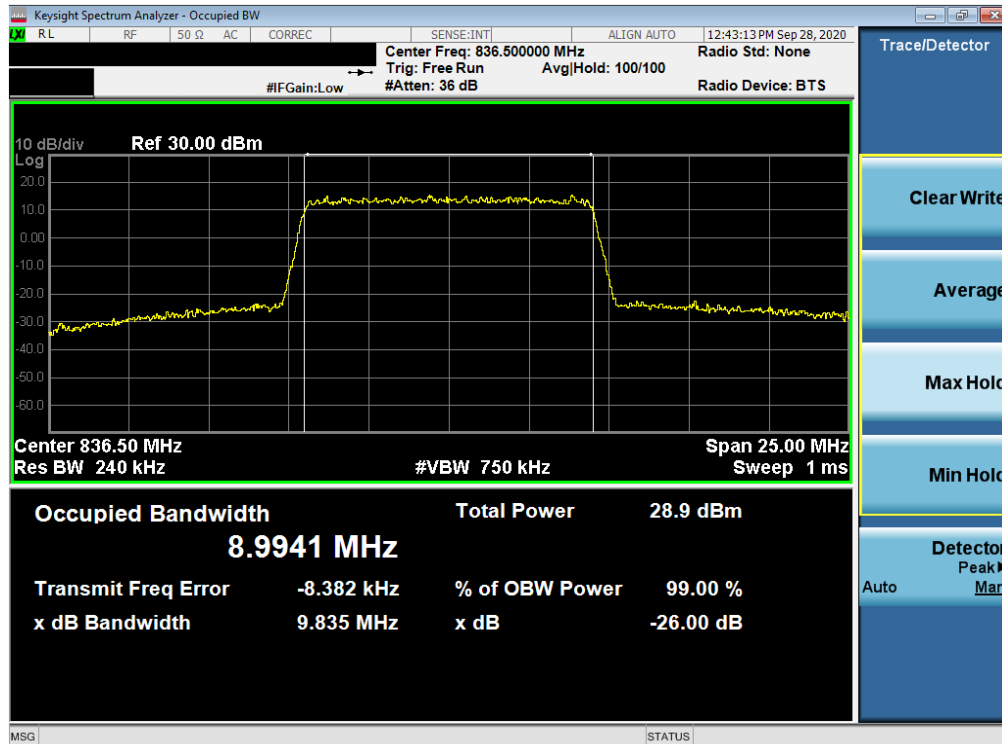
Plot 7-12. Occupied Bandwidth Plot (LTE Band 26/5 - 10MHz 256-QAM - Full RB Configuration)
