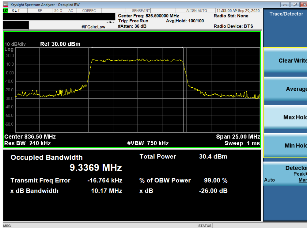
Plot 7-36. Occupied Bandwidth Plot (NR Band n5 - 10MHz QPSK - Full RB Configuration)
