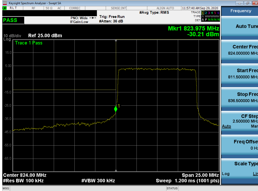
Plot 7-112. Lower Band Edge Plot (NR Band n5 - 10.0MHz - Full RB)
