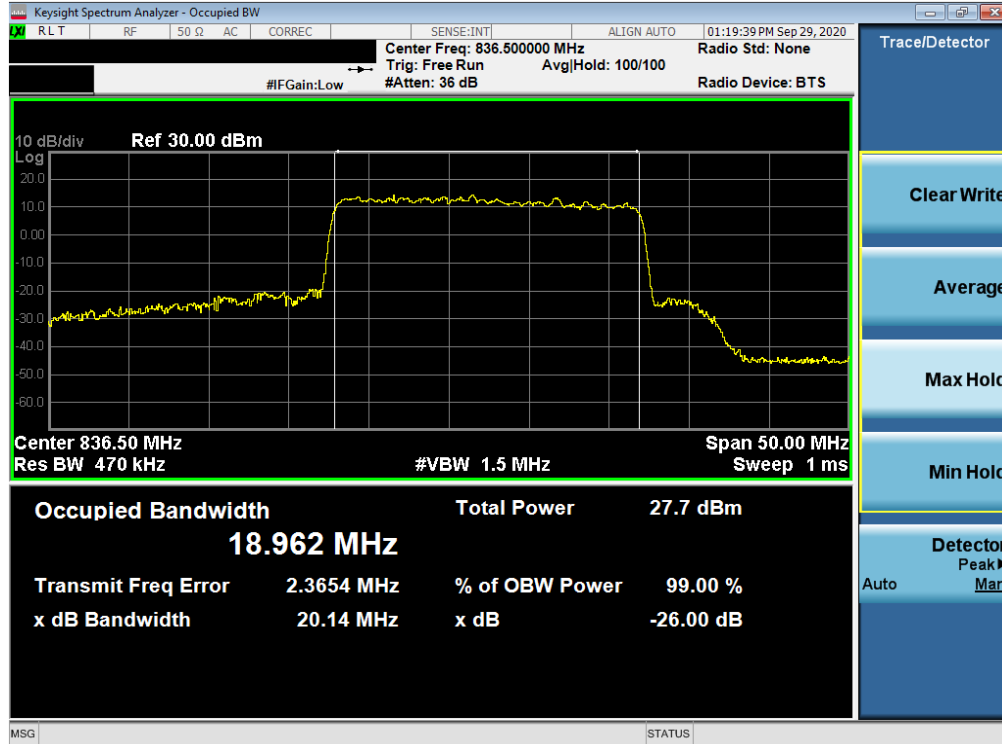
Plot 7-29. Occupied Bandwidth Plot (NR Band n5 - 20MHz 256-QAM - Full RB Configuration)
