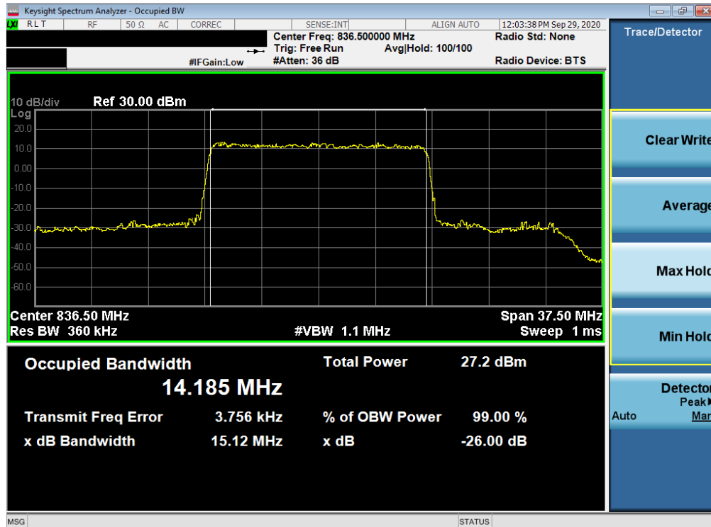
Plot 7-34. Occupied Bandwidth Plot (NR Band n5 - 15MHz 256-QAM - Full RB Configuration)
