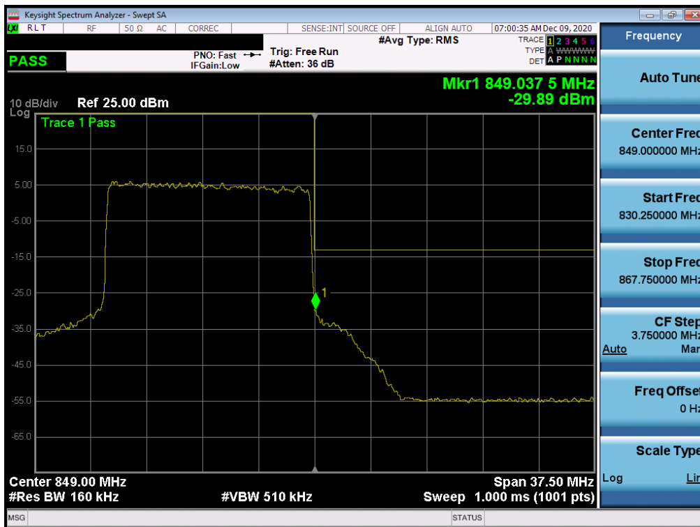
Plot 7-111. Upper Band Edge Plot (NR Band n5 - 15.0MHz - Full RB)
