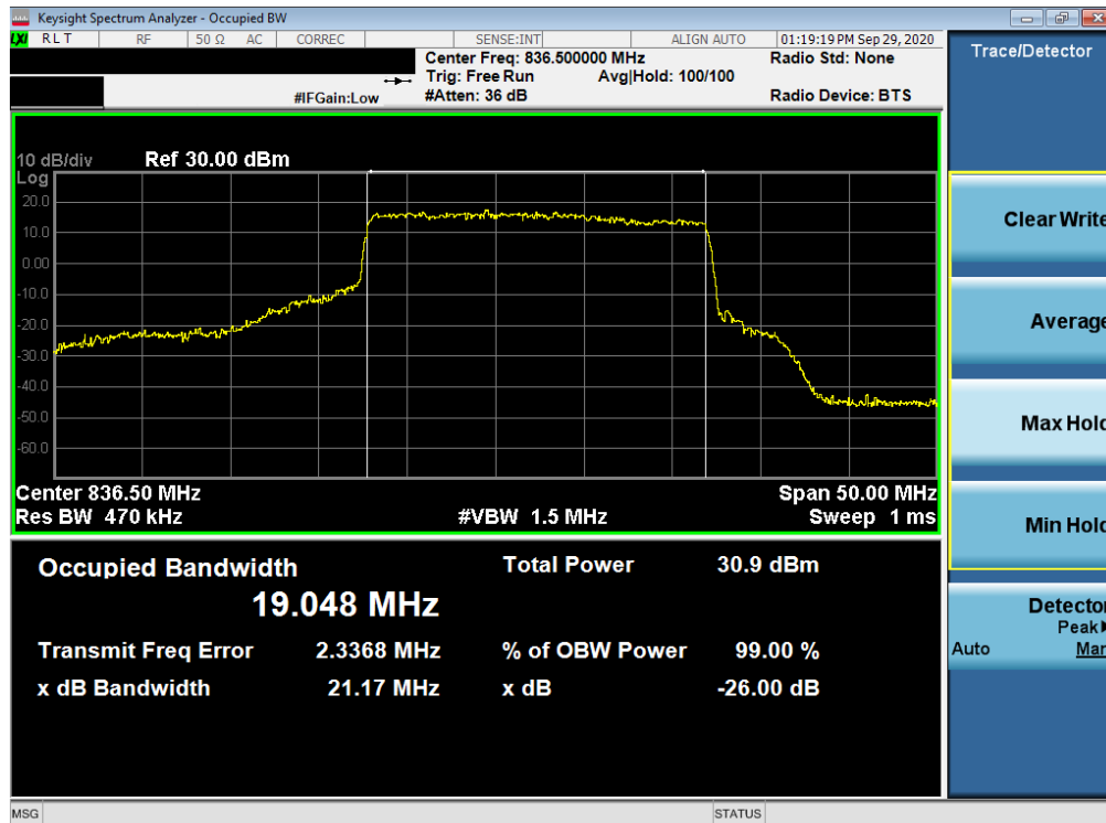
Plot 7-27. Occupied Bandwidth Plot (NR Band n5 - 20MHz 16-QAM - Full RB Configuration)
