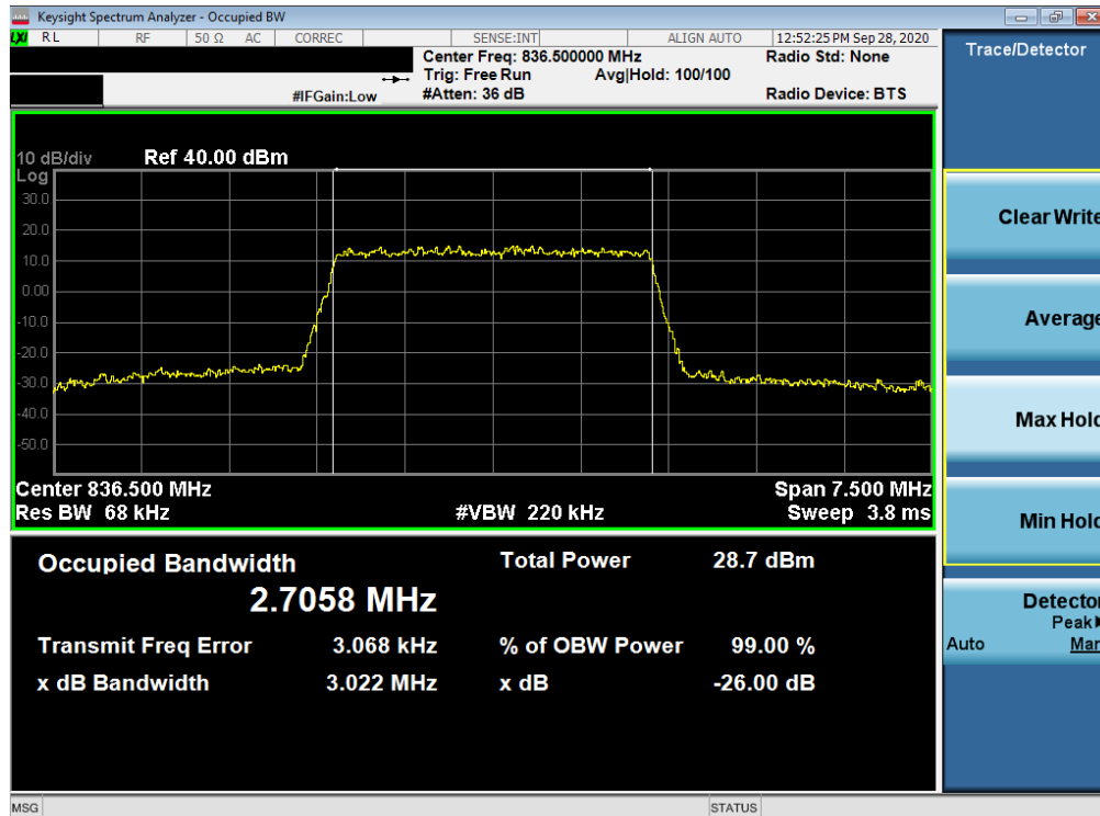
Plot 7-20. Occupied Bandwidth Plot (LTE Band 26/5 - 3MHz 256-QAM - Full RB Configuration)
