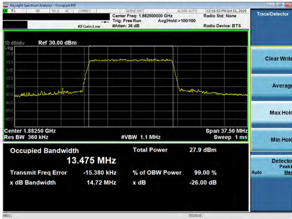
Plot 7-12. Occupied Bandwidth Plot (LTE Band 25/2 - 15MHz 256-QAM - Full RB Configuration)
