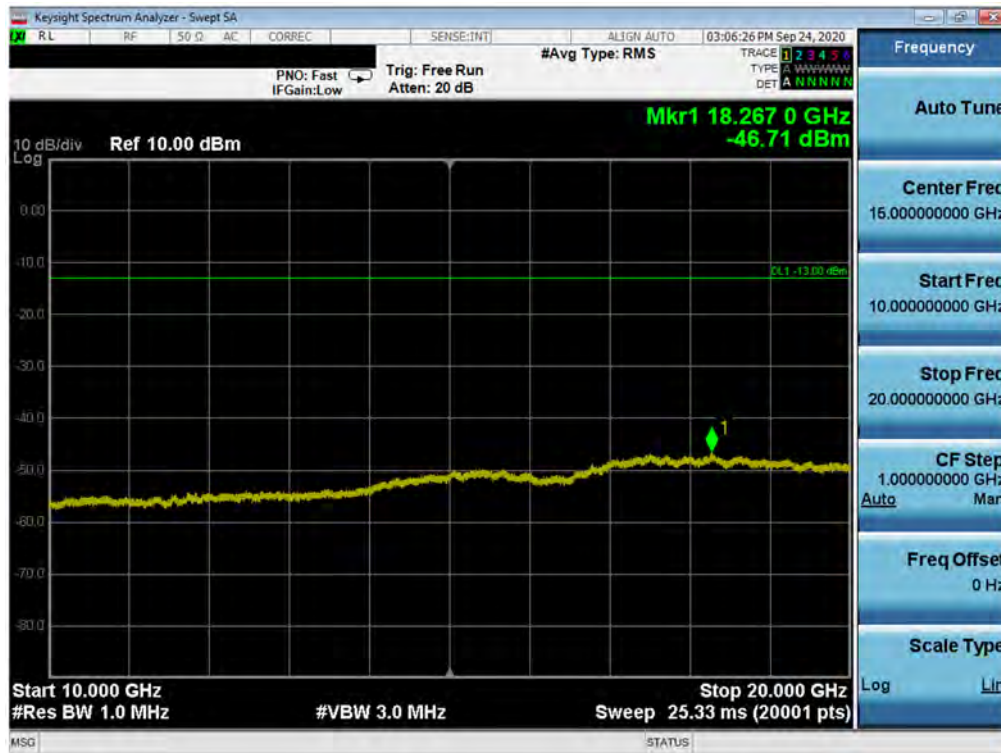
Plot 7-31. Conducted Spurious Plot (WCDMA Ch. 9400)
