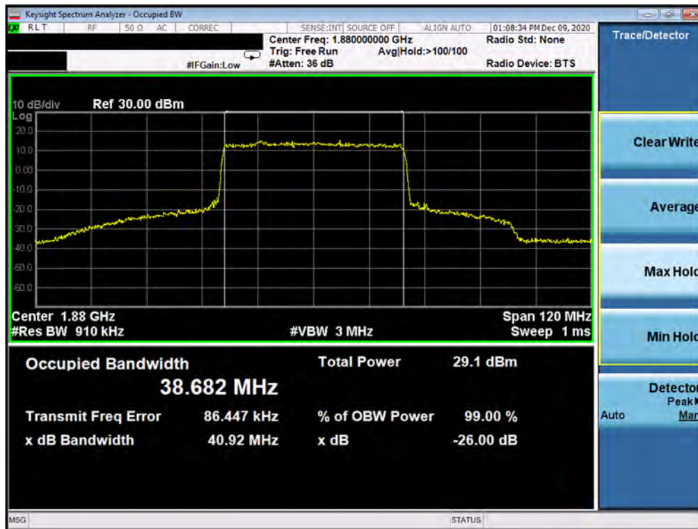
Plot 7-32. Occupied Bandwidth Plot (NR Band n25 - 40.0MHz CP-OFDM 64QAM - Full RB)
