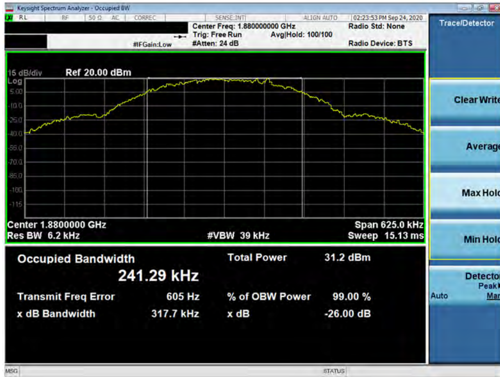
Plot 7-1. Occupied Bandwidth Plot (GPRS, Ch. 661)
