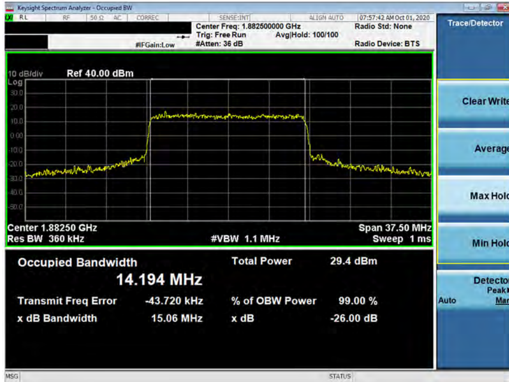
Plot 7-52. Occupied Bandwidth Plot (NR Band n25/2 - 15.0MHz CP-OFDM 64QAM - Full RB)
