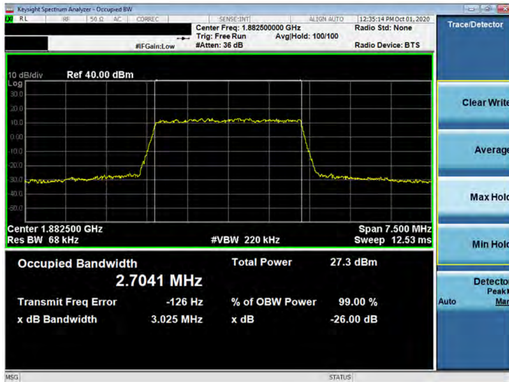
Plot 7-24. Occupied Bandwidth Plot (LTE Band 25/2 - 3MHz 256-QAM - Full RB Configuration)
