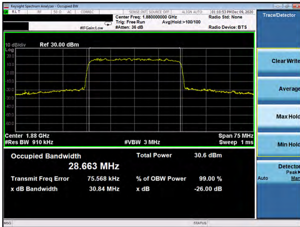
Plot 7-36. Occupied Bandwidth Plot (NR Band n25 - 30.0MHz CP-OFDM 16QAM - Full RB)
