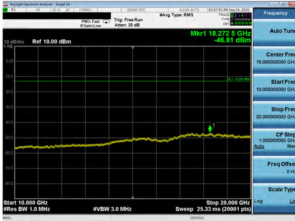
Plot 7-31. Conducted Spurious Plot (WCDMA Ch. 9262)
