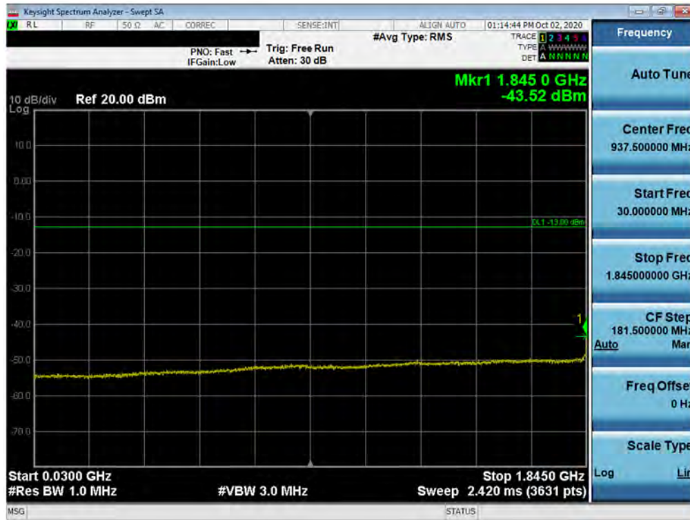
Plot 7-31. Conducted Spurious Plot (CDMA Ch. 25)
