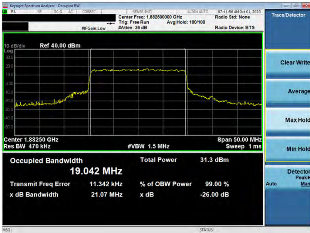
Plot 7-45. Occupied Bandwidth Plot (NR Band n25/2 - 20.0MHz CP-OFDM QPSK - Full RB)
