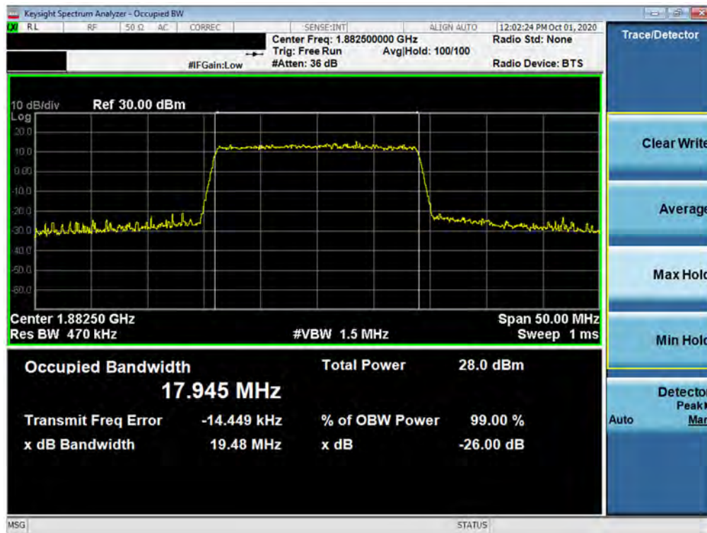
Plot 7-8. Occupied Bandwidth Plot (LTE Band 25/2 - 20MHz 256-QAM - Full RB Configuration)
