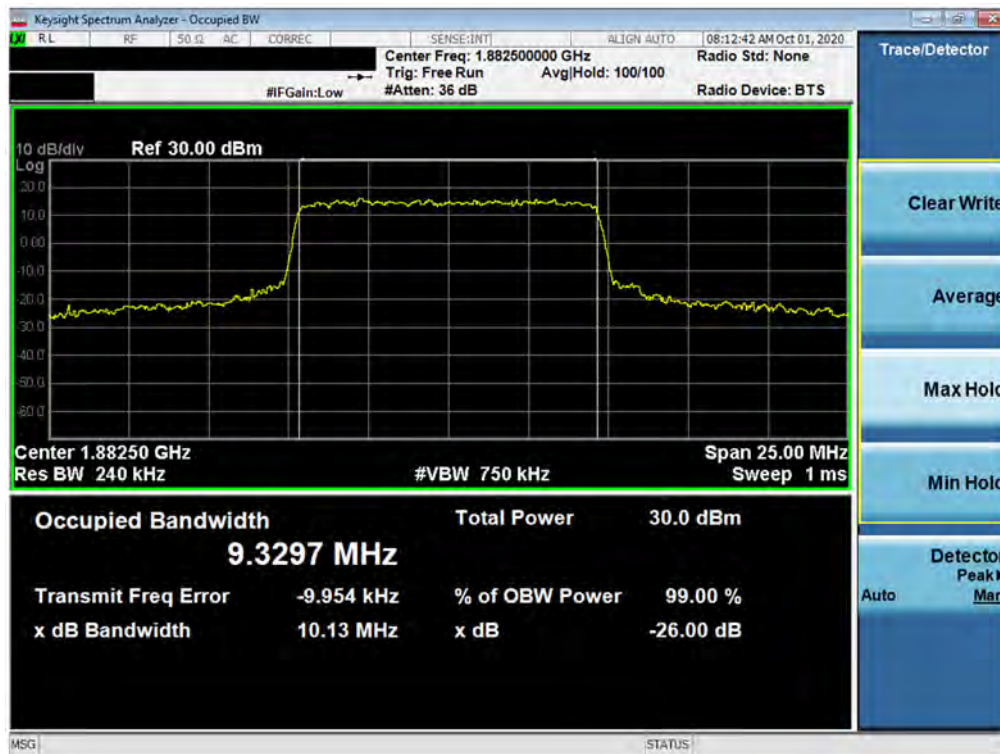
Plot 7-57. Occupied Bandwidth Plot (NR Band n25/2 - 10.0MHz CP-OFDM 64QAM - Full RB)
