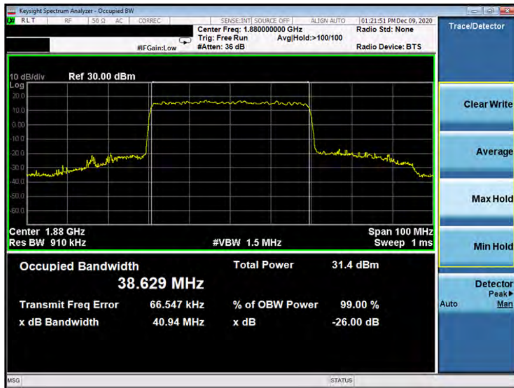
Plot 7-65. Occupied Bandwidth Plot (NR Band n25 - 40.0MHz CP-OFDM QPSK - Full RB)
