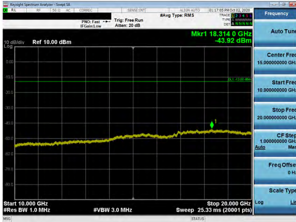
Plot 7-31. Conducted Spurious Plot (CDMA Ch. 1175)
