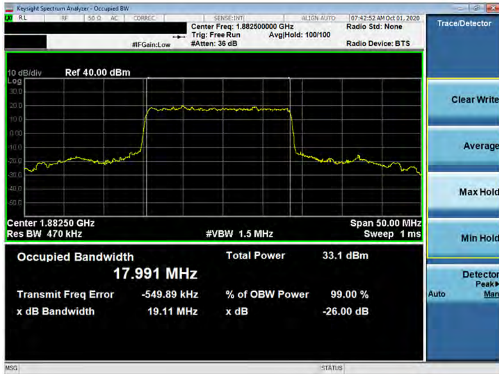
Plot 7-44. Occupied Bandwidth Plot (NR Band n25/2 - 20.0MHz DFT-s-OFDM BPSK - Full RB)
