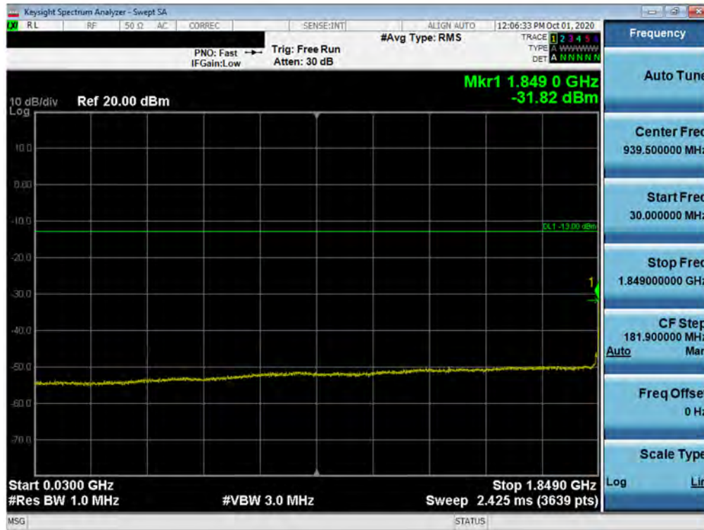
Plot 7-99. Conducted Spurious Plot (LTE Band 25/2 - 20MHz QPSK - RB Size 1, RB Offset 0 - Low Channel)
