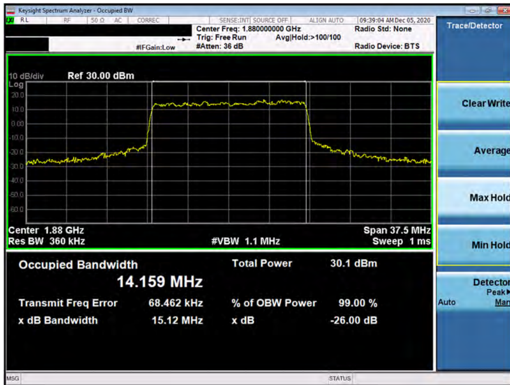
Plot 7-86. Occupied Bandwidth Plot (NR Band n25/2 - 15.0MHz CP-OFDM 16QAM - Full RB)
