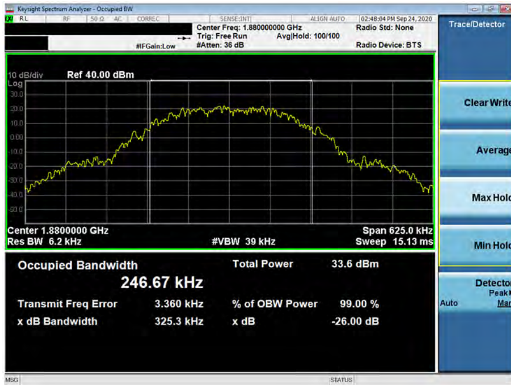
Plot 7-2. Occupied Bandwidth Plot (EDGE, Ch. 661)
