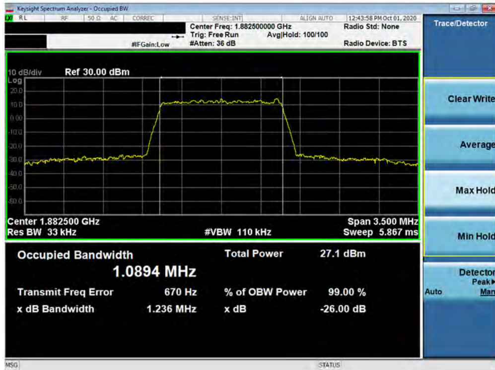
Plot 7-28. Occupied Bandwidth Plot (LTE Band 25/2 - 1.4MHz 256-QAM - Full RB Configuration)
