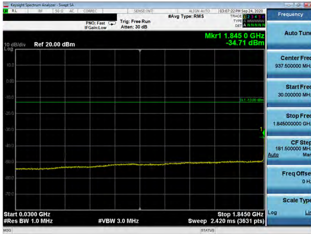
Plot 7-31. Conducted Spurious Plot (WCDMA Ch. 9262)
