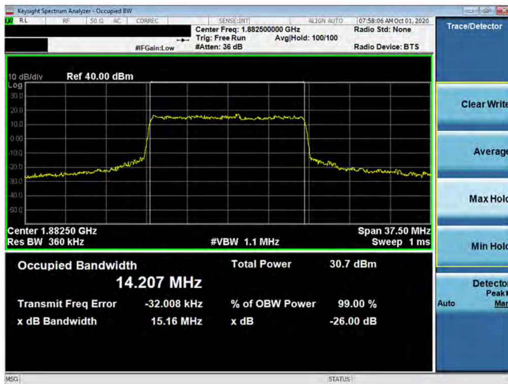
Plot 7-51. Occupied Bandwidth Plot (NR Band n25/2 - 15.0MHz CP-OFDM 16QAM - Full RB)
