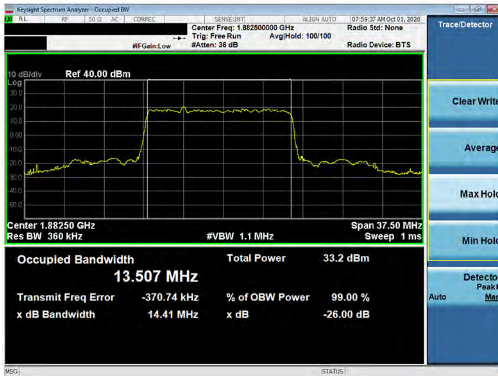
Plot 7-49. Occupied Bandwidth Plot (NR Band n25/2 - 15.0MHz DFT-s-OFDM BPSK - Full RB)
