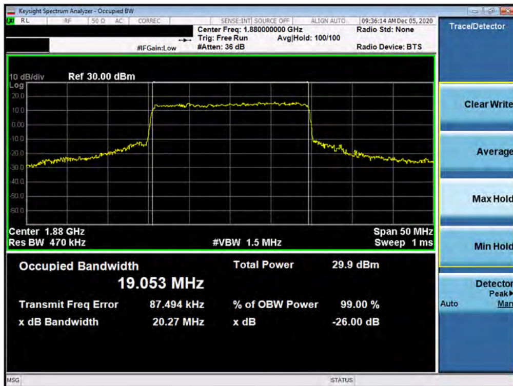
Plot 7-80. Occupied Bandwidth Plot (NR Band n25/2 - 20.0MHz CP-OFDM QPSK - Full RB)
