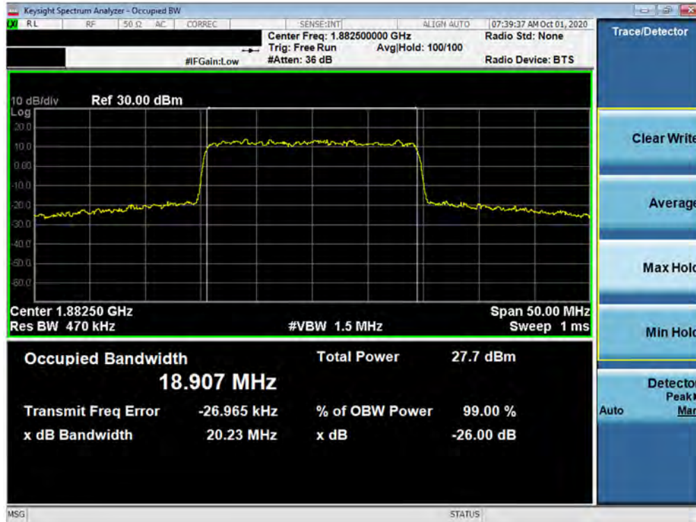
Plot 7-48. Occupied Bandwidth Plot (NR Band n25/2 - 20.0MHz CP-OFDM 256QAM - Full RB)
