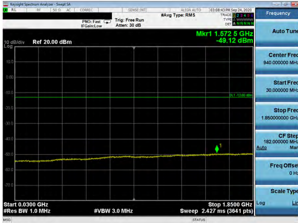
Plot 7-31. Conducted Spurious Plot (WCDMA Ch. 9538)
