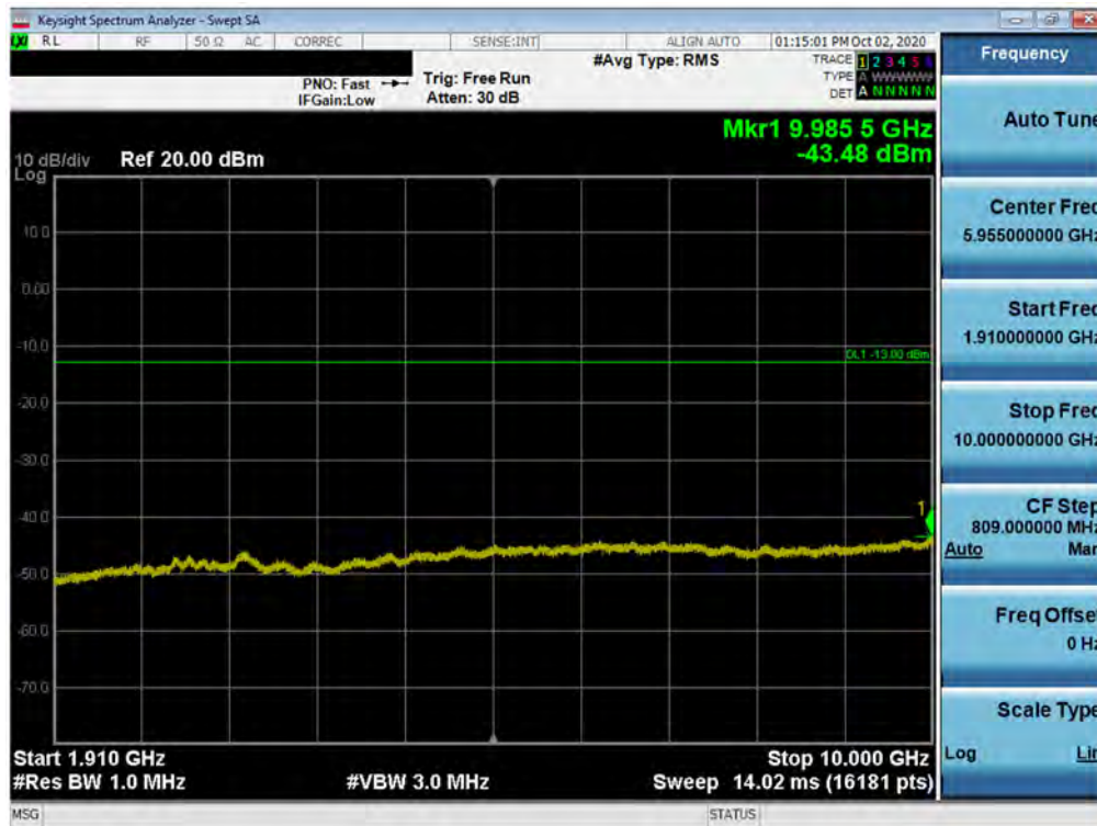
Plot 7-31. Conducted Spurious Plot (CDMA Ch. 25)
