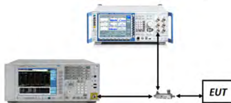
Figure 7-1. Test Instrument & Measurement Setup
