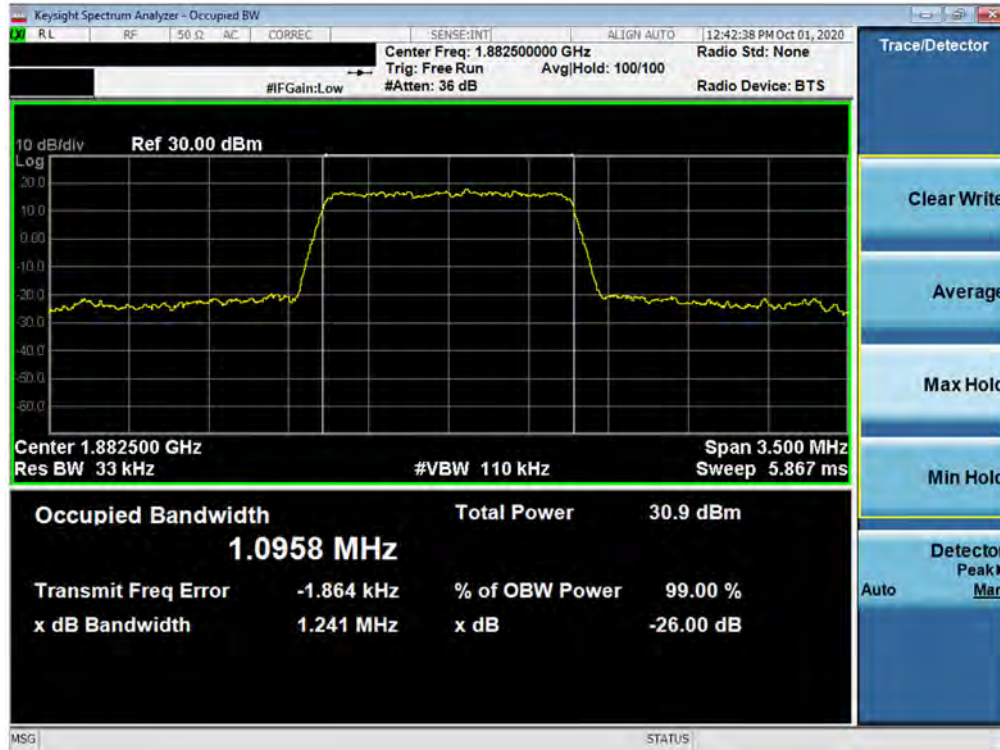
Plot 7-25. Occupied Bandwidth Plot (LTE Band 25/2 - 1.4MHz QPSK - Full RB Configuration)
