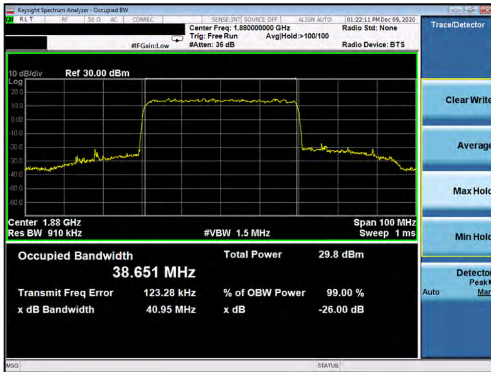
Plot 7-67. Occupied Bandwidth Plot (NR Band n25 - 40.0MHz CP-OFDM 64QAM - Full RB)
