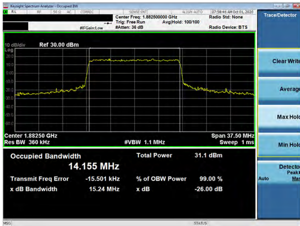
Plot 7-50. Occupied Bandwidth Plot (NR Band n25/2 - 15.0MHz CP-OFDM QPSK - Full RB)
