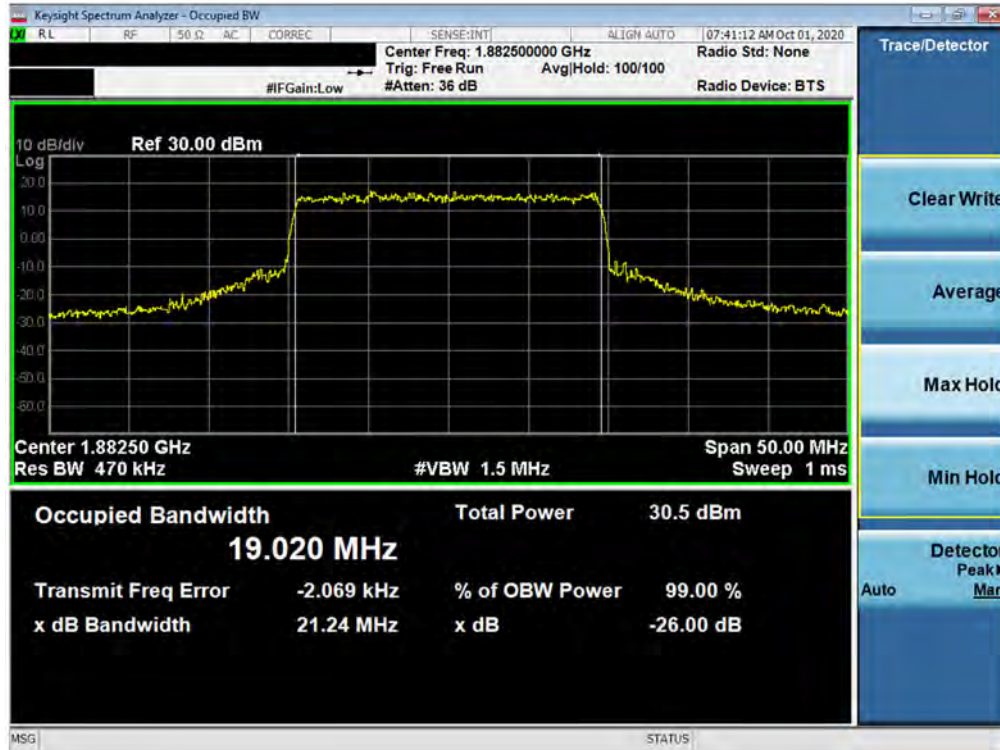
Plot 7-46. Occupied Bandwidth Plot (NR Band n25/2 - 20.0MHz CP-OFDM 16QAM - Full RB)
