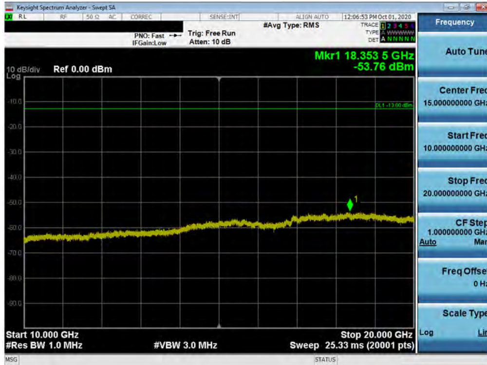
Plot 7-101. Conducted Spurious Plot (LTE Band 25/2 - 20MHz QPSK - RB Size 1, RB Offset 0 - Low Channel)
