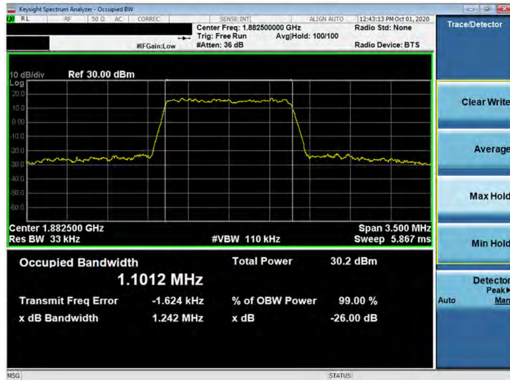
Plot 7-26. Occupied Bandwidth Plot (LTE Band 25/2 - 1.4MHz 16-QAM - Full RB Configuration)
