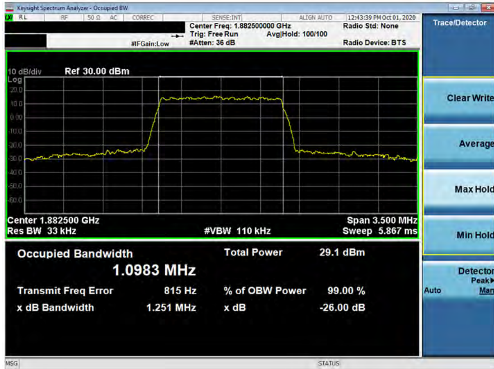
Plot 7-27. Occupied Bandwidth Plot (LTE Band 25/2 - 1.4MHz 64-QAM - Full RB Configuration)
