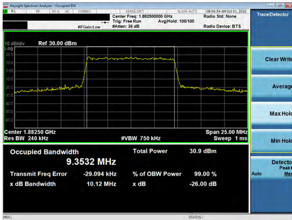
Plot 7-55. Occupied Bandwidth Plot (NR Band n25/2 - 10.0MHz CP-OFDM QPSK - Full RB)
