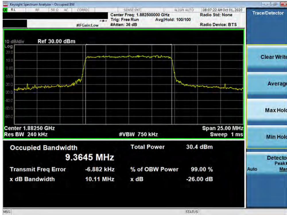
Plot 7-56. Occupied Bandwidth Plot (NR Band n25/2 - 10.0MHz CP-OFDM 16QAM - Full RB)
