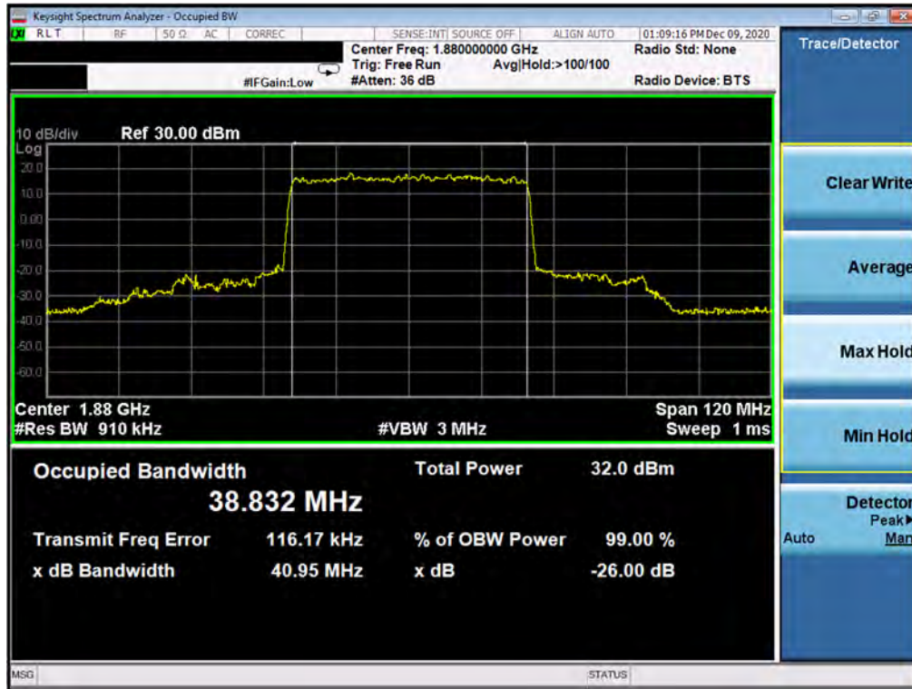
Plot 7-29. Occupied Bandwidth Plot (NR Band n25 - 40.0MHz DFT-s-OFDM BPSK - Full RB)
