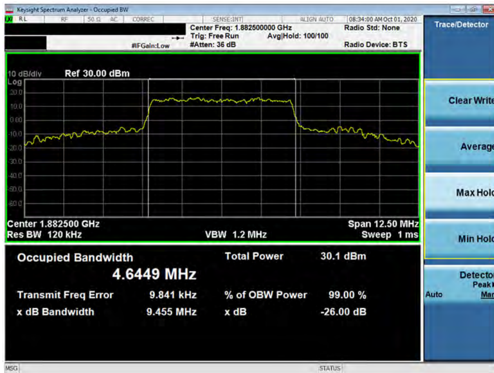
Plot 7-61. Occupied Bandwidth Plot (NR Band n25/2 - 5.0MHz CP-OFDM 16QAM - Full RB)
