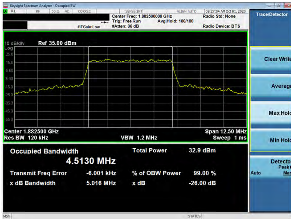
Plot 7-59. Occupied Bandwidth Plot (NR Band n25/2 - 5.0MHz DFT-s-OFDM BPSK - Full RB)
