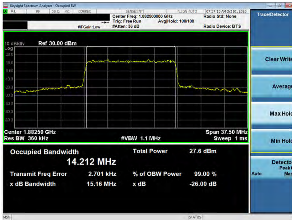
Plot 7-53. Occupied Bandwidth Plot (NR Band n25/2 - 15.0MHz CP-OFDM 256QAM - Full RB)
