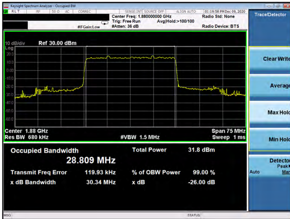
Plot 7-69. Occupied Bandwidth Plot (NR Band n25 - 30.0MHz DFT-s-OFDM BPSK - Full RB)
