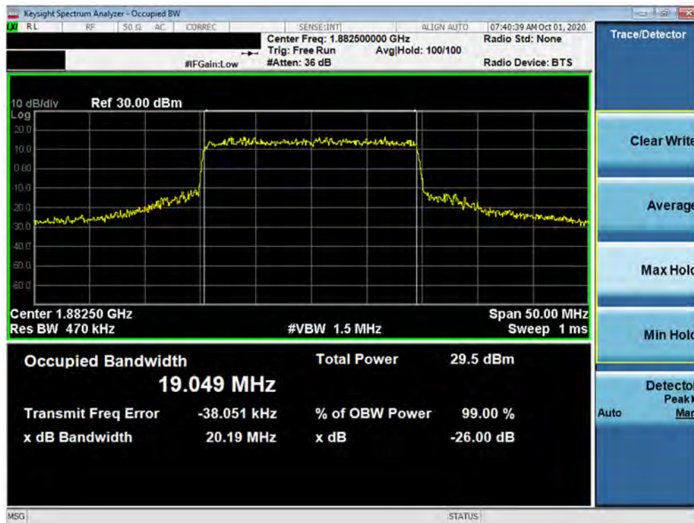
Plot 7-47. Occupied Bandwidth Plot (NR Band n25/2 - 20.0MHz CP-OFDM 64QAM - Full RB)
