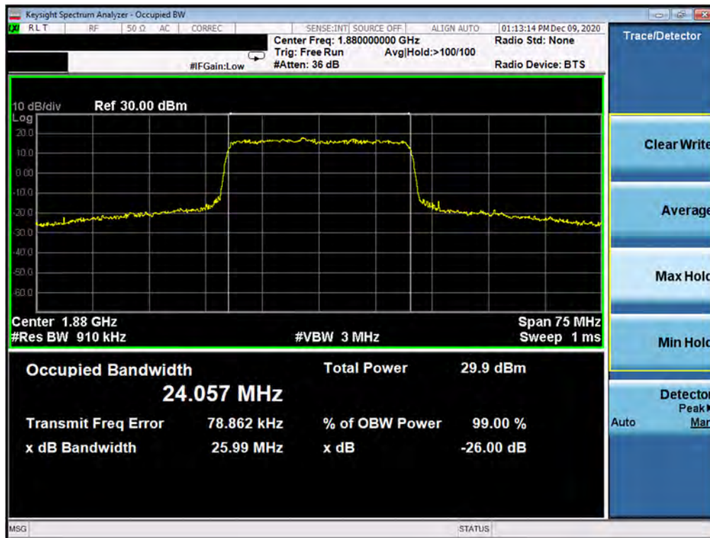
Plot 7-40. Occupied Bandwidth Plot (NR Band n25 - 25.0MHz CP-OFDM QPSK - Full RB)
