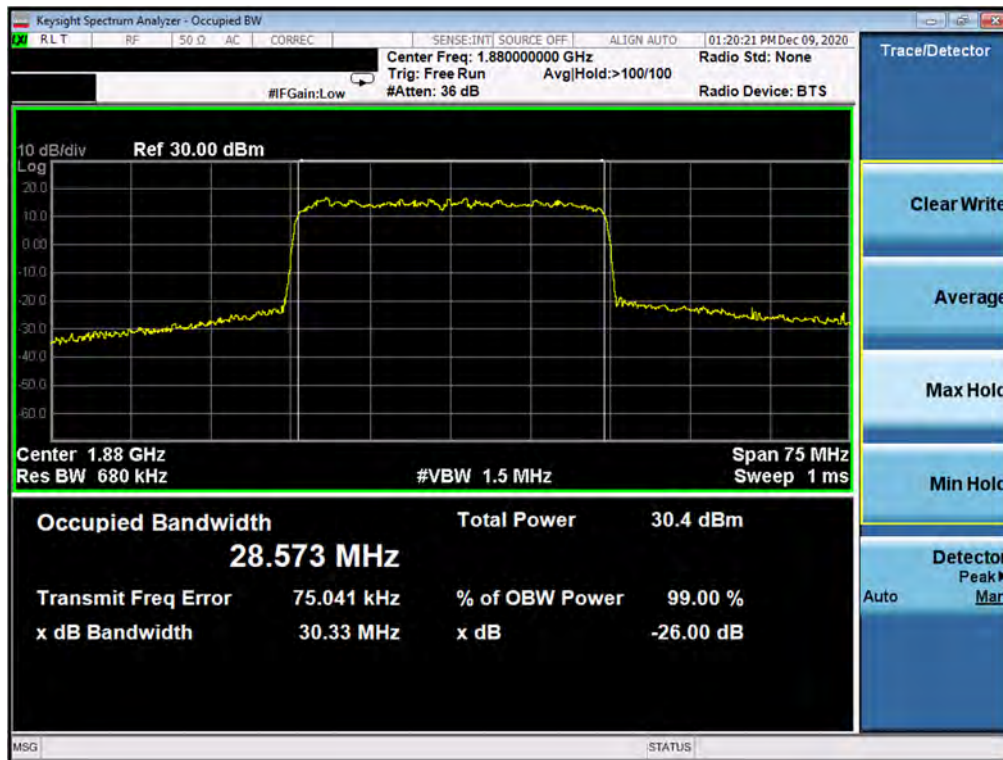
Plot 7-71. Occupied Bandwidth Plot (NR Band n25 - 30.0MHz CP-OFDM 16QAM - Full RB)
