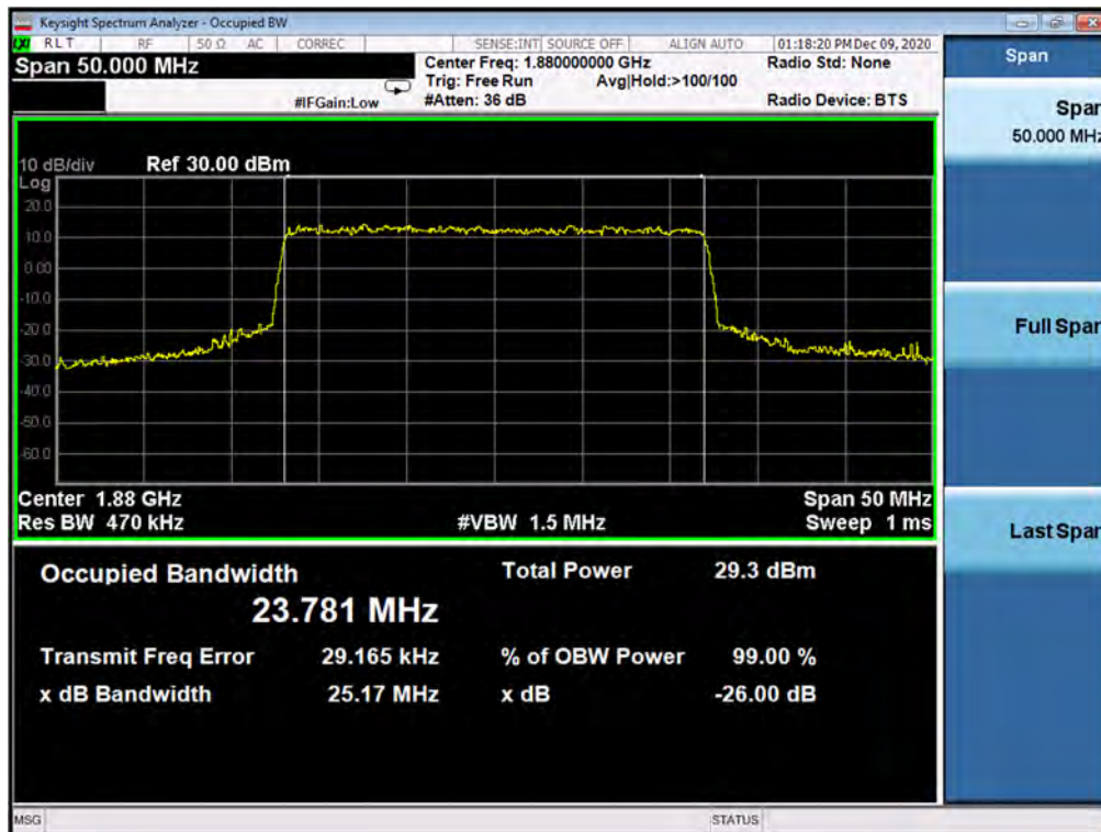
Plot 7-75. Occupied Bandwidth Plot (NR Band n25 - 25.0MHz CP-OFDM QPSK - Full RB)
