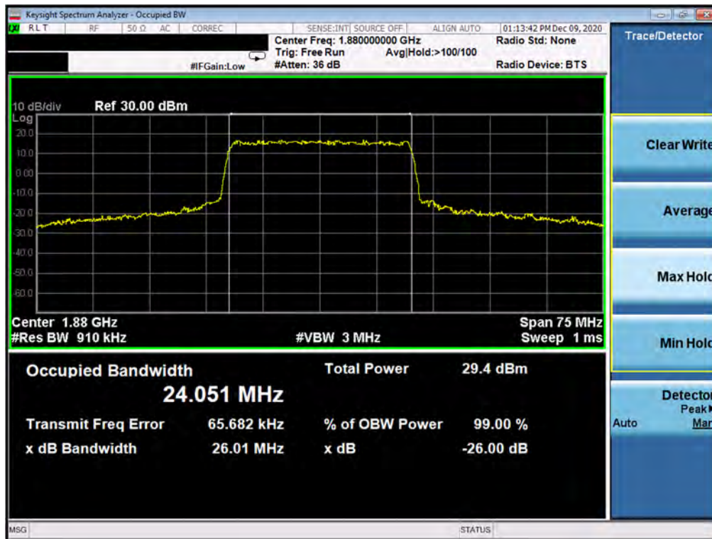
Plot 7-42. Occupied Bandwidth Plot (NR Band n25 - 25.0MHz CP-OFDM 64QAM - Full RB)
