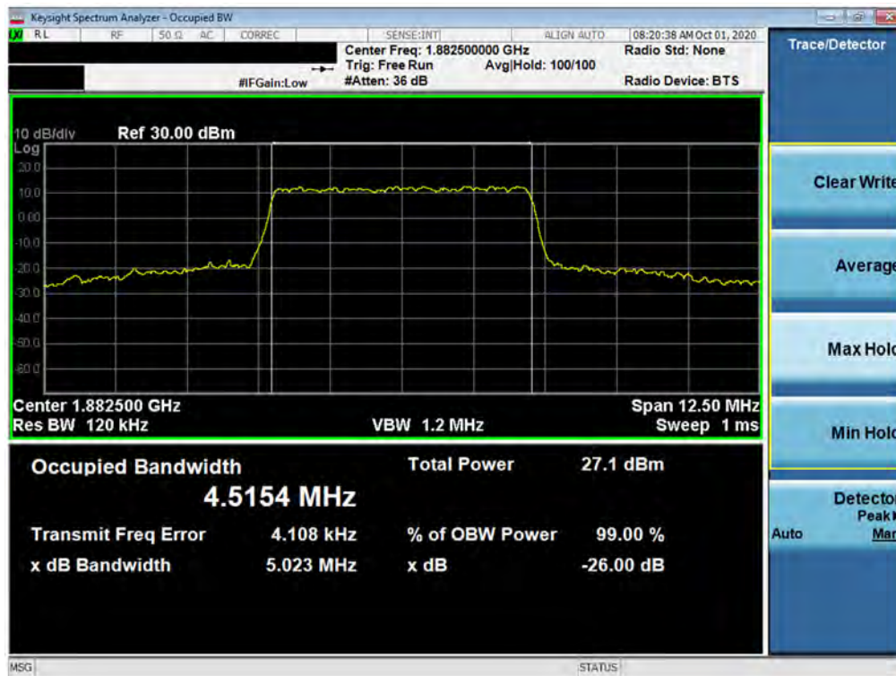
Plot 7-63. Occupied Bandwidth Plot (NR Band n25/2 - 5.0MHz CP-OFDM 256QAM - Full RB)
