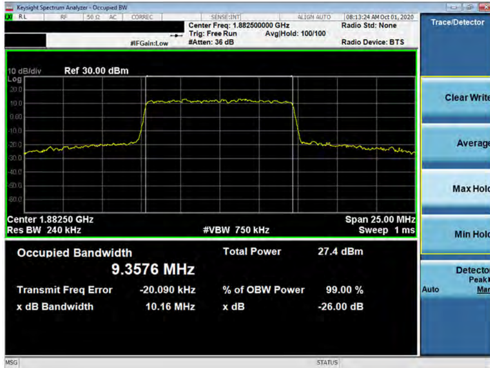
Plot 7-58. Occupied Bandwidth Plot (NR Band n25/2 - 10.0MHz CP-OFDM 256QAM - Full RB)
