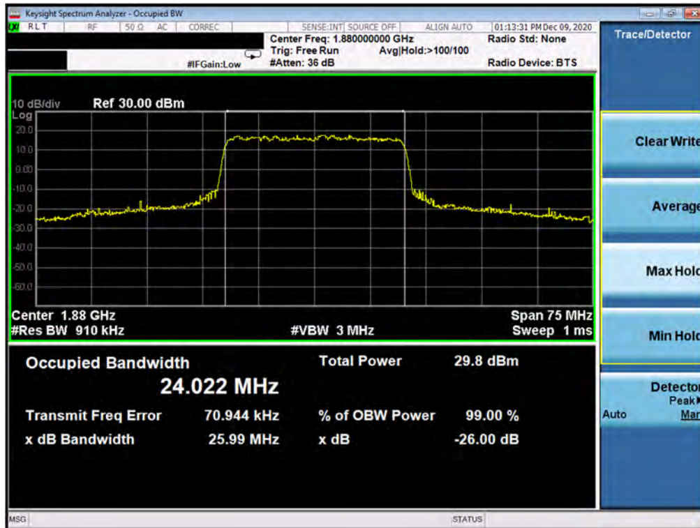
Plot 7-41. Occupied Bandwidth Plot (NR Band n25 - 25.0MHz CP-OFDM 16QAM - Full RB)
