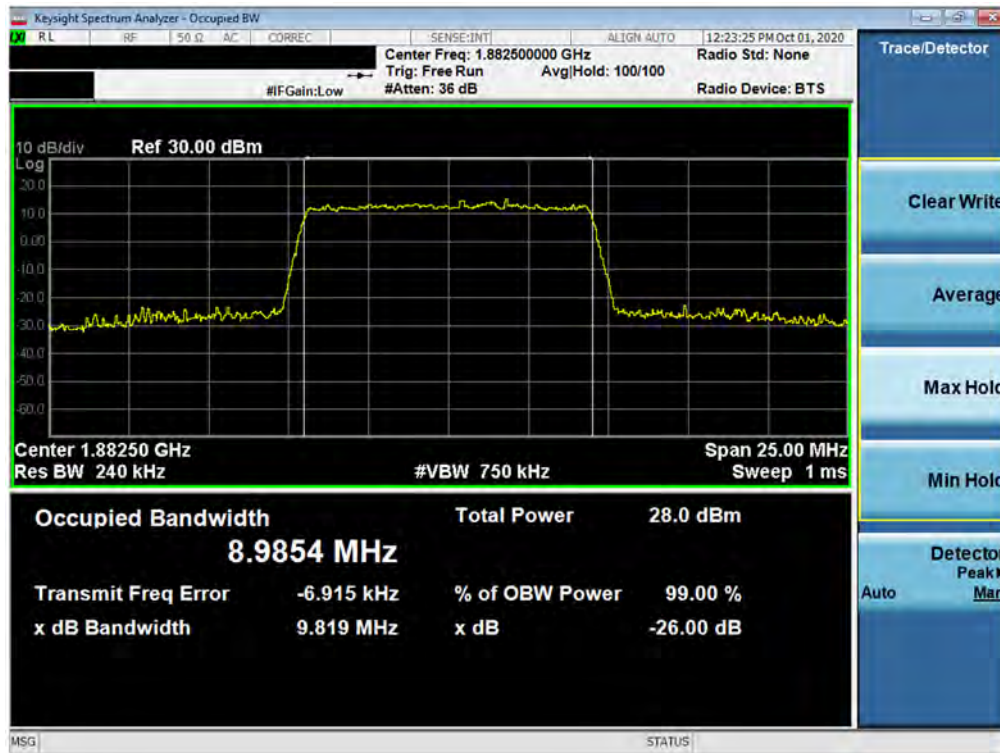
Plot 7-16. Occupied Bandwidth Plot (LTE Band 25/2 - 10MHz 256-QAM - Full RB Configuration)
