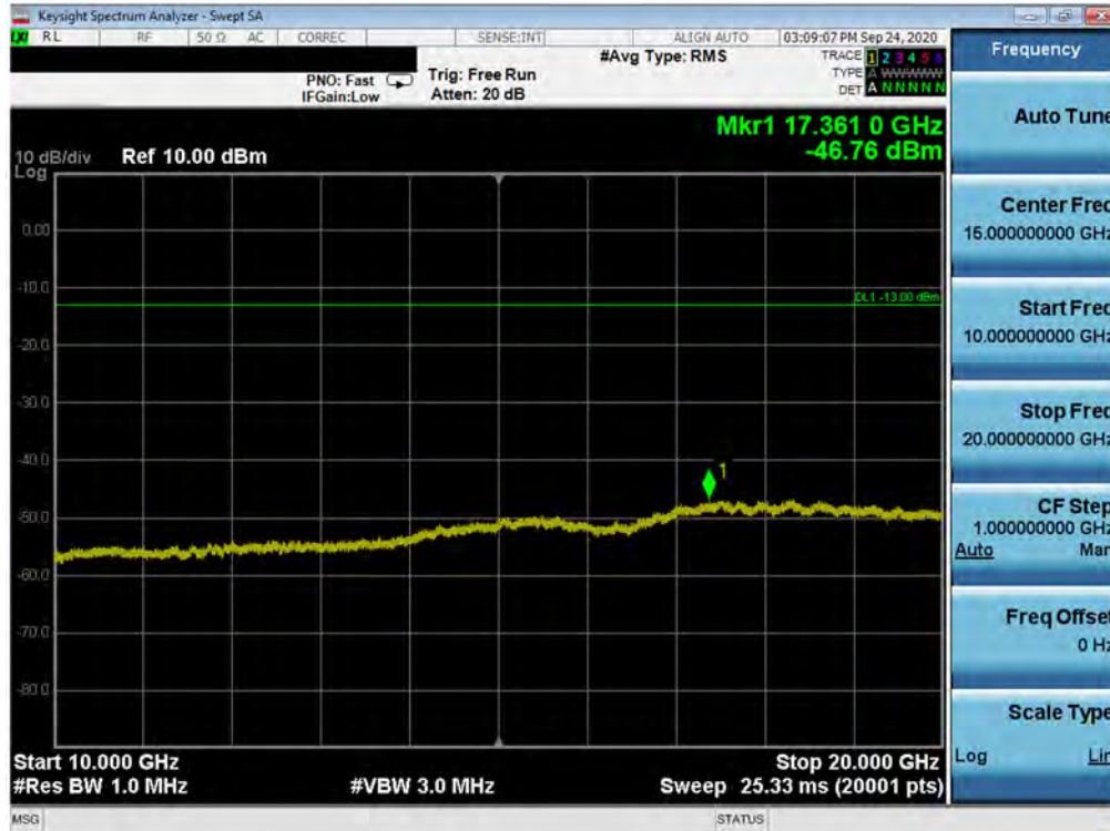
Plot 7-31. Conducted Spurious Plot (WCDMA Ch. 9538)
