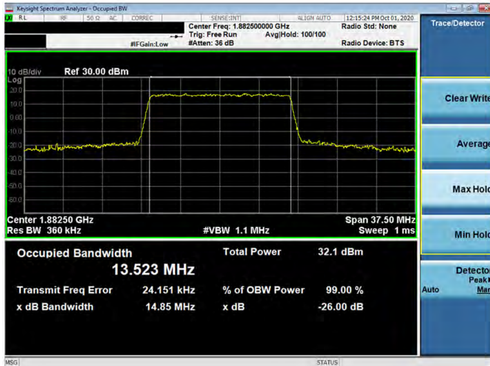
Plot 7-9. Occupied Bandwidth Plot (LTE Band 25/2 - 15MHz QPSK - Full RB Configuration)
